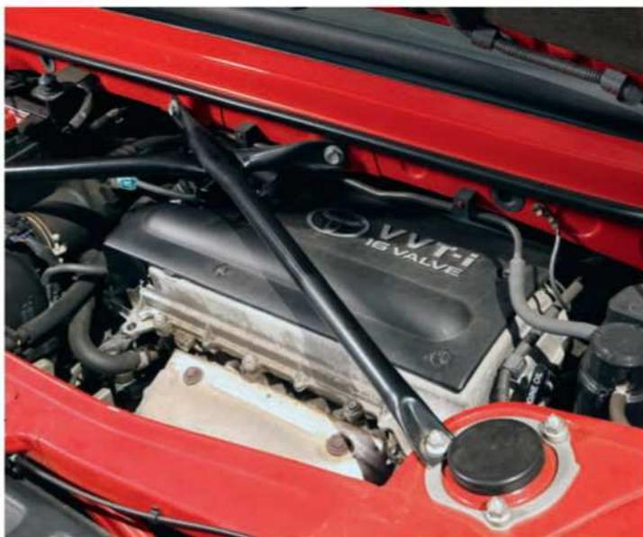
The VVT 16-valve twin-cam **engine** is a classic modern all-aluminium unit: revvy, powerful and remarkably durable if well maintained (many have reached 150k+ miles without problems). Look for a full service history, no warning lights or fault codes, and ideally evidence that pre-cat issues have been addressed
