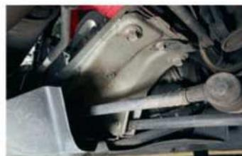
Check the rear **subframe** that carries the engine and suspension, because it rots. If in doubt, remove the undertray that hides it on all but the final cars
