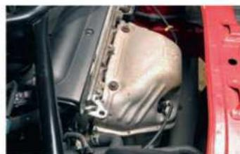
The pre-cat, linked to the EGR system in the **exhaust manifold**, can cause major engine damage when it breaks down: it's best replaced or removed
