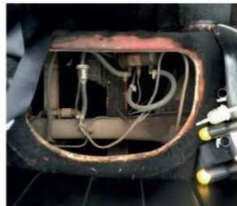
Back seats out to adjust the handbrake
