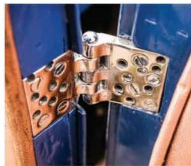
Clockwise from main: Type 57S's lines were crafted by English coachbuilder Corsica; unblown 3.2-litre straight-eight has punchy performance; snug cabin, low seat; holes drilled in 57.375's door hinges, in pursuit of lightness
