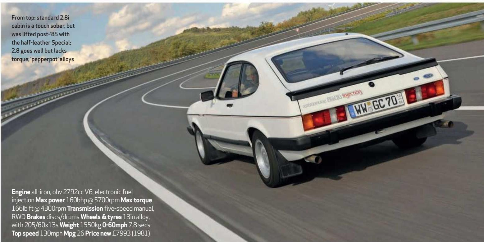
**Engine** all-iron, ohv 2792cc V6, electronic fuel injection **Max power** 160bhp @ 5700rpm **Max torque** 166lb ft @ 4300rpm **Transmission** five-speed manual, RWD **Brakes** discs/drums **Wheels & tyres** 13in alloy, with 205/60x13s **Weight** 1550kg **0-60mph** 7.8 secs **Top speed** 130mph **Mpg** 26 **Price new** £7993 (1981)
