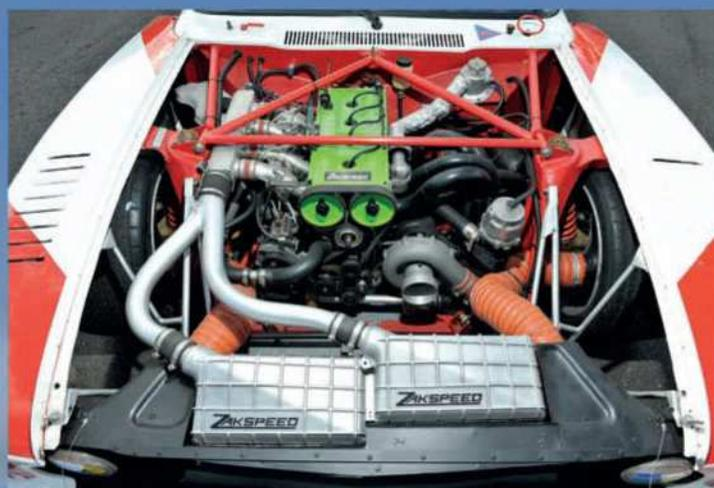
**Engine** all-alloy, dohc 1745cc 'four', Bosch electronic fuel injection and twin KKK turbochargers **Max power** 600bhp @ 9000rpm
