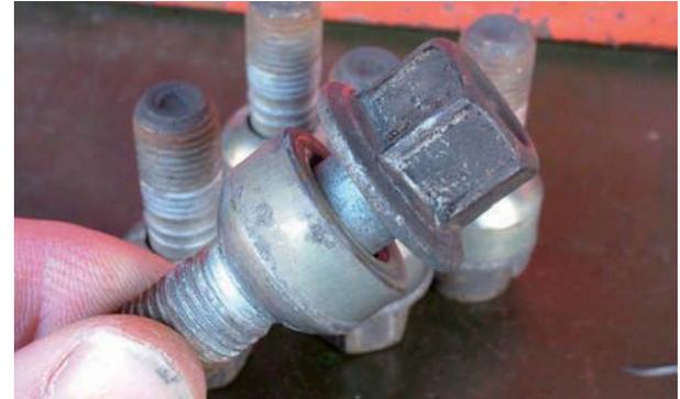
To grease or not to grease? That is, indeed, the question. On the threaded area, certainly (but sparingly), and between top of collar and underside of bolt head. But NOT on conical face of collar
