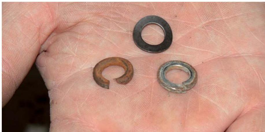
Spring washer on the far right looks OK, doesn't it? Maybe so, but chances are it could eventually break up like the one on the left, leaving the nut and/or bolt it is meant to be securing free to work loose. Best answer – where locking compound is neither specified nor appropriate – is a wave washer (top)
