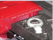
2008 Cayenne's VIN - stamped into cargo-space floorpan - shows type number, like that of first-generation cars, to be 9PA; VIL (left) shows additional AL1 code
