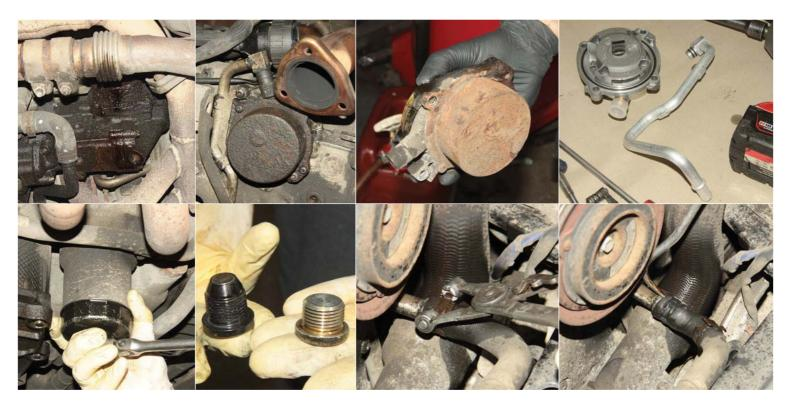
Access to pump necessarily limited; second pic from top left shows its location on another engine removed from car. Surface rust quickly develops into tiny holes. New pump costs £318 plus VAT. Job requires draining engine oil, so a good opportunity to change it, together with filter; install magnetic sump plugs, too. Remove air-filter housing for access to top end of metal pipe
