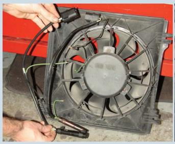
Resistor pack, as it is known, comes complete with wiring and integral connection, plus new clips - as you might hope for £70-plus a time
