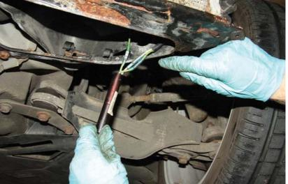
Removing the entire radiator fan to make the necessary connections is such a palaver, however, that most specialists simply cut and splice into the wiring here
