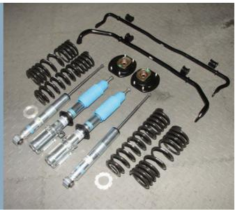
he story so far: two months ago, in the August edition of the magazine, we left Chris Howell's 964 Targa on the combined lift and geo rig at Center Gravity in Warwickshire, in the early stages of what would prove to be more or less a full suspension overhaul, using brand-new Bilstein dampers, Eibach Pro-Kit springs, and anti-roll bars from the latter
