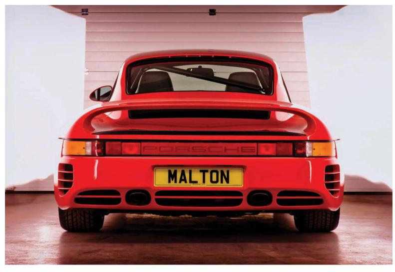
Engine is a 2.8-litre, twin turbo, with water-cooled heads, putting out 450hp. As you can see, this is one of the ultra rare Sport models, with cloth trim and roll cage etc. Hollow spoke, magnesium wheels, featured tyre pressure monitors
