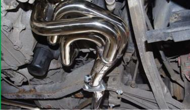
A pipe bending work of art. Shame the new manifolds are hidden under the car
