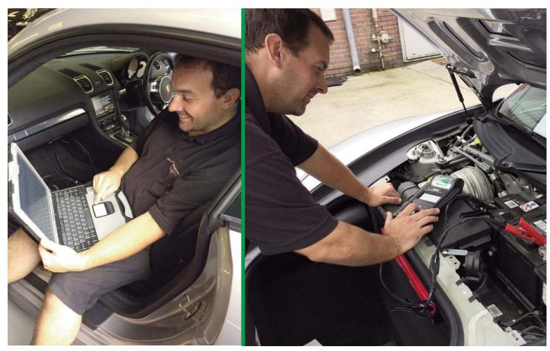
Mark always smiles when he's working! Checking the fault codes led to a check on the alternator output and battery condition
