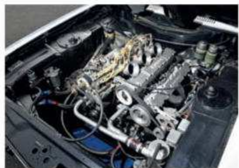
Cologne engine was based on 3-litre block
