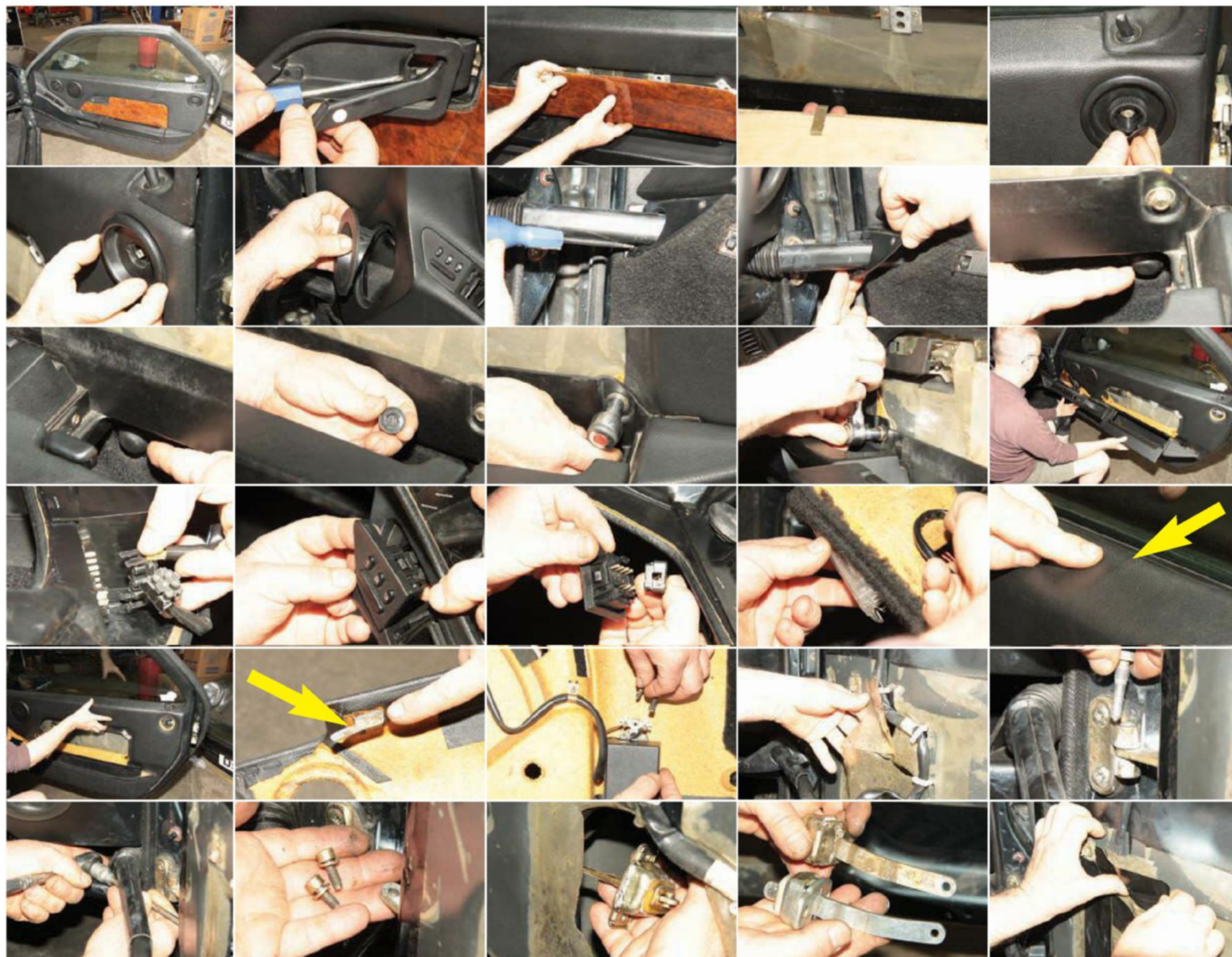
Wooden trim panel has press fixings along its top edge, metal tabs along the lower; carefully prise off accordingly. Plastic recess for door-locking knob (second row, far left) unscrews in usual anti-clockwise direction. Disconnect all wiring after armrest has been removed – and only then attempt to separate bottom part of door card from shell. Most important point is arrowed tab (above), which requires that card be pulled forward slightly before you try to lift it. Ignore that, and you'll leave a tell-tale crease (above)
