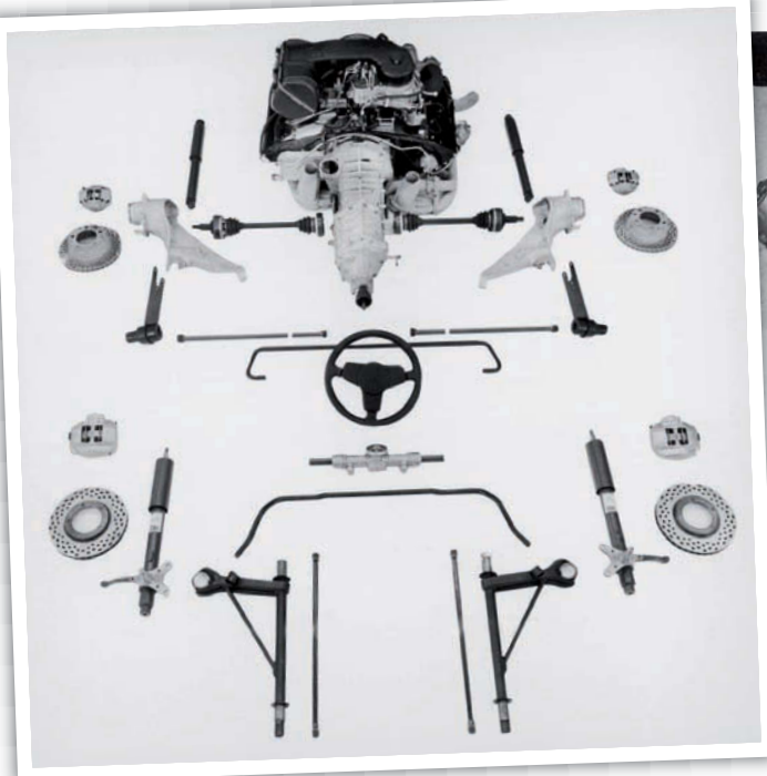
The nuts and bolts of the 911 Turbo: exhaust, turbo, uprated brakes and suspension components were laid out for all to see by the press department. First Turbos, though, relied on stock 911S braking...
