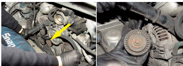
Auxiliary drive-belt (for the generator, plus the coolant, steering and air-con pumps) is tensioned by a spring-loaded roller (arrowed). Release that with a suitable spanner, and belt slips off easily. Latter can be used again if in good enough condition (in which case make sure it goes back on in the same orientation as before), but no harm in fitting a new one, while you have the opportunity. Likewise this idler roller (right), which has to come off anyway, for access to one of the alternator's fixing screws
