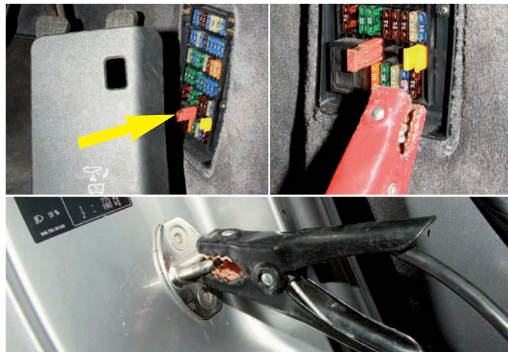
These photos show the fuse board and emergency battery connection in a 996, but 997 is pretty much identical. Use this for opening the front lid only, NOT as a way of jump-starting - see above
