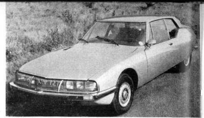
ADVANCED.-The Citroen SM with FWD, hydropneumatic suspension, variable power steering, inboard front brakes, V6 Maserati engine, and 5-speed gearbox. Of the six headlamps the inner pair turn with the steering, and the perspex cover over the lamps and number-plate presents an unbroken nose-line to the wind.
