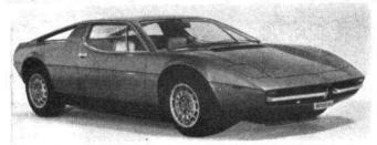
NEW BOLOGNA TRIDENT .- The Maserati "Merak" with centrally mounted 3-litre V6 engine and Citroën 5-speed gearbox driving the rear wheels. The body design is by Giorgio Gingiaro and his ITAL DESIGN
