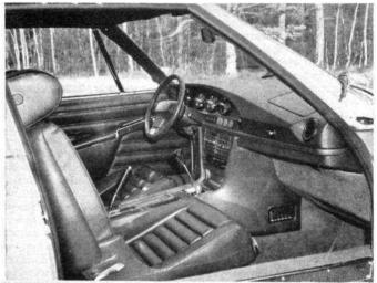
INTERIOR VIEW.—The driving compartment of the Citroen SM is spacious and comfortable with a rigid central gear-lever positioned for use. The oval steering wheel and column surround adjusts up and down or in and out, as a complete unit. The "glove locker" on the scuttle is nothing more than that. Warm air is deflected onto the feet from the central grille.
