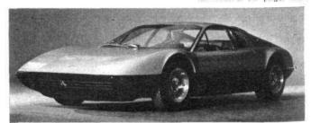
NEW: PRANCING HORSE.—The Ferrari Berlinetta-Boxer, with its 4.4-litre flat-12-cylinder engine mounted amidships. It runs on Michelin 215/70 VR 15X tyres and 187 m.p.h. is claimed as top speed.
