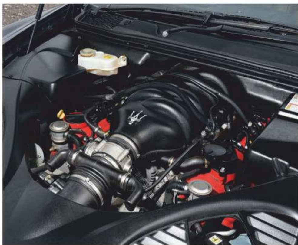
There's little to choose between the 4.2- and 4.7-litre engines ; both are superb. All have red cam covers except 4.2 ZF-gearbox cars, which had blue. DuoSelect cars had dry-sump engines, ZF cars had a wet sump. Listen for rattly timing variators (on start-up and overrun), and look for oil and water leaks
