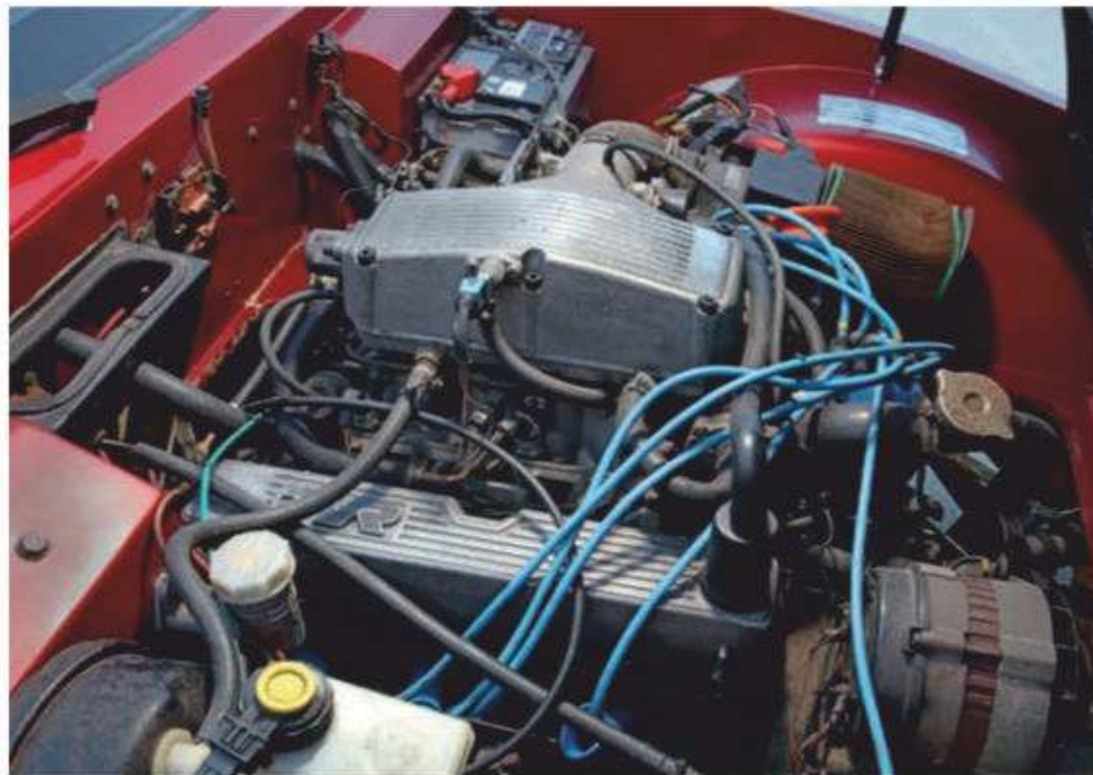
Above: wedge at rest on Rosslare beach – bright-red additions lift the angular interior, but the glovebox lid was originally veneered. Right: the Buick-derived, all-aluminium Rover V8 makes 197bhp in 3.5-litre form for the 350i
