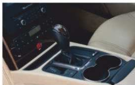
Here is ZF's auto gearbox with the paddleshift option. Early cars had the DuoSelect transaxle, an automated manual – only for enthusiasts
