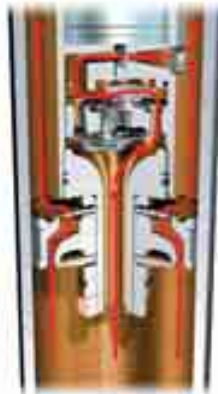
Compression in 'Normal' mode – bypass valve open
