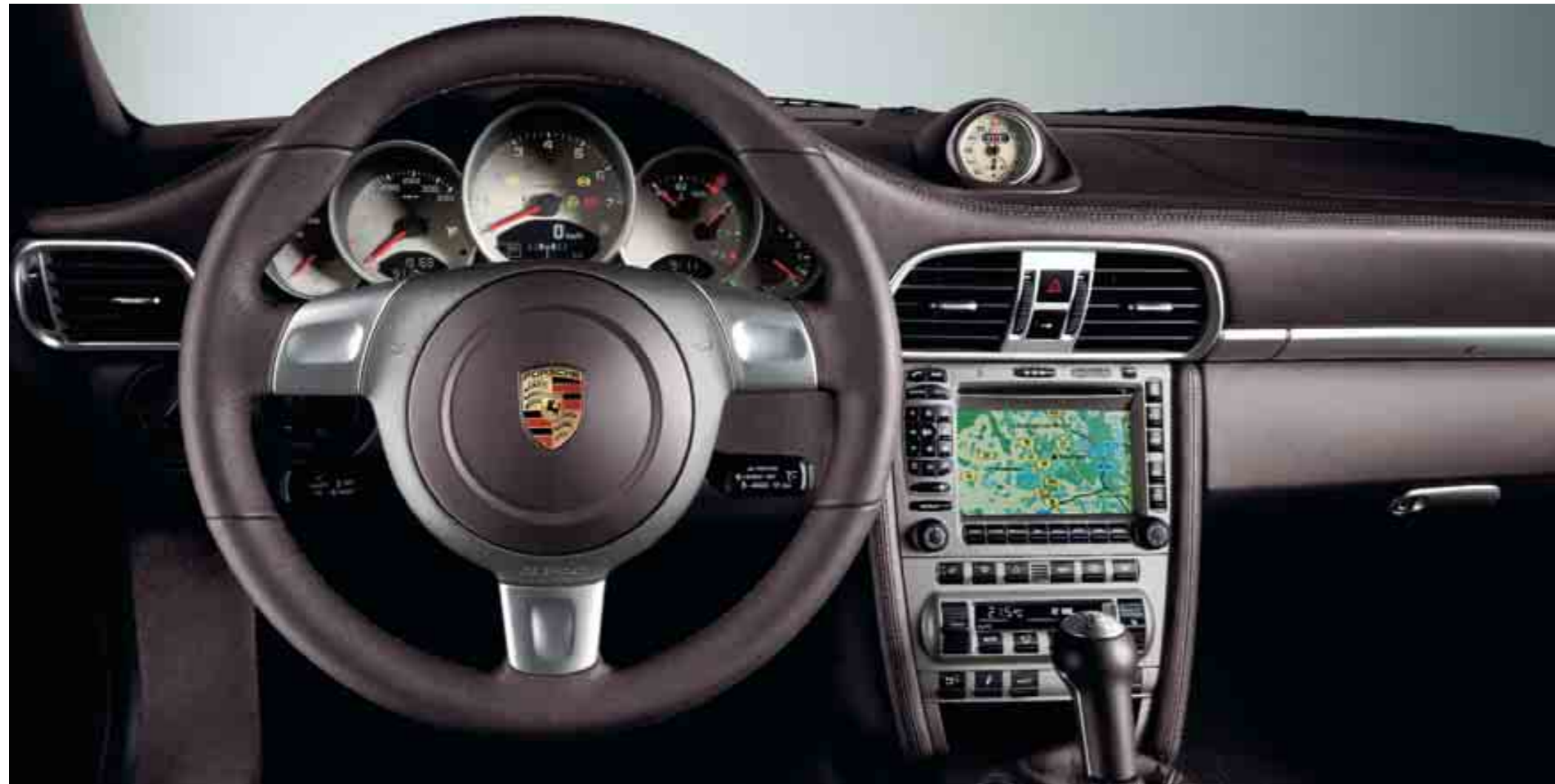
Dashboard (911 Carrera S/911 Targa 4S) with various options, including leather interior, Sport Chrono Package Plus, cruise control, navigation module and Tyre Pressure Monitoring (TPM)
