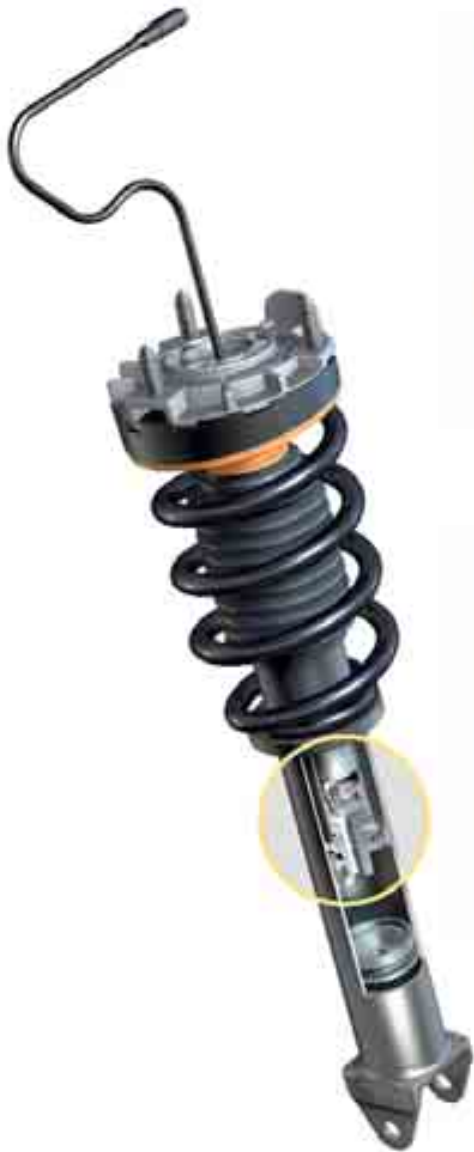
Rebound in 'Normal' mode – bypass valve open
