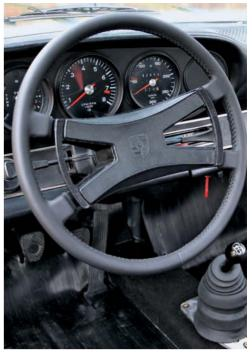
Interior looks remarkably standard, right down to the steering wheel. Simple door pulls and Scheel seats hint at Sport ('lightweight') M471 specification
