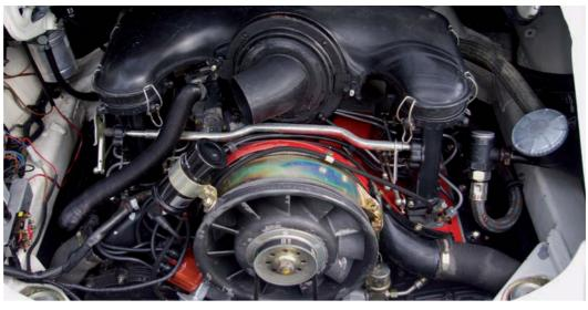
2993cc engine featured a bore and stroke of 95mm x 70.4mm, and produced 23obhp at 62oorpm. Aluminium crankcase was used in preference to lighter magnesium for strength
