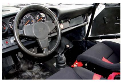
Recaro seats have been upgraded to meet current FIA regulations. Full-on RSR version came with 10,000rpm tach, but roadgoing RS featured regular 8000rpm instrument
