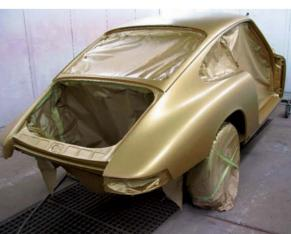
Seeing the car fully masked up, in primer and rubbed down ready for paint was a major boost. When the gold basecoat was first applied, it looked dull, with an almost green-ish tint. But that would soon change...
