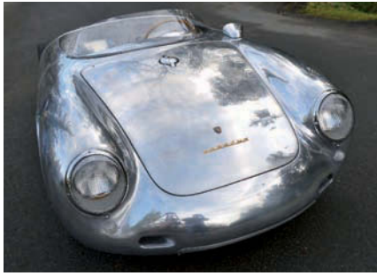
Finished bodywork is flawless. Simple roll-over hoop is removable, along with its brace, to allow removal of rear bodywork. Photo on far right emphasises how small the 500A Spyder is in real life!
