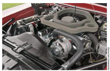
Unlike the R/A-IV engine, the R/A-III engine could be ordered with air conditioning. This example also features optional cruise control. The 400-H.O. option, available in the Firebird 400, was a functionally identical engine sans the Ram Air system.
