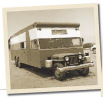
dead axles—perhaps the same ones that originally underpinned the travel trailer—and that the builder used the Jeep because its transfer case allowed it to run off the front wheels alone.
