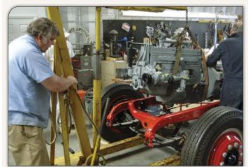
The Hercules engine is being lowered into position. This massive six-cylinder was rated for only 143 hp; however, it was selected by the factory not for speed, but rather its torque—a whopping 488 lb.ft.—to drive the water pump with ease.
