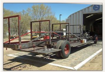
With exception of the suspension systems and the ladder bed framing welded into position at the Seagrave assembly plant, everything has been removed from the chassis, most of which has been painstakingly stripped to bare steel.
