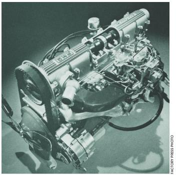
Pontiac's Sprint package for the OHC-6 from 1967 through 1969 had a four-barrel and a hotter camshaft, as this pre-1969 press photo reveals.
