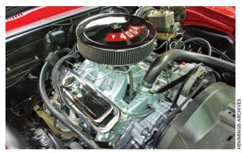
Maintaining a somewhat stock appearance, our feature car's 400 engine has been modified for more power. Note the painted Edelbrock intake, open air cleaner and long-branch exhaust.
