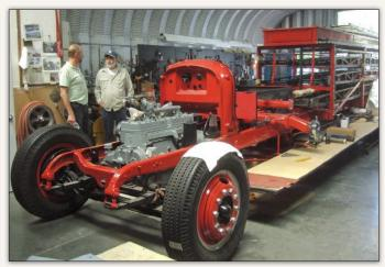
The engine, cowl—now outfitted with its refurbished factory gauges—and water pump have been installed. At the opposite end, the full complement of restored ladders has been carefully loaded into the associated steel framing; running boards are next.
