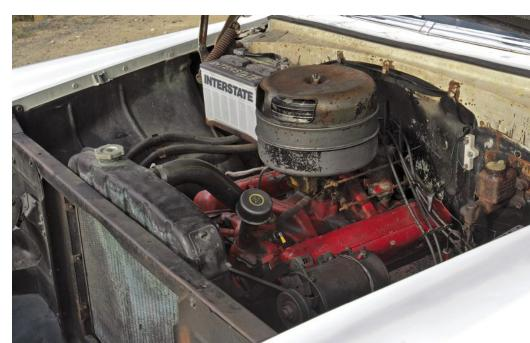
The quiet and competent 265-cu.in. small-block Chevrolet V-8 still runs well with the original oil-bath air filter and two-barrel carburetor. The Harrison radiator is also original.
