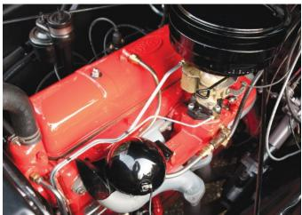
Shortly after the truck was purchased, the 1956-vintage 270 sixcylinder was rebuilt and the engine bay detailed. A 302 GMC six is currently being rebuilt for it.
