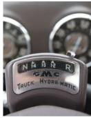
It's strange to see a 1947-'54 GM pickup without a clutch pedal and with the Hydra-Matic range indicator on the column, but **GMC** first installed the automatic in light trucks in 1953. The driver had three ranges to choose from, plus reverse and neutral.
