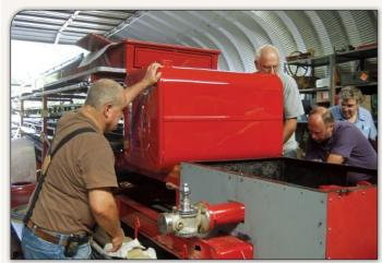
A new water tank is being positioned on the chassis. With the original heavily damaged, a replacement was fabricated from a fuel tank obtained from a tractor-trailer. Also note the newly minted water pump casing that has yet to receive paint.
