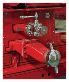
functional. It was no short feat, because we also had to fabricate a driveshaft. There's a short shaft that comes from the transmission to the pump, and then a second shaft from the pump to the differential—the driveline goes through the pump. A fire truck is basically a pump on wheels, and that's why this had a 529-cu. in. engine in it; not for horsepower, but for torque to drive the pump."
