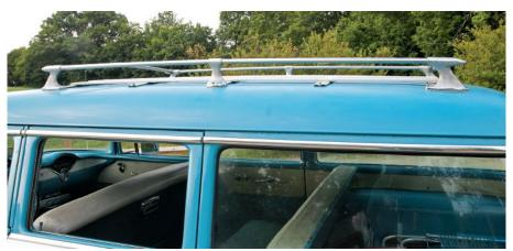
The roof rack chrome finish is worn from use and the elements, but the aluminum and steel structure is still strong enough for luggage or surfboards: the perfect touch for a wagon.
