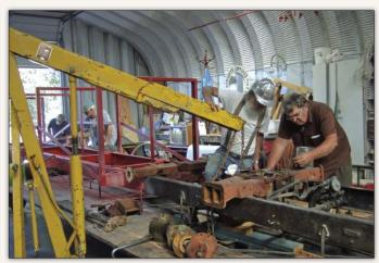
With the front of the chassis stripped of factory paint, club members carefully positioned a new period-correct water pump's mounting points on the frame. This hefty fabrication work done now eliminates the threat of damaging the restoration later.
