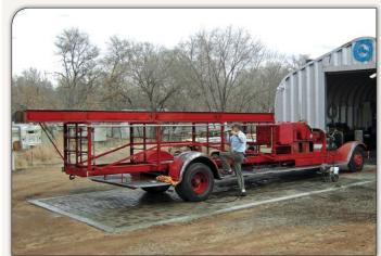
With the truck outside of the clubhouse building, members have already begun the disassembly process by removing hoses, wooden ladders and miscellaneous parts. A thorough power wash removed grime to help expedite the next restoration phase.
