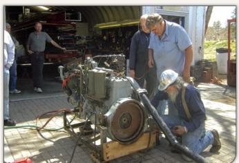
Earlier, a rebuilt military-surplus 529-cu.in. Hercules straightsix had been obtained from a vendor in Ohio. Once delivered to Prescott, Arizona, club members gave it a thorough inspection and test run in preparation for its later installation.
