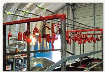
Although the chassis still required some preliminary work, the ladder bed framing became a handy makeshift spray booth for small bolt-on components, which were then left in place to cure before being placed into temporary storage until needed.
