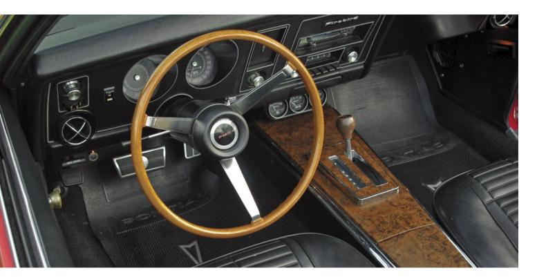
Geno's standard Firebird interior has an optional console and steering wheel (gauges are aftermarket).
