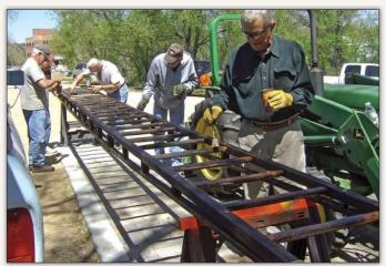
Restoring the Seagrave's factory wooden ladders was just as important. The process started with a chemical stripper, which was later followed by extensive, labor-intensive sanding and several coats of black varnish.
