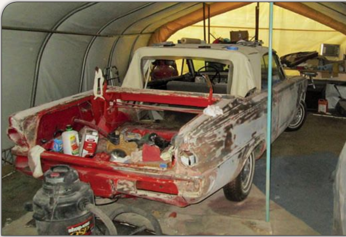
Protected by a temporary structure from the Southern California elements, the convertible was first relieved of its trim and removable panels, save for the doors. The paint was then removed via chemical stripper and sanding.
