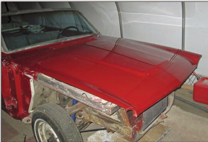
Back inside the temporary structure, the body panels were slowly returned to the Dart chassis. This replacement hood from a parts car sedan was painstakingly aligned to avoid damage later. Fenders and decklid would soon follow.
