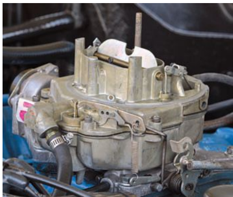
The 390-cu.in. V-8 was returned to stock appearance with the proper factory air cleaner and original Autolite 4300 four-barrel carburetor. A Pertronix electronic ignition hides under the distributor cap.
