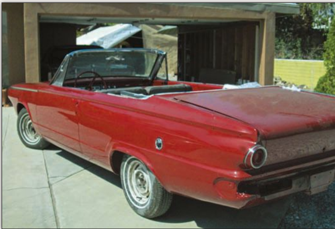
Pulled from hiding, a few pieces of trim have already been returned to the Dart's body. If it looks as though the trunk lid is ajar, that's because it is about to be bolted back into position and realigned with the rest of the rear panels.
