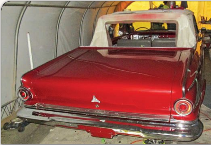
Bit by bit, trim was slowly returned to the back half of the Dart, while making sure the wiring remained functional. Overspray on the convertible top was not a concern, as a new one was going to be installed in due time.
