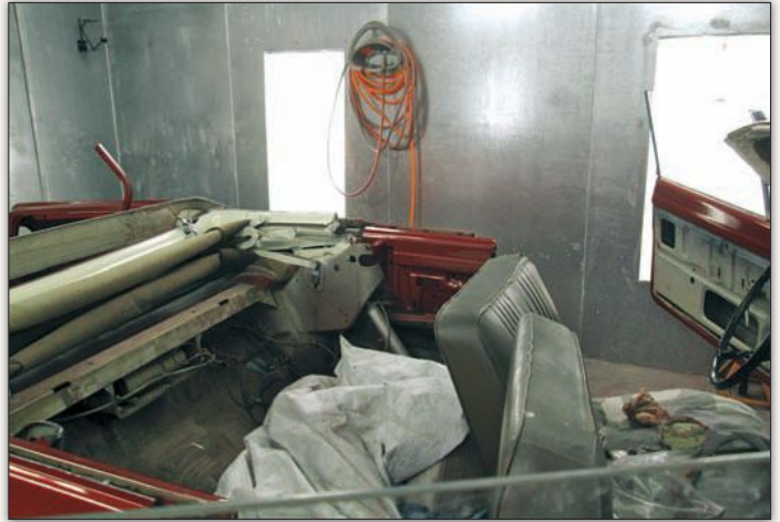
During most restorations, the interior is removed prior to paint. In this case, as the car remained functional, the original shoddy interior and top, sans rear bench seat, were left in place to assist in the car's movement from one location to another.
