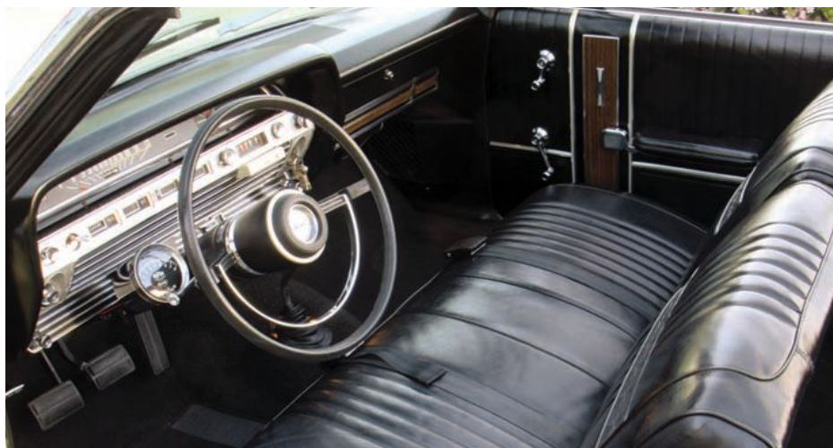
A dealer accessory tachometer sits to the left of the new-for-1967 energy-absorbing steering wheel. The vast expanse of bench seat makes for easy views of the sweeper speedometer. The AM radio with 8-track cassette player is original Ford equipment.
