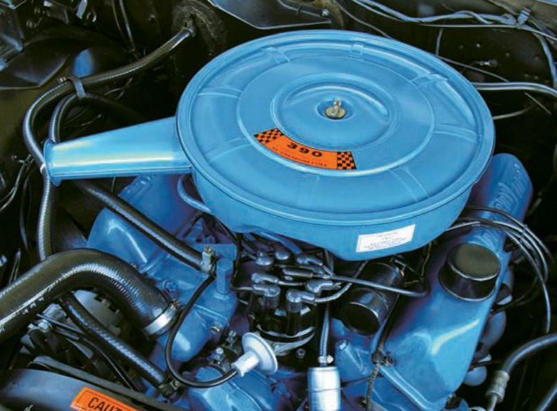
The 390-cu.in. V-8 was returned to stock appearance with the proper factory air cleaner and original Autolite 4300 four-barrel carburetor. A Pertronix electronic ignition hides under the distributor cap.
