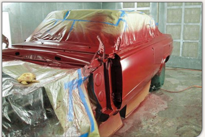
Using Restoration Shop products, primer was followed by three applications of color tinted to match Signet Royal Red. Proper cure time was permitted between the applications of primer and paint, as shrinking primer can lead to cracked paint later on.
