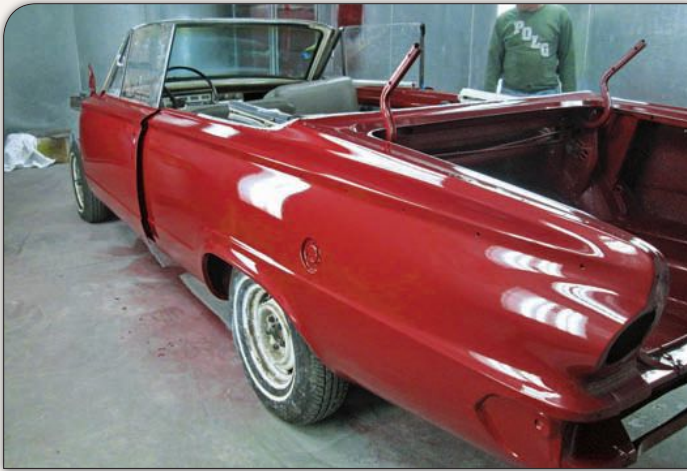
After color, the body was sealed in three carefully applied layers of clearcoat. Again, proper curing time was allowed before the body was wetsanded with 1500-grade paper that ultimately provided a smooth finish. Buffing brought out the rich sheen.
