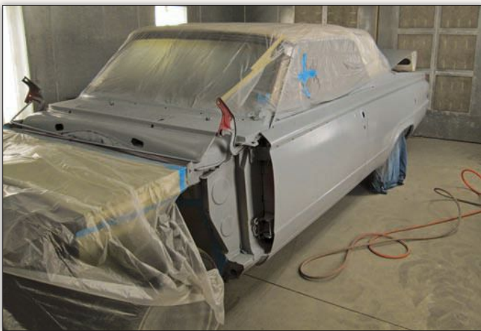
Once all of the slight imperfections on the body panels had been carefully smoothed out, the engine bay and interior were masked off with plastic. Two coats of two-part epoxy primer were then applied in a professional-grade spray booth.
