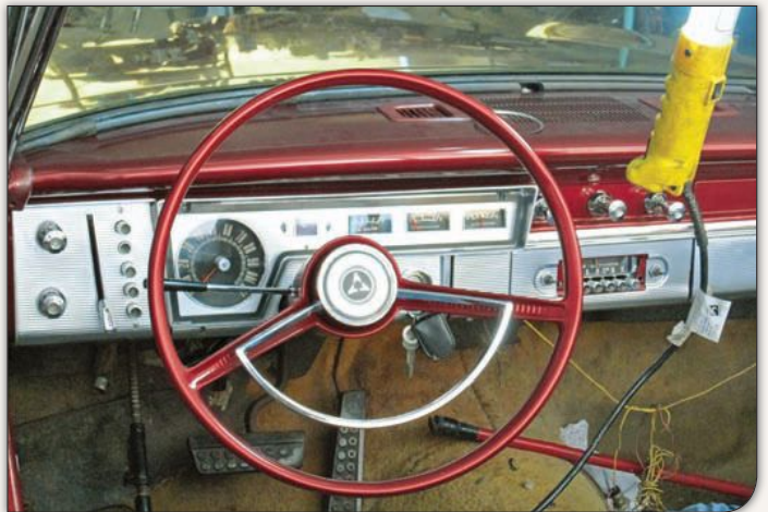
With its gauges and trim refinished and installed, the dash is complete. So, too, are the steering wheel and column, meaning the Dart is once again capable of moving under its own Slant Six power.
