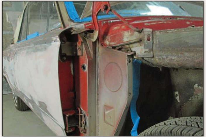
Even after removing the fenders, the team of restorers didn't find any corrosion that would need to be eliminated. Here, a little over a year's worth of bodywork is well under way, with the continued application of body filler and hours of sanding.
