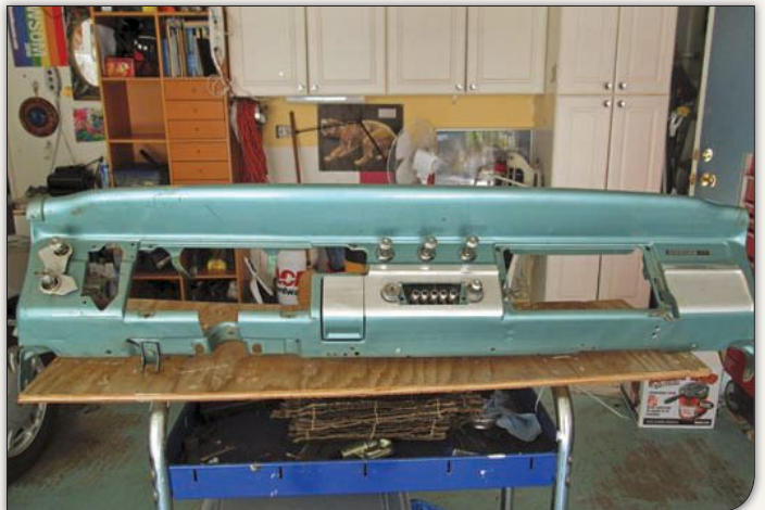
Each Dart, regardless of interior trim, carried a standard instrument panel arrangement, controls and decorative trim. The radio was optional. This is also a replacement from the parts car that was refinished to match the Signet Royal Red paint.
