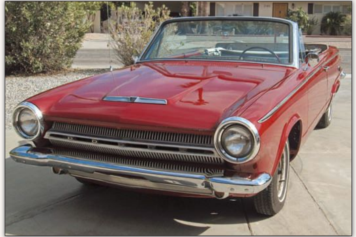
At this stage, body and trim is now complete, including the restoration of the protruding aluminum headlamp trim rings. This is departure day for the Dodge as it was shipped off to Classic Auto Restyling for a reproduction GT interior and top.
