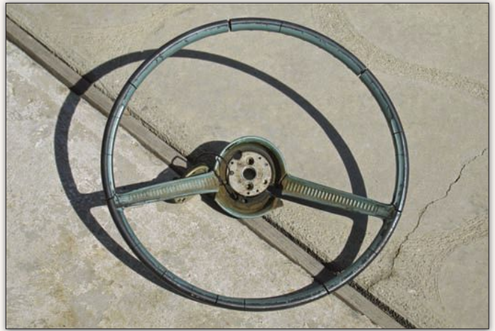
Look closely and you will note that the two-spoke steering wheel has several fissures along the rim. This wheel was sent out to be repaired and was then refinished to match the body color. Its chrome horn ring was replated at the time.
