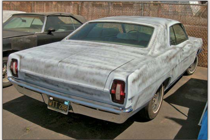
Once the body work had been completed, the remaining trim was masked before a protective yet thin layer of primer was applied to protect the sheetmetal. This was the first of two applications of primer the Formal Roof GT was to eventually receive.
