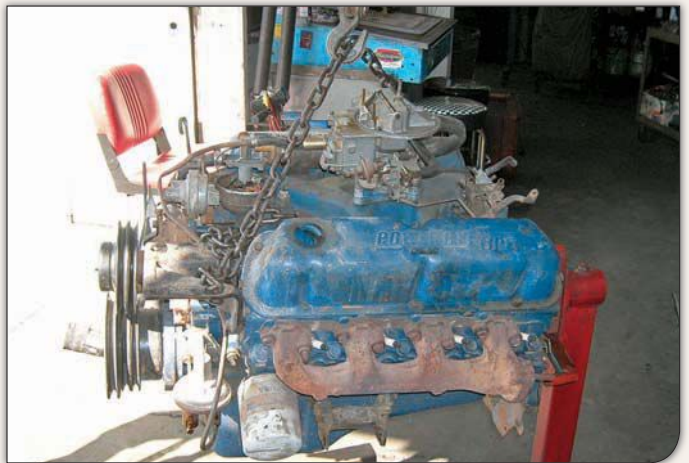
Having been rebuilt seven years prior, the 9.0 compression, 210-hp 302-cu.in. engine was removed again. This served two purposes: It permitted access and cleaning of the front unit-body structure, and eased the restoration of the engine's exterior.
