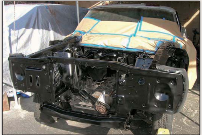
After the engine bay and surrounding unit-body structure had been cleaned, the rest of the body was masked off before primer and a coat of semi-gloss black paint was applied. It was given a proper cure time before the area was repopulated.
