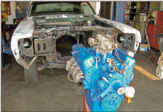
At this stage, the front fenders have been bolted into place and realigned with the rest of the body. The 302-cu.in. engine has also been pulled from hibernation and prepped for its return to the chassis with a fresh coat of Ford Engine Blue paint.
