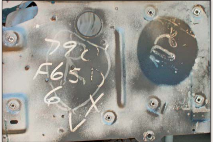
As the engine bay was being media-blasted, great care went into documenting factory markings uncovered on the radiator support panel and firewall. Doing so enabled the owner to have them replicated later in the restoration process.
