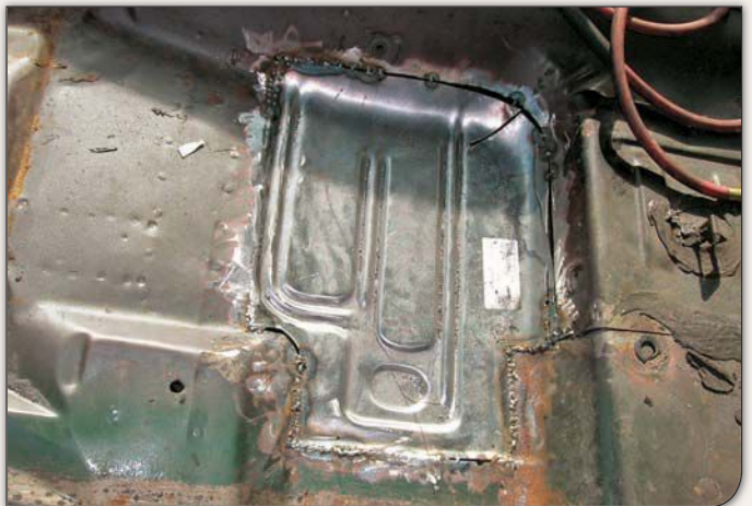
In spite of its deteriorated condition, the Ford fortunately had not succumbed to copious amounts of damaging rust. While surface rust on some body panels was easy to rectify, the only patch panel the GT required was this section of floorpan.
