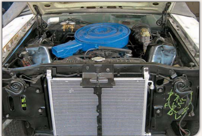
Reassembly is already in full swing in the engine bay. With the engine in place, the front section of wiring harness has been reconnected to most of its associated components. Note the replicated factory marking on the radiator support panel.
