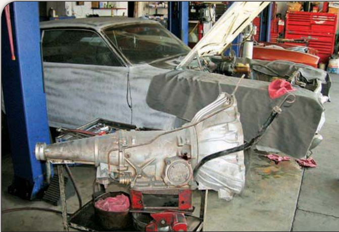
Ford's C4 automatic transmission was also separated from the Torino a second time. Like the engine, it was cleaned after its prolonged slumber and placed in protected storage while the engine bay was receiving its refurbishment.
