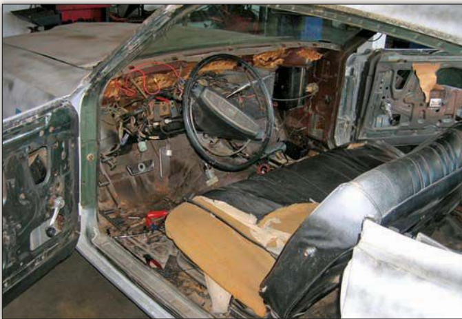
The Torino's front bench seat had clearly seen better days and was scheduled to be reupholstered later. At this early stage, the dash and instrument panel, door panels, and front section of floor carpet have already been removed.
