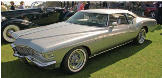
This striking fastback is the 1971 Buick Silver Arrow III—one of Bill Mitchell's Riviera concepts. It's powered by a 455 Stage 1 V-8.
