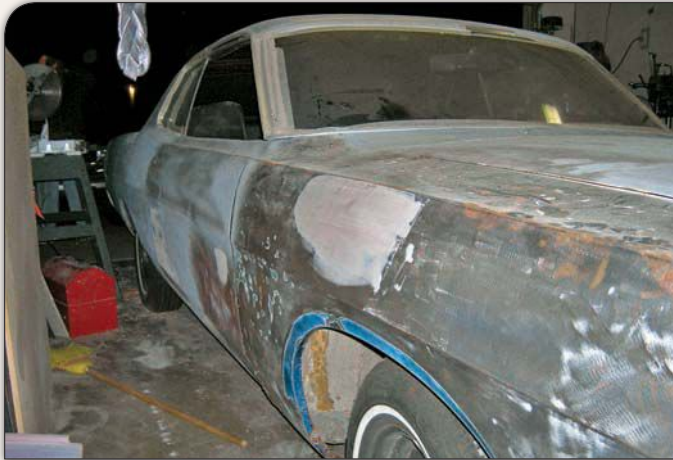
The Torino GT's body was stripped of its remaining paint and surface rust using various grades of sandpaper. Leaving the body panels in place helped retain its natural lines as skim coats of filler were applied and sanded to smooth imperfections.
