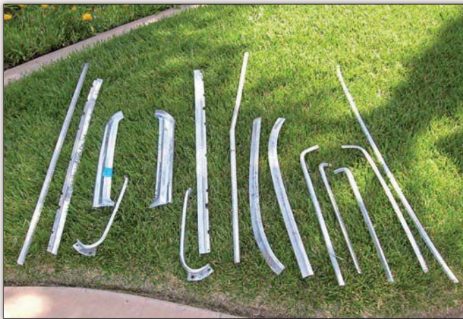
Here, trim has been carefully arranged according to which side of the car it had originated on. It was also inspected for damage, which helped determine which pieces would need either simple buffing or complete refinishing.
