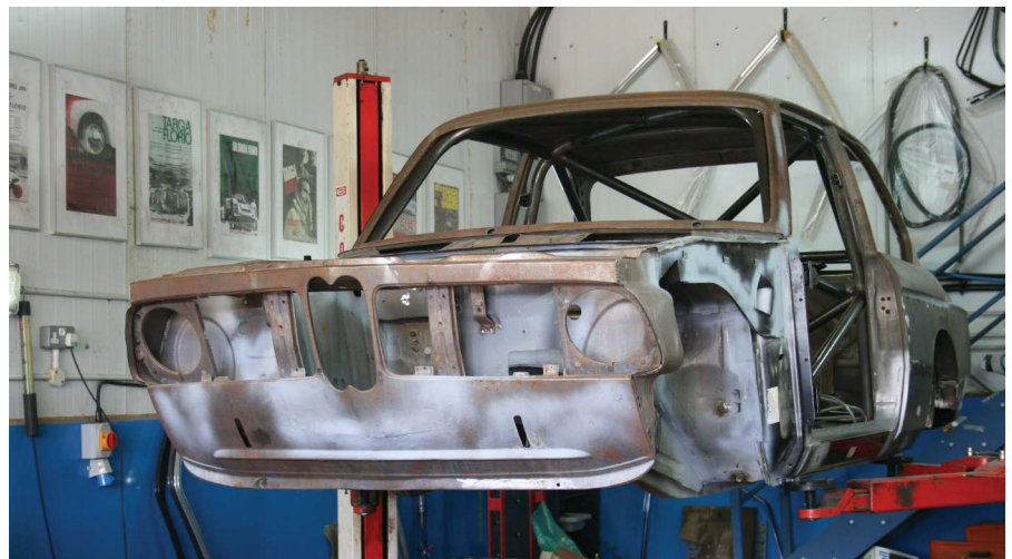
OK, it's not a Porsche. This is an ex-1971 Monte Carlo BMW 2002 that Nick is restoring to Group 2 specification. It's been a long-term project because Porsche works keeps rolling in
