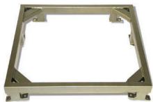
Frame Jig For 911 and 912 suspension pan replacement Duplicated from original tools T52-863
