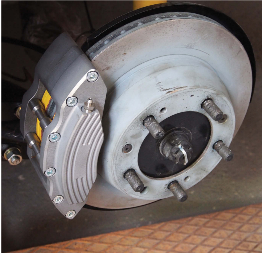
Above: Billet four-pot calipers from R-to-RSR is part of a kit to upgrade brakes on a SWB car. Six-pot fronts will be fitted next
