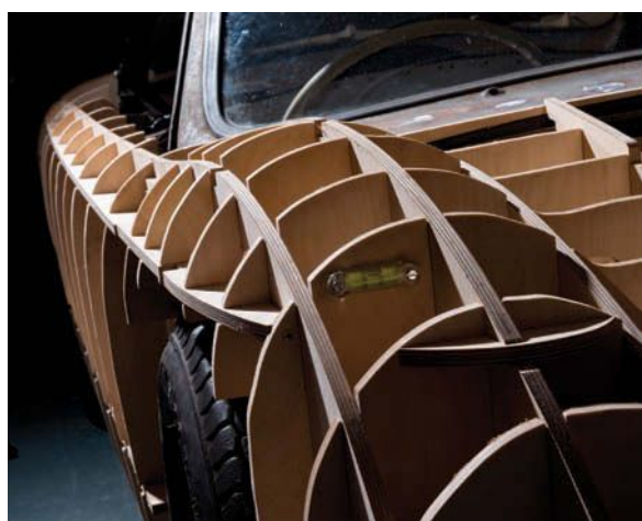
Steve Wright (left) with Ian Clark - they share driving duties on Steve's 356 (above, at Castle Combe), with Ian carrying out the mechanical preparation. It's a team that's starting to make its mark... Okrasa-powered Special (right) now awaits its handmade aluminium body. Wooden formers establish shape
