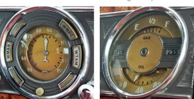
A bank of five gauges is centered on the dash; the middle gauge is actually an AM radio. Oddly, the fuel/oil pressure gauge is offset to the far right.
