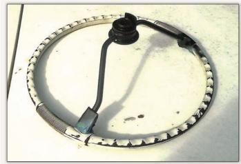
The original "steering wheel" was just a rusted metal ring, so after Dan Morton, webmaster of www.59plymouth.net, gave him a replacement steering wheel, Richard lightly sanded the rim, then applied three coats of Rust-Oleum Gloss Black Appliance Epoxy.
