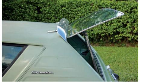
Oscar has a pair of hydraulic struts to replace the tired originals that hold open the Fairway Green Kammback's rear window. This is the only external access to the luggage area.
