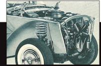
Now note the difference with Nash and Rambler. Huge members extend from windshield to grille, surrounding the engine, bracing it from all sides with rigid impact absorbing structures.
