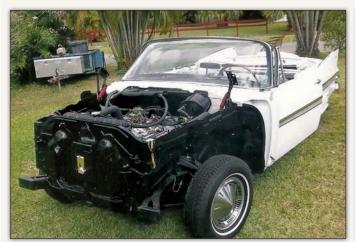
After the body was painted and the engine and transmission installed, the radiator was bolted to the chassis along with both inner fenders. This allowed the radiator to be installed and hoses to be connected to the engine, along with the horns and hood hinges.
