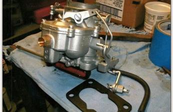
The replacement engine had a two-barrel intake, so Richard decided to keep it and buy a used two-barrel carb instead of switching to a four-barrel set-up. He now regrets that, due to the two-barrel's poor gas mileage. It was rebuilt prior to installation.
