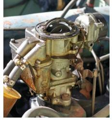
A single one-barrel Carter YF carburetor has proven more than adequate to feed the Gremlin's base inline-six engine.
