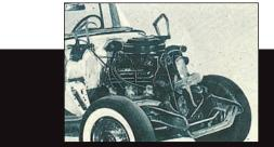
See the shortcomings of a typical car with old-style construction. No impact absorbing protection above the frame... greater tendency to force engine into passenger space in a collision.
