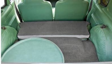
When the Gremlin was introduced in 1970, a basic two-seat model was available, while the four-seater was more costly. The twoseater was gone by 1973, and this example shows how the seatback folds over the sculpted base to provide a nearly flat cargo floor unfortunately interrupted by the full-size spare wheel.
