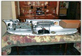
There's nothing like the comfort of using the kitchen table to reassemble the instrument panel. After a single coat of epoxy primer, the backside was painted white, as per the original, then the topside was refinished with several coats of gloss black.
