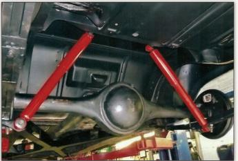
The replacement axle and differential assembly came from Richard's parts car. It was rebuilt using new bearings and seals, and the original 3:31-ratio gear set was retained. It was finished in the correct semi-gloss black, while new rear shocks were sprayed red.
