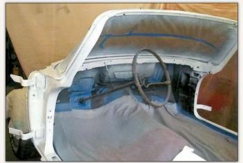
Instead of spraying the body in one shot, it was easier for Richard to spray the car in sections. Using easy-to-remove blue tape, the entire firewall, floor pan and both sides of the windshield were covered with thick autobody paper for maximum protection.
