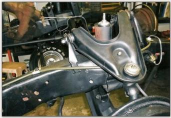
Every wearing component, such as ball joints, tie-rods, bushings, bearings, seals and shocks was replaced with a new part. The old rusted gas and brake lines, and brake flex hoses, were also replaced, including the little brackets that hold them onto the frame.
