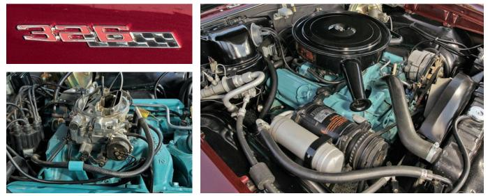
The original 326 H.O. V-8 engine was bored .030 over and upgraded with a longer-duration camshaft and a 650-CFM carb during its rebuild.
