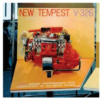
A cutaway of a V-326 is displayed at a 1963 auto show.
