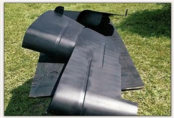
Right-side rear armrest was fabricated using the left-side armrest as a mirror image pattern because the original armrest was rusted beyond recognition. Both armrests were sent to SMS Auto Fabrics in Oregon to be covered so they would match the door panels.
