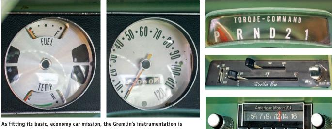
As fitting its basic, economy car mission, the Gremlin's instrumentation is barebones, but like the Mustang, this car could be fitted with an incredible range of options and accessories. This one has a column-shifted automatic, air conditioning and an AM radio, but a denim-like Levi's interior was also available.
