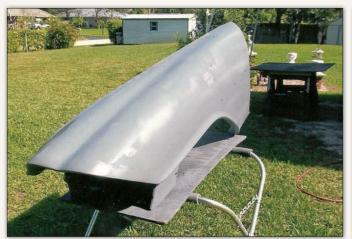
Both front fenders, doors and hoods were refinished separately. Just a few small spots required a thin layer of lightweight body filler, followed by a coat of light gray epoxy primer, then two coats of primer/sealer. All the painting was done by Richard.
