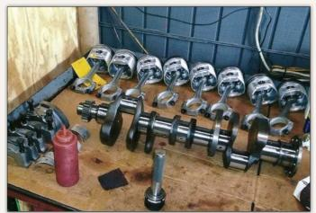
Machine Shop in nearby Lake Park to be machined and rebuilt. The shaft was cut .010, polished and balanced for smooth operation.
