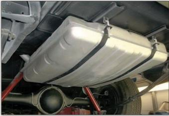
Gas tank is original, but prior to being repainted, it was cleaned in a hot tank and the interior filled with a special sealer followed by several coats of silver enamel on the outside. The straps were media blasted and then refinished in semi-gloss enamel.
