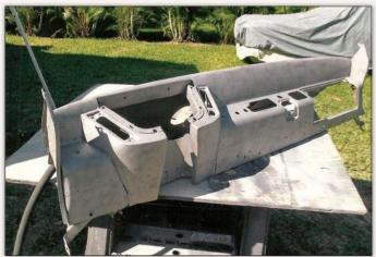
After the instrument panel had been removed and all the knobs, switches and wiring had been taken off, it was sandblasted down to bare metal using 30-grade media abrasive. After a second blast using finer 60-grade media, it was primed and painted.
