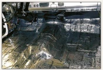
To help prevent unwanted road noise from infiltrating the cabin, a layer of Eastwood's Thermo-Coustic Sound Deadener barrier was installed all over the floor and on the entire firewall. Made of a butyl rubber membrane, it sells for about \$120-\$150.
