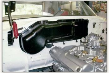
Using nothing more than a rattle can, the heater housing was cleaned, primed and painted with Rust-Oleum Gloss Black Appliance Epoxy. The heater core was flushed and tested before installation, and all new rubber gaskets and drain flappers were installed.
