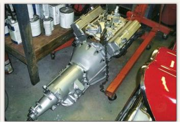
With the rebuilt and painted V-8 now back from the machine shop, the intake, valve covers, exhaust manifolds and engine mounts were installed before the engine was bolted to the transmission. Then the unit was lifted into place using a two-ton engine hoist.
