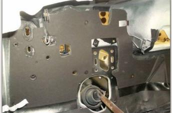
A new factory-correct interior firewall insulation pad was sourced from Gary Goers. Specializing in Chrysler parts, Gary also rebuilt the rubber-covered vent doors and supplied all weatherstripping, rubber bumpers and the gold "V-8" trunk emblem.
