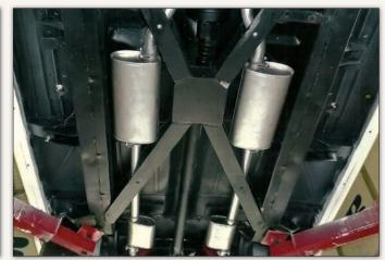
From the exhaust manifolds back to the dual exhaust tips, the exhaust system had been replaced with new pipes, resonators, mufflers and clamps. Made of mild steel, they were refinished in high-temperature silver heat paint to protect them from rusting.
