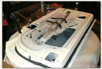
Each door's window operating system was refurbished and then reinstalled with new glass run channels and inner and outer door whiskers. The interior of the doors was sandblasted, wiped with Ospho, sprayed with two coats of epoxy primer and seamsealed.
