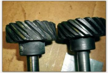
A new oil pump and distributor driveshaft, which is gear-driven by the camshaft, was installed because the original gear had several broken teeth. An NOS shaft and gear assembly was found at Len Dawson's Deception Pass Auto Parts in Washington state.
