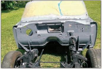
After the body was bolted back on the frame to have the replacement The replacement 318-cu.in. V-8 engine was sent to Lake Park Auto floor pans precisely aligned, it was lifted off again in order to be sprayed with a single coat of Eastwood's Encapsulator Epoxy, followed block was bored .030-over and fitted with new pistons; the crankby two coats of urethane primer/sealer.
