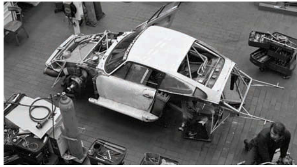
Far left: The 935/77 had revised bodywork, which included a new rear section with rear screen which had to fit over the original screen. Rear bulkhead was moved to allow space for intercooler
