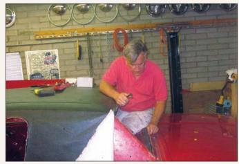
With the interior gone, it was possible for the team to remove the vinyl top without putting stress on their lower backs. As that process gets under way, the last bits of the original weatherstripping are being eliminated from its channel.
