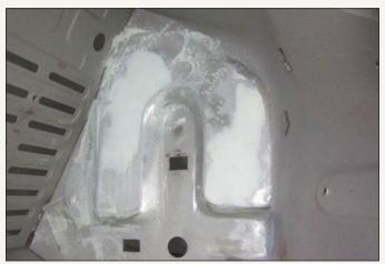
After media blasting, the battery tray was cleaned of debris. Small patch panels were fabricated and butt-welded into place, and then carefully ground flat. To help smooth the surface for a factory look, a skim coat of filler was applied and sanded.
