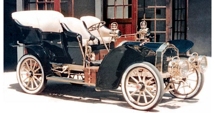
This fine-looking 1905 Packard Model N touring car features, like all Packards of the time as well as many other American cars, a righthand-mounted steering wheel. It would be a few more years before American automakers would settle on left-hand steering.
