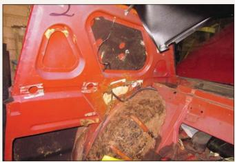
At this point, a significant portion of the interior has been removed, exposing the vast C-pillar substructure. To the relief of the team, none of the metal in this area had been compromised by rust, nor had vermin destroyed the original insulation.
