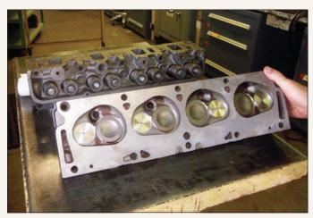
Each of the cast-iron cylinder heads was also cleaned, stripped and evaluated before it was rebuilt. The face of each was milled to true so it would mate with the block's surface, and then OE 2.02/1.57inch intake/exhaust valves and OE springs were installed.
