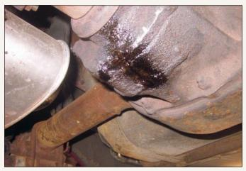
Further inspection of the undercarriage revealed that there were other problems, bolstering the decision to restore. It was discovered that gear oil was pooling on the underside of the differential, confirming that there was an oil seal failure.
