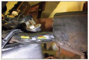
Although the Thunderbird had been able to ward off rust through the decades, the first hint of potential trouble due to rodents was discovered when the wiring harness was being removed from the body: Mice have chewed through the wiring's insulation.
