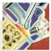
Pontiac's new wedge-shaped combustion chamber with 8.0:1 compression ratio squeezes tremendous power out of every gallon of gas. And because the chamber is completely machined and includes a large guench area, you are assured of a smoother, quieter power flow.
