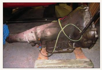
The original C6 three-speed automatic transmission was removed from the car along with the engine and then separated afterwards. Already known to have a leak from the initial inspection, it was delivered to a transmission specialist for a complete rebuild.
