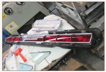
Another subassembly has been completed during the initial body and paint process; this time, the full-width taillamp and corresponding bezel. Earlier, the unit's trim had been polished and the lens carefully cleaned; new bulbs were also installed.
