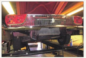
Utilizing the shop lift eased disassembly of the Thunderbird's lower exterior trim and panels. Here, the front headlamps and bezels have been taken off, along with the lower front valance, in preparation for the removal of the bumper.
