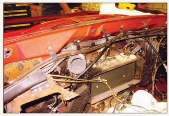
As the instrument panel and padded dash are removed, it becomes clear that small vermin had occupied its recesses. The remains of a mouse nest were uncovered; however, damage had been surprisingly minimal, in spite of the reputation of rodents for mayhem.
