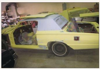
In order to prevent the bare metal of the body panels and shell from flash-rusting, even in the dry desert climate, a protective layer of epoxy primer was applied, at which point exterior surfaces could be smoothed with a skim coat of body filler.
