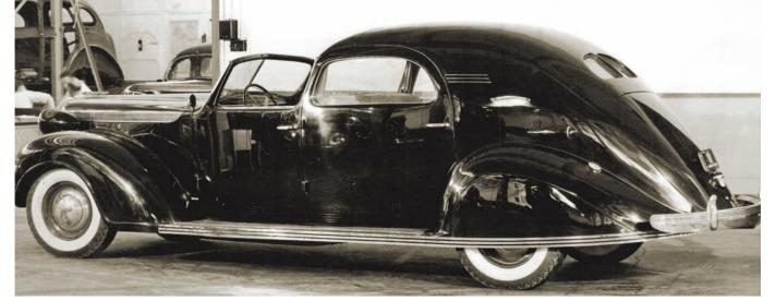
At the Briggs Body plant soon after completion, with what could be — in the background at the far left — the body of the donor car, which had been removed from the chassis used to build the town car. Note how the wide plated trim band starts at the back of the front fender and wraps completely around the back edge of the body.
