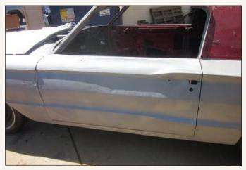
Media blasting of select areas of the body eliminated both an older repaint and the factory layer, exposing bare steel. Only a few surprises were found, including damage to the driver's door, which was replaced with a perfect door from a parts car.
