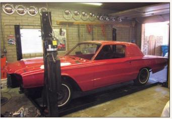
At this stage, most of the disassembly has occurred. To help expedite delivery to a local facility for media blasting, many of the major body panels have been reunited with the chassis, while the entire suspension system remains bolted into position.
