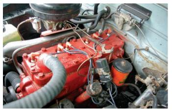
Based on Hudson's eight, the 202-cu.in. flathead six makes 104hp; it's peppy and economical. Radiator overflow tank is only modern item.
