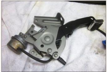
As the body received corrective treatment, smaller subassemblies were carefully restored. This is the parking-brake foot pedal and some of its corresponding linkage fully reconstructed and ready for installation when needed, saving reassembly time.
