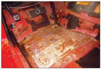
No matter the body style, the driver's side floorboard sees more moisture abuse than the other sections. As fortune would have it, the rust seen here was only superficial, eliminating the need to make repairs with patch panels at a later date.
