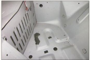
As is often the case, the steel battery tray had corroded over time. Again, however, damage appeared to be surprisingly minimal. While media blasting revealed that corrosion had spread to a greater extent than was first thought, it hadn't migrated to the inner fender.
