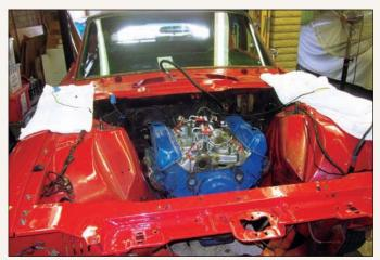
With both the engine bay and the big V-8 stripped of bolt-on and auxiliary electronics, final preparation is underway to pull the 315hp 390. A keen eye will note that the engine's intake manifold is an aftermarket piece; an OE replacement was needed.
