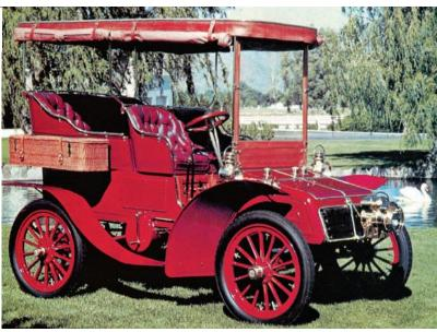
This 1903 Packard Model F is set for a fun drive in the country, with its surrey top, roll-down side enclosures, and handsome picnic baskets. Note the details of this car: flared front fenders, red leather seating, brass lamps and wood-frame windshield. Notice, too, that the crank is mounted on the side.
