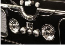
The tastefully trimmed interior gives no hint as to the complexity of this restoration. The body's ash framing had to be replaced. Yes, the clock on the dashboard not only works, but keeps time reliably. Round knobs are radio controls. Pushbuttons raise and lower the town car's glass divider. Knob beneath dash ahead of shifter activates overdrive. Note the sunburst pattern on the speedometer.
