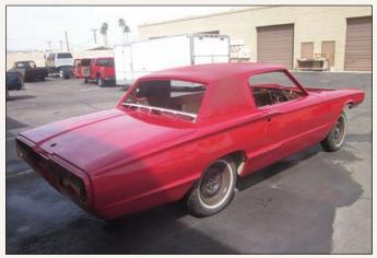
Single-stage urethane, matched to the original factory red hue, was finally applied to the body shell and other exterior body panels. Although exact details of the process are not known, it was permitted to cure before being returned to the restorer.
