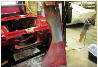
Both sides of each body panel were carefully removed and inspected. Here, it's the right-front fender that's being inspected, and upon closer examination, only a trace of surface rust can be seen. Holes for fender trim are apparent near the leading edge.
