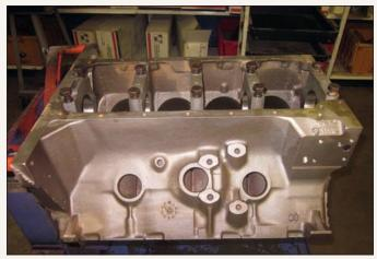
After the engine was removed from the Thunderbird, it was sent to an engine specialist. There, it was completely stripped, evaluated for hairline cracks and fully cleaned before the cylinder bores were subjected to a standard .030 overbore.
