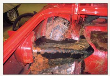
Focus quickly shifted to the trunk. It's not unusual to find corrosion below a trunk mat; however, in this case, upon its removal, nary a speck of oxidation was found. This fact ultimately helped speed up the whole process, as only a basic cleaning was needed.
