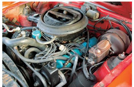
Oscar loves the sounds that the vacuum-operated cowl induction system makes when he hammers the accelerator of the potent 401-cu.in. V-8 under the hood.
