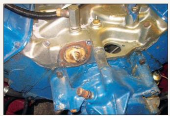
In spite of earlier work by previous owners, the original FE-Series 390-cu.in. engine had been retained and repainted, which meant that when its bolt-on components had been removed to facilitate its extraction, expected minor corrosion was uncovered.
