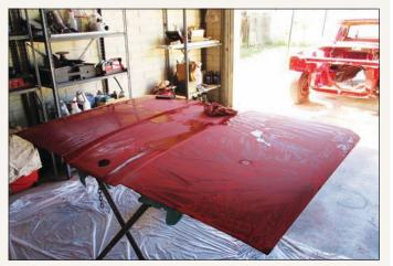
Although time was lost, the new shop embarked on correcting the paint. At the time this image was taken, the new PPG single-stage paint was being wet-sanded. Join us next month, as the restoration continues to the 113.2-inch wheelbase chassis and interior.
