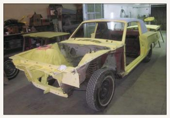
Over the course of the next four months, progress with regard to bodywork seemed slow. After the filler had been block sanded smooth following the common step process of using progressively finer sandpaper, a sealing layer of primer was applied yet again.
