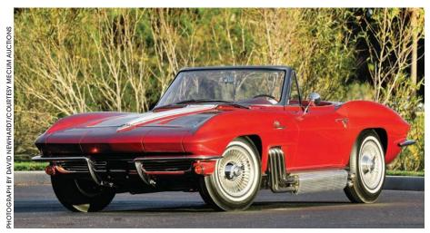
This 1963 Corvette was built for Knudsen and is reminiscent of the blue one, built for retired GM VP and styling chief Harley Earl. It's Fire-Frost Red with a white racing stripe, has custom interior and a four-speed, and a side-exit exhaust for its fuel-injected 327.
