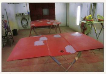
Now five months into the process, yet another application of primer revealed that not all surfaces were as smooth as they should have been. More filler in select areas was applied and continuously sanded smooth before paint could at last be shot.
