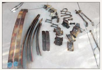
After the second repaint had been accomplished, restorer Ward Gappa and his team stripped the suspension from the chassis, including the rear semi-elliptic leaf springs, both of which have been separated to get them ready for media blasting.
