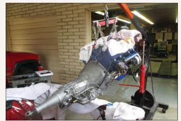
After testing, the engine — reunited with the C6 three-speed automatic earlier — were returned to the chassis as a subassembly. Though it looks cumbersome and requires careful guidance, they are easier to install together than as separate units.
