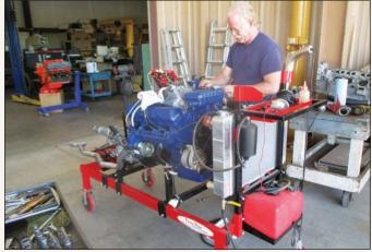
Rather than break in the rebuilt V-8 while it's bolted in the chassis, it was done on a special engine stand. In this setup, it would be easier to correct any problems that might arise without having to remove it from the chassis, risking damage to the new finish.
