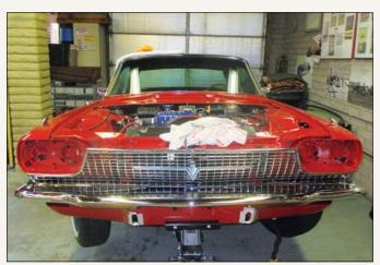
In spite of the installation of the front fenders and the replated bumper and grille, there was still a long list of tasks that needed to be accomplished, including adjusting panel gaps, refitting the hood and finishing the electrical system and remaining trim.
