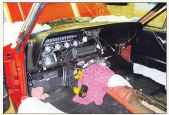
Focus next shifted to the interior. Installed first was the rebuilt instrument cluster, followed by the refinished pedals and floor carpet. The restored padded dash came after much of the wiring harness had been reconnected to key components.
