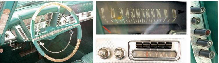
The Sport Fury for 1959 was outfitted with several distinct features, including the unique upswept exterior side trim and the half-padded steering wheel. Besides the Deluxe radio, pushbuttons were also used to engage the three-speed TorqueFlite automatic transmission.
