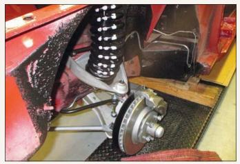
Accompanied by new bushings and ball joints, the suspension and brake systems were rebuilt and reinstalled; the two-piston calipers had also been rebuilt. Note that the front coil springs were refinished to factory color, including paint dab markings.
