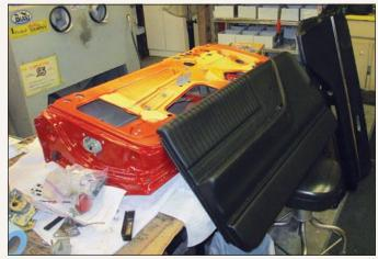
To prevent a restoration project from getting bogged down, it's helpful to stay one step ahead. Here, new door panels are in the process of being test-fitted, as the other body panels and main shell receive a second corrective coat of PPG single-stage urethane.
