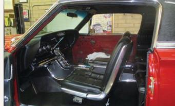
Look closely and you'll note that, along with the front bucket seats, most of the interior has been completed, including the C-pillar trim, rear seats, restored center console and steering column. Note the exterior top trim has also been returned.
