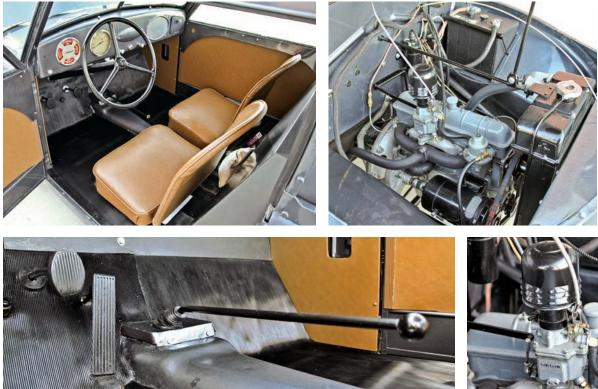
The Crosley pickup's interior is spartan, but boasts a full compliment of gauges and a speedometer. Power comes from Crosley's 44-cu.in. cast-iron fourcylinder, backed by a T-92 Warner threespeed gearbox.
