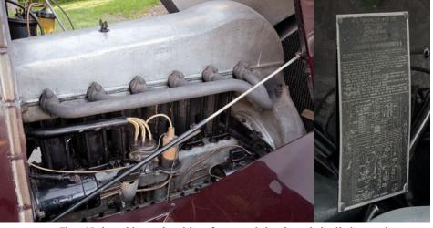
The 10B ducted its engine-driven fan to cool the air-cooled cylinders; maintenance information and electrical schematic were included with chassis plate.
