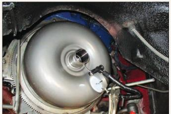
Everything from the flywheel to the tiniest of tolerances were checked. The cause of the vibration was discovered to be pieces of walnut shell that had been used to clean the radiator; several small bits had passed through the cooling lines into the transmission.
