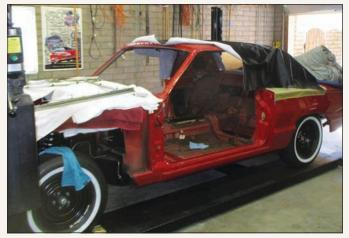
With the chassis rebuilt, the Thunderbird was another step closer to completion. Work could now progress to resurrecting the exterior, including the installation of a new black vinyl top. Protecting the new paint are a number of microfiber towels.
