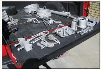
Components were sent in batches for media blasting. Having been returned here are suspension and brake system parts, the engine's exhaust manifolds and air-cleaner assembly. Parts requiring paint received treatment quickly to prevent flash rust.
