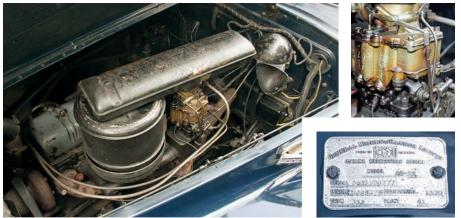
The 248-cu.in., two-barrel-carbureted, 107-hp straight-eight starts instantly and offers lots of hill-pulling torque. The data plate reveals its GM of Canada Ltd. origins.
