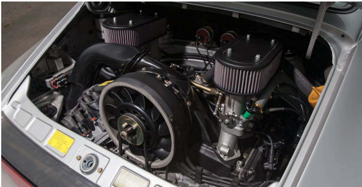
Graham Ridgway's 3.0 RS-inspired car runs a 3.8-litre motor, with PMO throttle bodies, 11.5:1 CR, Mahle cylinders and JE pistons. It's hooked up to a G50 trans with Quaife differential
