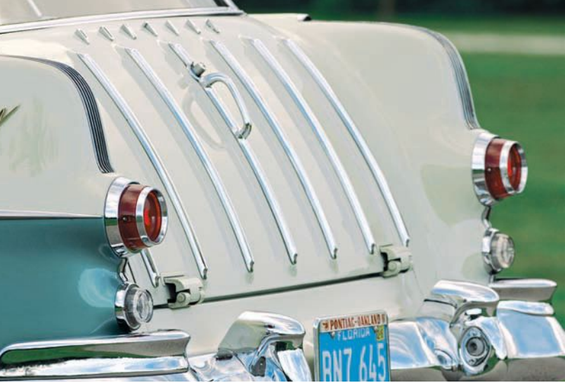
Roof and tailgate, including hallmark bright strips, are shared with Chevrolet Nomad. Carpeted cargo area is exclusive to Safari and helps protect luggage and deaden road noise. Backup lamps were optional. All 1955 models had Silver Streak trim.
