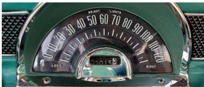
Hooded speedometer has redline indicator instead of needle; all gauges are illuminated green at night. Climate controls adjust Venti-Heat under-seat heater that works like a modern heated seat but uses a second heater core in lieu of electrical components.
