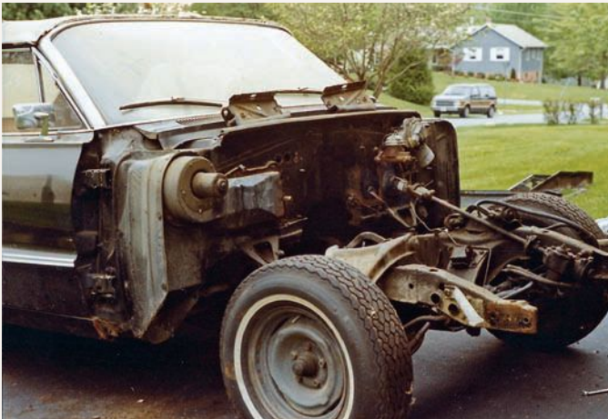
The engine and transmission, as well as the rest of the front body panels and associated support brackets, were removed. At that time, it became apparent that rust extended beyond the fender's outer skin; in this case, the lower cowl was badly corroded.
