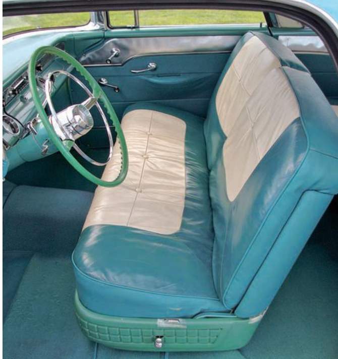
The wide, leather-covered bench seat is very comfortable, and is adjustable fore and aft. Power assist was optional.
