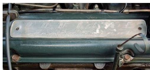
Strato-Streak 287-cu.in. engine was Pontiac's first OHV V-8. With its two-barrel carburetor, hydraulic lifters and 8.0:1 compression ratio, it developed 180hp. Dual exhausts were not available.
