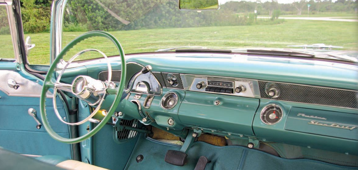
Instrument panel design is handsome and usable. Centrally mounted glovebox door is flanked by fuel/oil pressure gauge and clock; view of the former can be hindered by gearshift lever. Bright finish on top and chrome windshield trim can create glare issues.
