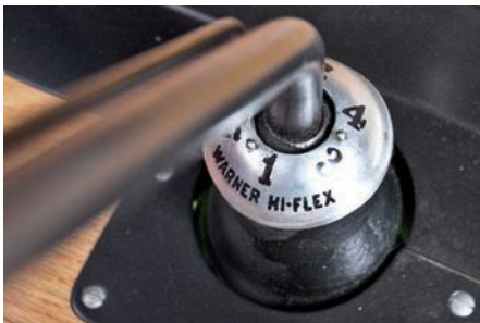
The optional Warner Hi-Flex four-speed takes a little getting used to, as first and third are at the bottom of the pattern, while second and fourth are at the top. Powering this Graham is a 208-cu.in. Dodge six-cylinder.
