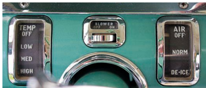
Hooded speedometer has redline indicator instead of needle; all gauges are illuminated green at night. Climate controls adjust Venti-Heat under-seat heater that works like a modern heated seat but uses a second heater core in lieu of electrical components.
