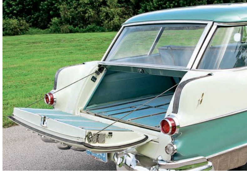
Roof and tailgate, including hallmark bright strips, are shared with Chevrolet Nomad. Carpeted cargo area is exclusive to Safari and helps protect luggage and deaden road noise. Backup lamps were optional. All 1955 models had Silver Streak trim.
