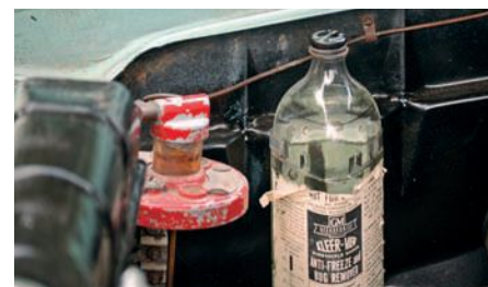
The 288-cu.in. straight-eight engine had become frozen from decades of disuse, and had to be rebuilt. The radiator was re-cored when the original was found to be impossible to repair. The windshield washer was one of many factory options installed by the car's first owner.
