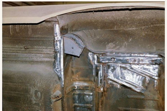
After being removed from the frame, the body was braced to prevent warping and placed on a rotisserie, providing easier access to the underside. Several precisely fabricated patch panels have already been carefully MIG-welded into place at this stage.
