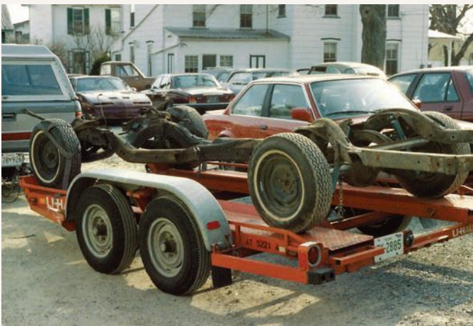
After a three-year hiatus, the Impala's restoration continued in early 1991. The body was lifted off, and the frame was delivered for a date with a media blaster. Fortunately, the cleansing did not reveal any fatigued metal.
