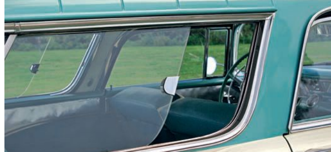
Sliding windows vent the interior, which is easily warmed due to large greenhouse. Slanted B-pillars and coupe doors set sport wagon apart.
