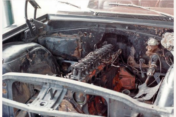
Removing the hood and several key front end trim items provided easier access to the 230-cu.in. straight-six engine, which was partially disassembled to shed weight, making the task of its extraction from the chassis considerably more manageable.
