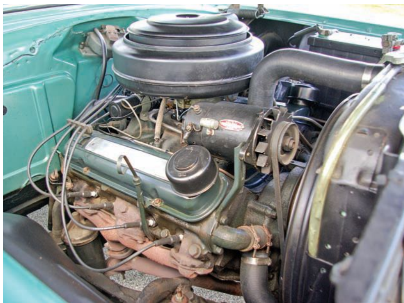
Strato-Streak 287-cu.in. engine was Pontiac's first OHV V-8. With its two-barrel carburetor, hydraulic lifters and 8.0:1 compression ratio, it developed 180hp. Dual exhausts were not available.
