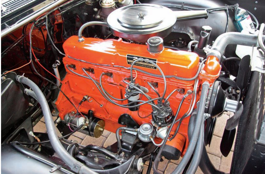
The vastness of space under the hood is apparent with the Impala's factory-original 230-cu.in. straight-six engine installed; this means that any detail flaws would be easily visible.
