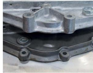
It's important to use a torque wrench when installing the tensioners, especially where early magnesium chain cases are concerned. Photo on far right shows left-side oil line in place
