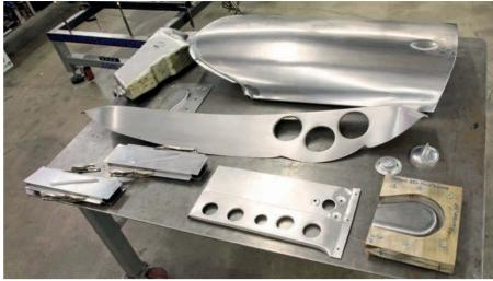
Planishing hammer and English wheel allow the skilled workforce to recreate virtually any shape of body panel in steel or aluminium
