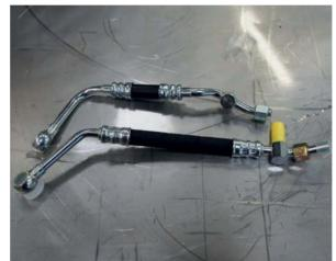
The complete pressure-fed tensioner upgrade kit - you'll need the longer extra oil line if fitting to early engine. Cam chain covers are aluminium, rather then the magnesium used on early engines
