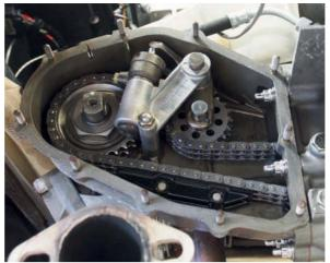
We had mechanical tensioners installed and decided to replace them with rebuilt 930-style hydraulic items, but one failed after less than 50 miles...
