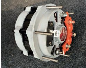
Changing the alternator on a 911 is a fiddly process but it had to be done as the diodes had failed in the original unit.
