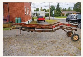
The next step was comparing the reworked frame against the corroded original. At first glance, it appears to be a perfect match; however, this was only the first part of the process. Note that threaded rod was used to make mounting-point comparisons.
