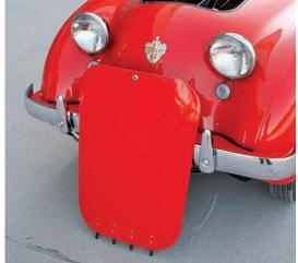
Removing the Hotshot's hingeless hood is as easy as twisting the keyed lock and lifting, exposing the 44-cubic-inch CIBA four-cylinder overhead-valve engine rated for 26.5 horsepower. Contemporary road tests regularly achieved speeds in excess of 70 miles per hour.
