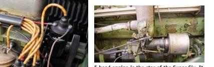
F-head engine is the star of the Super Six. It displaces 288-cu.in., produces 92 horsepower and features a balanced crankshaft for smoothness and high-speed capability.
