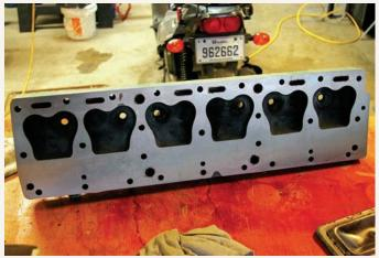
In order to avoid further issues with the top end of the straight-six engine, André had the mating surface of the cylinder head milled. This process provides a better seal between the gasket and head, helping to prevent coolant leaks.
