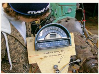
The Pontiac's original gauge cluster was bolted to a piece of plywood, and corresponding connections were made, enabling André to monitor the engine's status during initial break-in testing.
