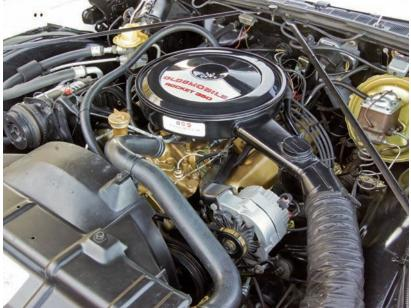
The factory-equipped Oldsmobile 350-cubic-inch V-8 was good for 180 horsepower and 275-lb.ft. of torque through the column-shifted Turbo-Hydra-Matic 400 transmission in 1974. Not quite the Rocket of years gone by, despite what the air cleaner promised, but, oh, so smooth.
