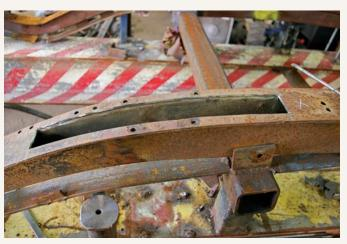
At several key positions, the frame's contours were too significant for the previously described bending method; it was determined that the metal would fracture. To prevent this from happening, they cut sections out of the bottom plate, exposing the channel within.
