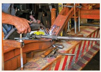
After the frame rails were sufficiently re-contoured, the pieces that had been cut from the bottom of the rails in order to facilitate bending without fracturing were welded back in place. The welds were later dressed to make the splice invisible.
