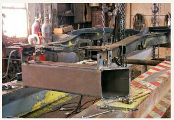
With the mounting points marked, the original frame was flipped over in order to begin to make a jig. To compensate for the frame's undulations, the front and rear mounts were elevated well above the platform using square tubing and plate steel.
