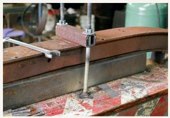
To maintain pressure where needed during the bending process, a makeshift but very effective clamp was fabricated using box tubing, threaded rods, nuts and washers. This system was employed at several locations along the length of each frame rail.
