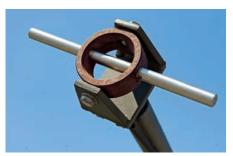
The "claw" of the Hucks Starter engaged a dog bolt on the end of the prop, which engaged the crankshaft to start an aircraft.
