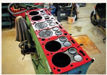
New crankshaft shell bearings have been inserted, and the pistons installed during the engine's second rebuild in 2005 — have been reinstalled, too, after it was ensured that none of the valves needed attention. Here, the new cylinder head gasket has been positioned.
