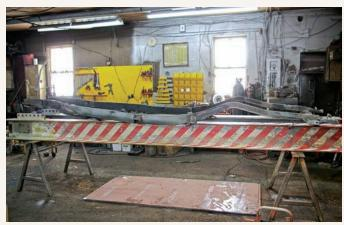
By the time André had obtained the new frame, two years had already passed since he had decided to restore the Pontiac. In this image, the difference in frame design has been discovered; fortunately, despite corrosion damage, the original remained true to its factory dimensions.
