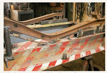
Although the center section of the replacement frame was not too far off from the original, the discrepancy was more significant in the aft section. Note that by the time this photo was taken, André had decided to remove the crossmembers to alter one rail at a time.
