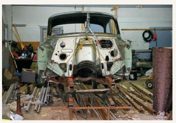
In spite of the misfortune that befell the body shell earlier in the restoration, its removal from the first shop proved to have some benefit, as it was conveniently on hand to serve as a second pattern for comparing with the reworked replacement frame.
