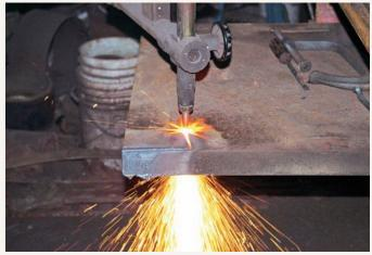
Blocks of solid steel were cut to assist with the process of bending the frame rails to match the jig, after taking internal measurements of the frame rails. The blocks spread the clamping force over a broader area, thereby preventing the formation of kinks or creases.
