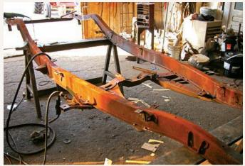
With the frame rails and crossmembers reunited, it was time to make final welds and adjustments to the body mounting points along the length of the frame. This was done with the frame in its normal position on conventional sawhorses rather than on the jig.
