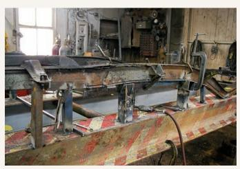
Next was the fabrication of new body mounts to replace the originals that had corroded away over time. These were critical, and making them now would save time later in the process. Note that a small side rail has been welded in place to help maintain frame width later.
