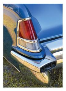
The left taillamp assembly swings open to reveal the fuel door. To achieve a lower roofline without sacrificing passenger headroom, the compartment floor dropped down between the frame rails. Consequently, the dual exhaust system was routed outside of them. Featuring resonators, mufflers and a crossover pipe near the rear axle, it terminates at bright tips through the rear bumper. Each fin of the wheel covers was hand fitted.
