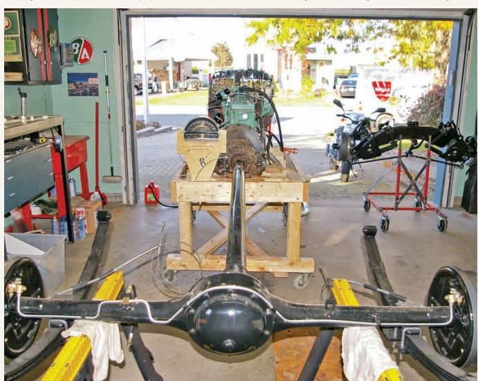
Rebuilt earlier, the differential/torque tube assembly was aligned via sawhorses and bolted to the transmission. Metal flex tubing was clamped to the engine's exhaust manifold and routed out the garage doors in anticipation of testing of the drive systems. Join us in the next issue as we learn about the restoration of this Canadian-born 1953 Pontiac Pathfinder's body.
