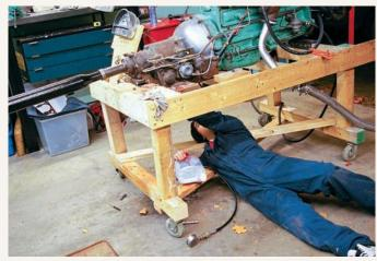
At this stage, both the engine and transmission have been rebuilt and reunited with one another. Jonathan is assisting the effort in securing them to a sturdy homemade wooden test stand while ensuring that all lubricants are at their proper fill level.
