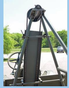
PTO-connected, chain-driven prop starter proved a relatively straightforward—and safer—alternative to hand-propping aircraft.
