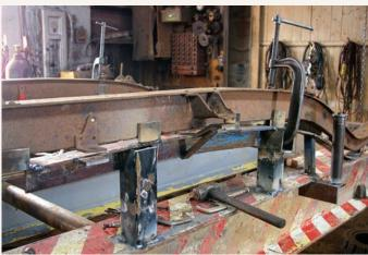
With the frame jig completed, it was time to drop the replacement frame into position and secure it using C-clamps. Initially, it was thought that the rails could be manipulated simultaneously, so each of the crossmembers remained riveted to the side rails.
