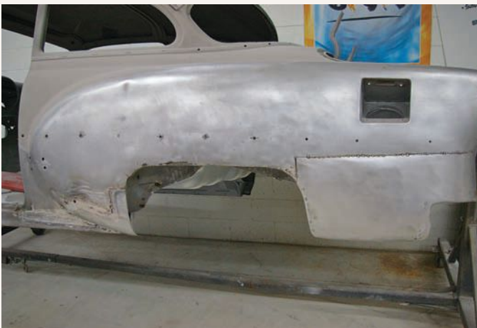
The same kind of damage that affected the right quarter panel also affected the left and had to be repaired similarly. Most of the work has already been accomplished in this image; however, if you look close, you'll see that rot still is present on the wheel lip.
