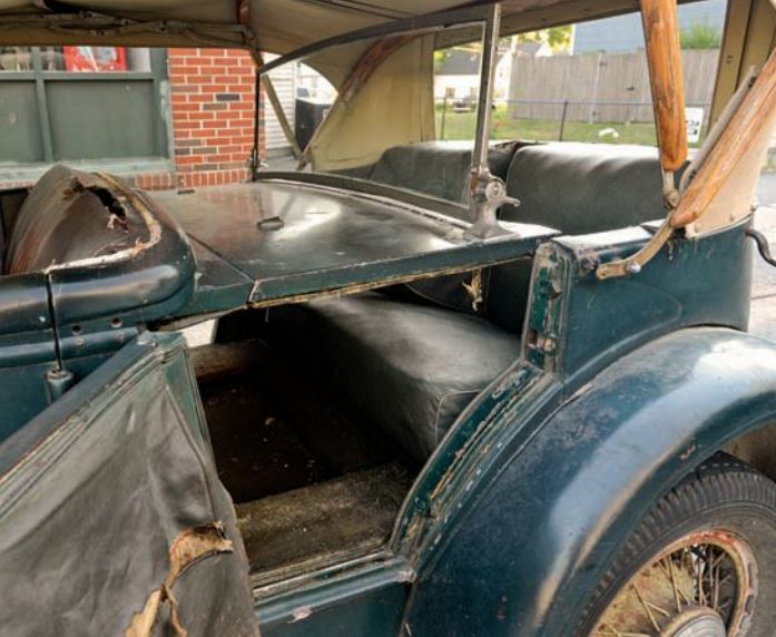
Filler panel behind the front seat flips up for rear-seat access. Owner has been driving this Franklin since 1954.
