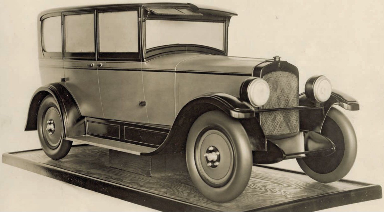
One model with two distinct, different halves. This showed customers how adding a belt molding or altering the design of the sunvisor could change the appearance. The radiator shell resembles a Reo or possibly an Oldsmobile of that era.
