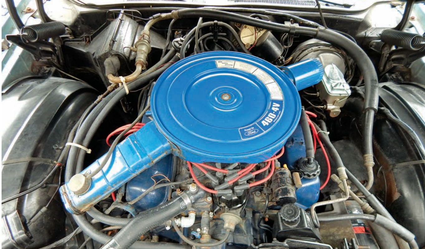
Four-barrel 460-cu.in. V-8 produced just 219 horsepower, but its stock in trade was creamy-smooth torque rather than outright power.
