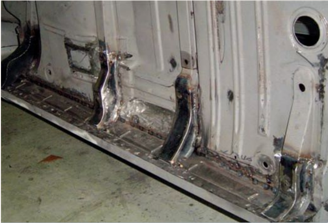
After several weeks of careful effort, each of the body's mounting points and bracing has been restored and tack welded into position. Seams are to be welded shut next, which will then be ground smooth; floorboard repairs have also been completed.
