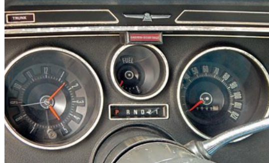
Color-keyed comfort was the name of Thunderbird's game in 1973. A clock and a 120-MPH speedometer are the gauges facing the driver; the AM/FM stereo cassette was an extra-cost option.
