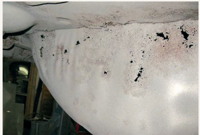
In all-too-typical fashion, the spare wheel carrier, stamped into the trunk floor, was found to be riddled with corrosion damage once media blasted. Patch panels were carefully fabricated from sheetmetal using the original steel as a template.
