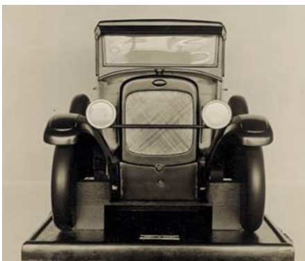
This generic radiator shell featured a crank-hole cover, emblem and radiator cap, and used a textured area to accurately represent the radiator core.
