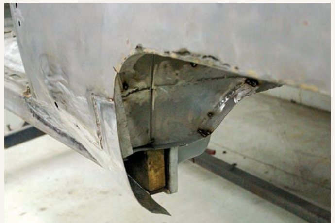
A testament to the amount of metalwork André's Pontiac required is present in this image. Not only had the outer quarter panel needed repairs, but so, too, did the inner fender structure and portions of the rocker panels. Note the temporary use of a wood stud.
