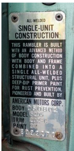
AMC reminds you that unitized bodies are sturdy. Codes indicate this car left the factory with roof and body painted Elmhurst Green.
