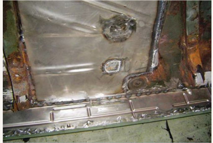
In 2010, the body shell was finally delivered to a second shop. The required work turned out to be more extensive than had been anticipated. Here a section of the floorpan has been replaced, as well as the inner rocker panel, both fabricated from sheetmetal.
