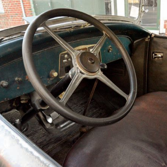
Franklin didn't use "dual-cowl phaeton;" instead, the Pursuit's body style is dubbed a sport touring. Minimal instrumentation includes a roller-type speedometer. The little spoon-shaped lever on the floor is the accelerator. Passenger compartment has never been restored.
