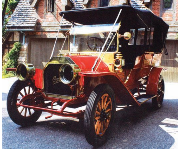
The top-of-the-line 1910 Overland Model 42 cost $1,500 and featured the larger 40hp four-cylinder engine with a sliding gear three-speed transmission. The 112-inch wheelbase chassis could be had with close-coupled four-passenger or five-passenger touring body.
