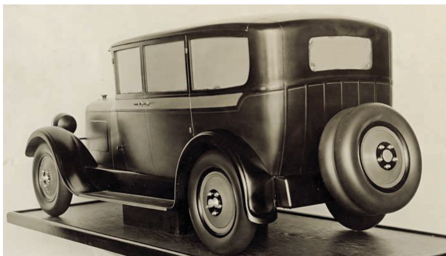
This is the only scale model in the numerous photos taken that has twin rear-mounted spare tires. The raised vertical body lines on the rear body panel represent cast, separate plated trim strips that would have been attached to a real body and were a styling accent that was popular at the time.
