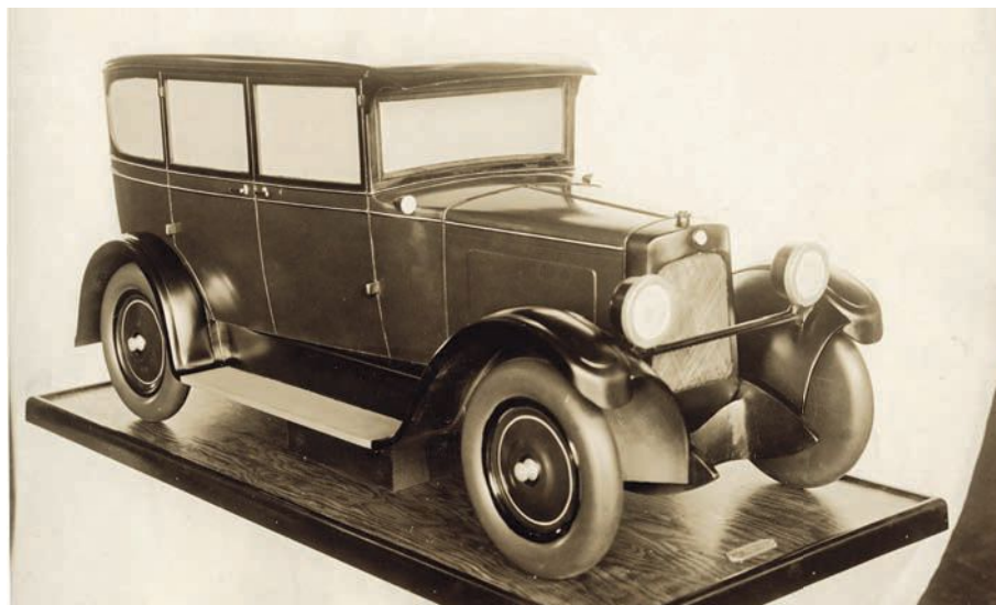
This model had more detail than most, with the addition of cowl lamps, and the front fenders had a more dramatic flair as well. Note the Budd body plate on the base board in front of the radiator and splash apron.
