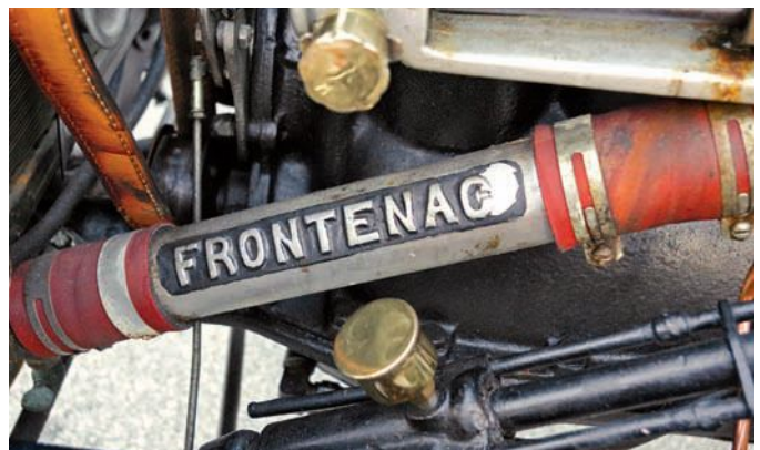
Frontenac-Ford engine boasts doubled horsepower, thanks to plenty of period speed equipment including eight-valve Frontenac R-cylinder head, Winfield S carburetor, finned coil cover and water pump.
