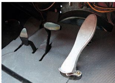
Top: Levers on column control throttle and spark advance. Starter switch has aircraft or marine origins. Right: Four pedals intimidate newcomers. Bottom: Aircraft seats have powder-coated frames and leather upholstery.
