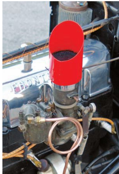
Frontenac-Ford engine boasts doubled horsepower, thanks to plenty of period speed equipment including eight-valve Frontenac R-cylinder head, Winfield S carburetor, finned coil cover and water pump.
