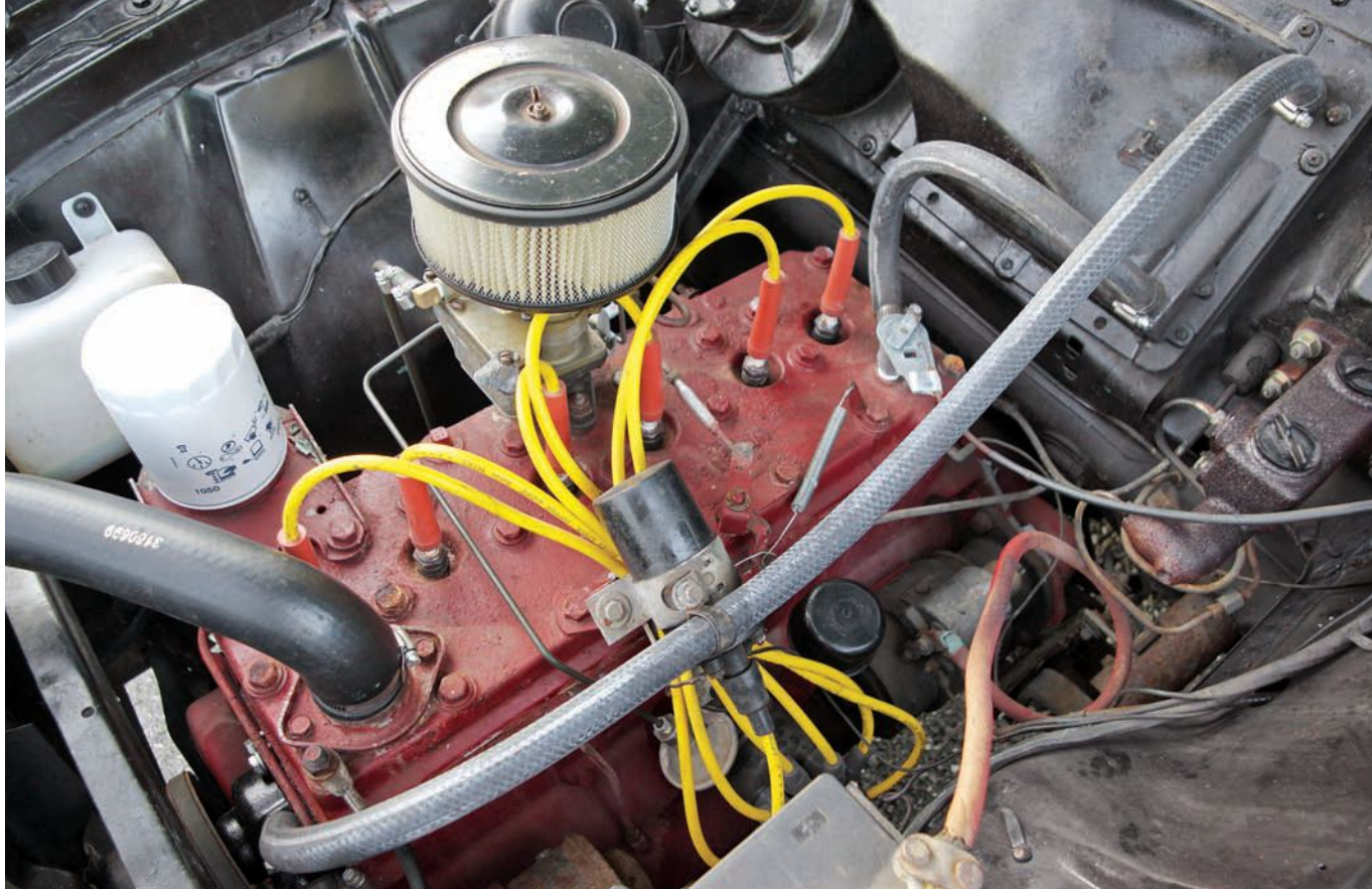
The 1956-cu.in. flathead straight-six engine puts out 90hp and gets 30mpg. Uncluttered engine bay provides easy access to mechanicals.
