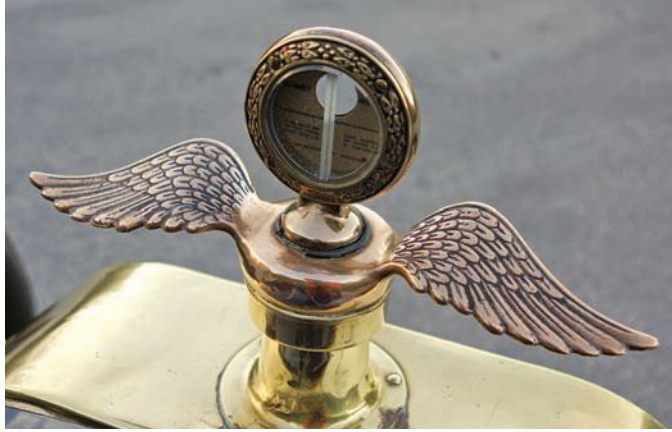
Before reliable gauges, a Moto-Meter was a popular accessory on both stock and modified Fords for monitoring of water temperature.
