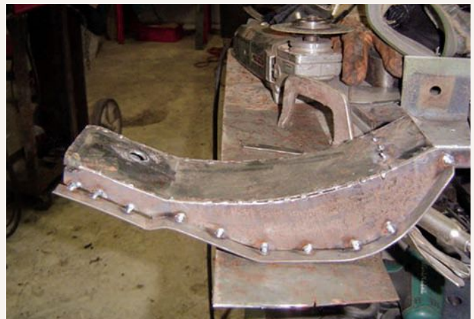
A few of the body mounts were fabricated from templates on a workbench. On the surface, it may seem as though this method could result in less certainty as to proper fit; however, it allowed for far greater control in adjustments and final welds.
