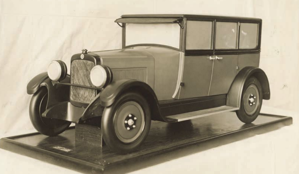
Most of the styling models were made with a generic radiator shell design, but there were exceptions. This particular example has a Hupmobile emblem on the radiator shell and a letter H painted at the center of the hubcaps. The A pillar has the coach lip styling feature at the bottom.
