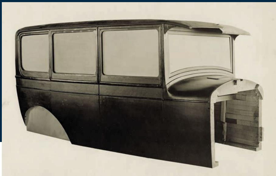
This half-size body model depicts the wood construction as seen looking into the cowl area. Note the two styles of sunvisor split at the center on the same body. Opaque windows were painted a light color to give the impression of glass and were made of heavy card stock or illustration board.
