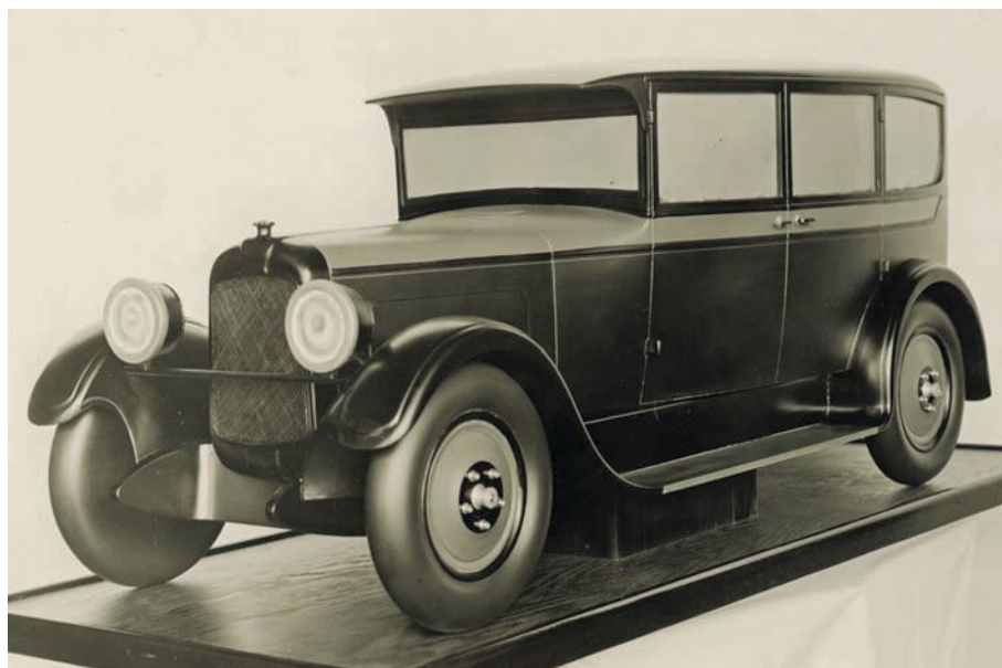
The design of the center top of the radiator shell on this model strongly resembles the one Stutz used on its new "AA" series cars of 1926, although this photograph dates from March 1925. Note the lack of detail on the inside of the front wheel.
