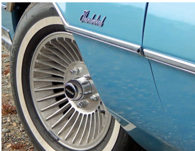
Period-aftermarket Prime 15-inch wheels traded the color-keyed elegance of original wheel covers for a more sporting demeanor.
