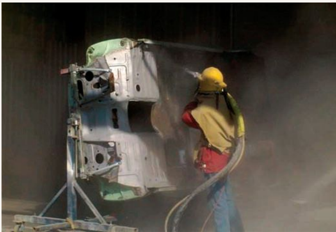
With the body shell secured to a rotisserie, only small sections of the body that were to receive immediate repair work were media blasted. This system of sectional repair work would prevent the rest of the body from being subjected to flash corrosion.
