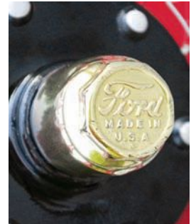
Brass grease cups permit regular lubrication of bearings, which is critical on the modified engine, especially when original Ford roller bearings are retained in service instead of upgraded.
