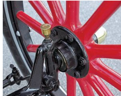
Brass grease cups permit regular lubrication of bearings, which is critical on the modified engine, especially when original Ford roller bearings are retained in service instead of upgraded.
