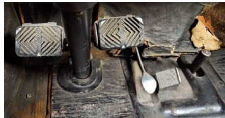
Franklin didn't use "dual-cowl phaeton;" instead, the Pursuit's body style is dubbed a sport touring. Minimal instrumentation includes a roller-type speedometer. The little spoon-shaped lever on the floor is the accelerator. Passenger compartment has never been restored.
