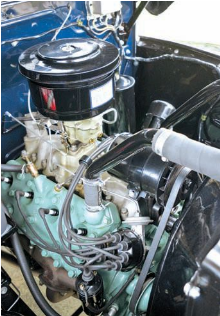
Six-cylinder engines weren't available beneath a Mercury truck hood ornament until 1957. This M-47 is powered by a 239 V-8.
