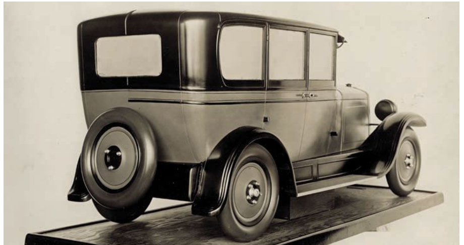
Even the seams where the panels of a real car body were joined together were represented on the scale model, as seen on the rear tub and roof area. Other incredible fine detail points were pinstriping, belt trim, hinges, and valance molding.
