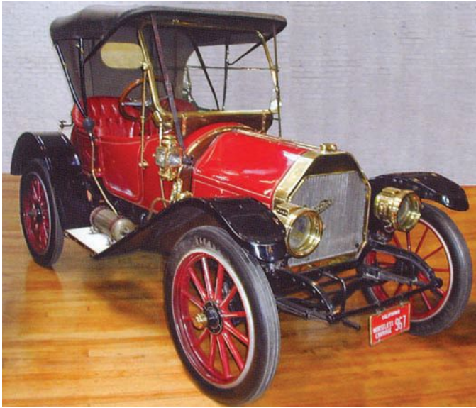
The 1910 Overland Model 38 featured a 25hp four-cylinder engine and two-speed planetary transmission and rode on a 102-inch wheelbase. It could be ordered as a roadster or with a single or double-bucket body, and it cost $1,000—$250 less than the 1909 model.
