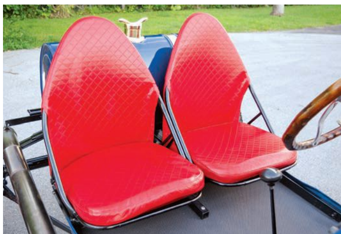
Top: Levers on column control throttle and spark advance. Starter switch has aircraft or marine origins. Right: Four pedals intimidate newcomers. Bottom: Aircraft seats have powder-coated frames and leather upholstery.
