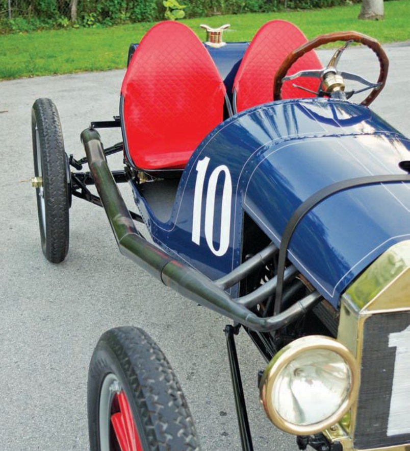
Triple-tube Frontenac exhaust manifold reduces backpressure and gives T engine “that Speedway Roar” sought by speed demons.
