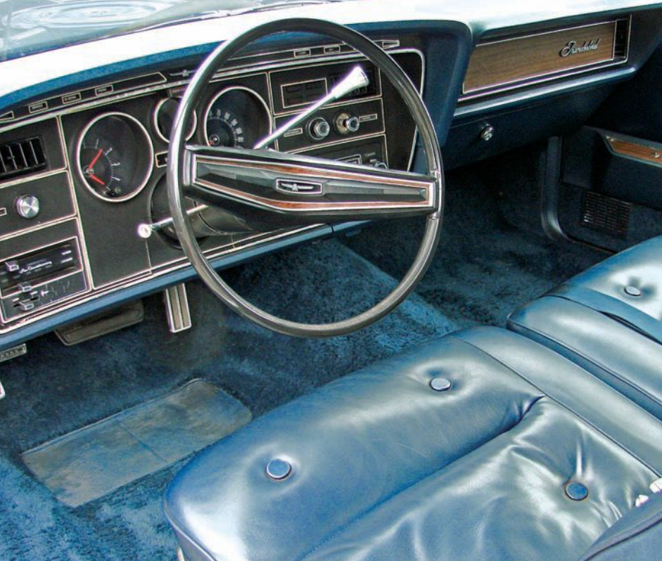
Color-keyed comfort was the name of Thunderbird's game in 1973. A clock and a 120-MPH speedometer are the gauges facing the driver; the AM/FM stereo cassette was an extra-cost option.
