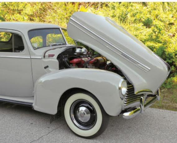
Carefully recessed firewall makes the 1950s 7X 308 look like it was factory installed in 1941. A Dodge Durango radiator hose provides a perfect solution to the early cooling issues caused by the dropped radiator—necessary for hood clearance. Note electric fan.
