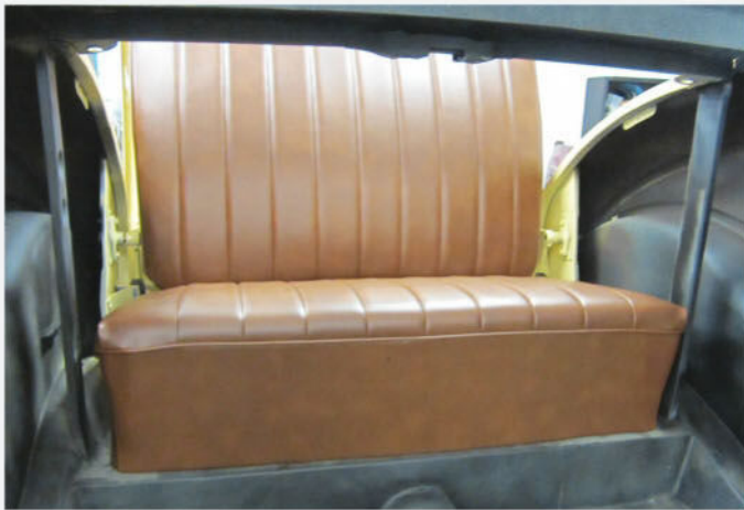
Having been finished several weeks earlier with new leather from a reproduction upholstery kit, the rumble seat has been secured into the Cabriolet with the aid of hard-to-locate hardware that was missing at the time the Ford was purchased.
