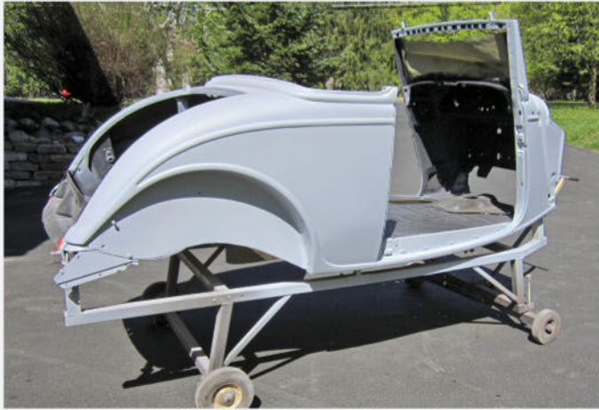
While the chassis was receiving its portion of the restoration effort, the last coat of primer is slowly curing on the Cabriolet body panel. In all, three layers of the Shopline epoxy primer were applied, each sanded smooth with 400-grade paper.
