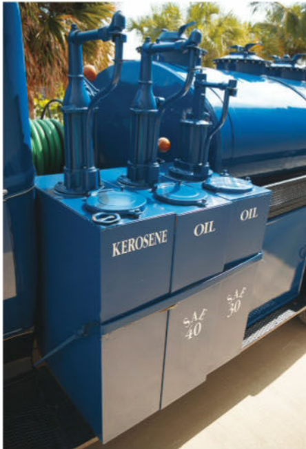
A four-compartment fuel tank made this 1931 Ford Double AA a versatile delivery truck. Additional side-saddle tanks could dispense motor oil or kerosene.
