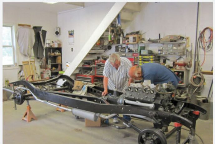
Within a six-month window, the frame and its suspension systems have been refinished in chassis black paint and reunited. In this image, the team is ensuring that the recently rebuilt 261-cu.in. V-8 engine and three-speed manual are properly secured.
