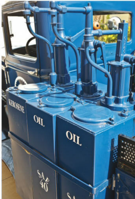
A four-compartment fuel tank made this 1931 Ford Double AA a versatile delivery truck. Additional side-saddle tanks could dispense motor oil or kerosene.
