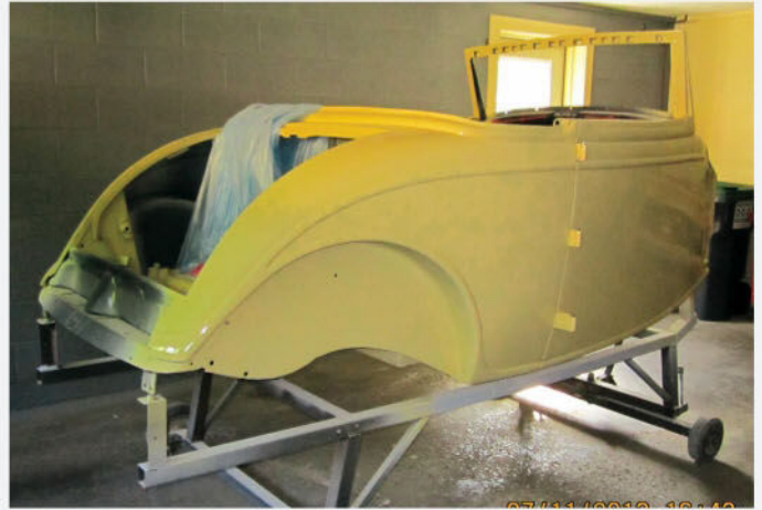
In late summer 2013, the body shell and other removable panels were each given five coats of PPG paint matching the Ford's original Tacoma Cream color. Wet-sanding with 1500-grade paper was one step that would help bring forth a superior shine.
