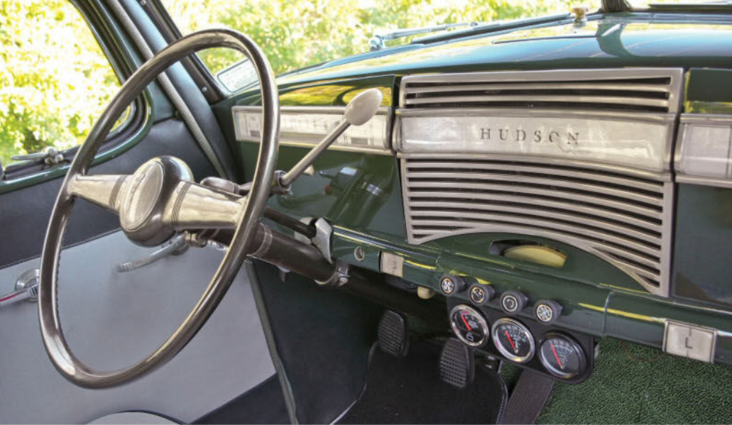
The original interior was well preserved but treated to new carpet and headliner. The column shifter still controls the Traveler's original three-speed transmission. Cavernous trunk swallows a salesman's samples, a couple's luggage or chairs and cooler for shows.
