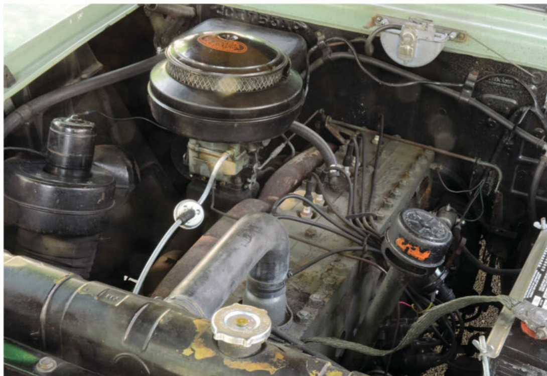
The 327-cu.in., L-head "Thunderbolt Eight" in the Deluxe Clipper made 160 horsepower with its two-barrel carburetor; senior Packards got four barrels and 20 more horses. Lacking a V-8, Packard boasted about the 8.0:1 compression ratio of its engine.
