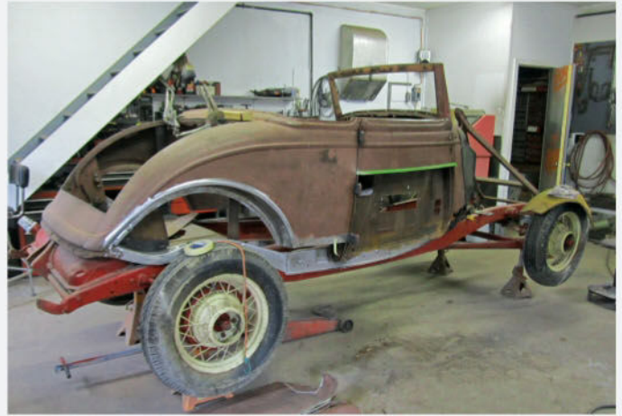
As the body was slowly receiving its corrective measures, the frame was finally delivered to the shop. Still wearing its red paint from the initial restoration attempt, the body is temporarily reunited to the frame to help facilitate the repairs.
