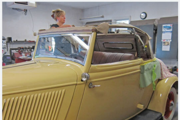
With the fresh paint carefully protected in some areas, Diana is in the process of installing the new Cabriolet top to the refinished bows. The original top kit was incorrect, but skill, diligence and careful coordination resulted in a new kit.
