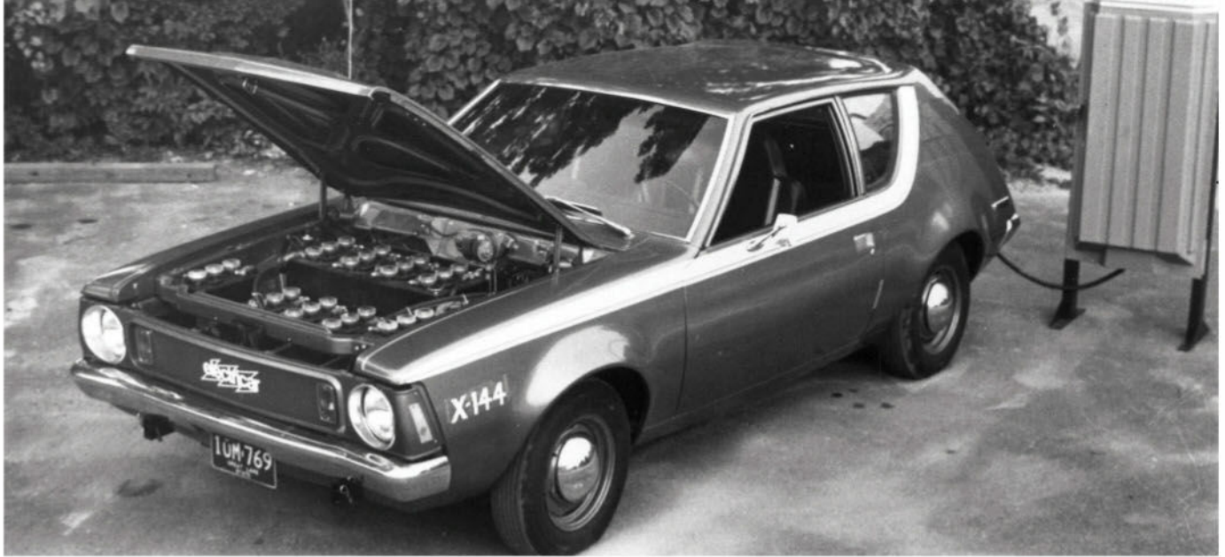
The 1973 X-144 Electricar by EFP was a two-door sedan built on a Gremlin chassis. Priced at $3,450, it had a range of 60-75 miles per charge. A top speed of 60 MPH was claimed.
