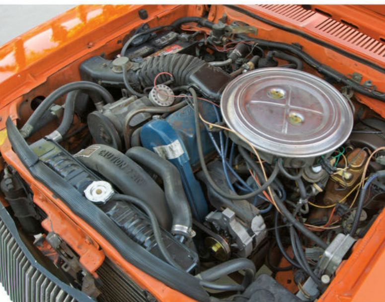
Ford's 2.3-liter four-cylinder engine had been under the hood since 1974, and was the go-to engine in the gas-crisis year of 1979.
