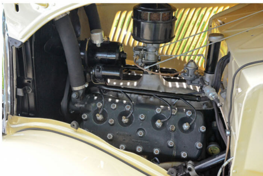
Powering the Cabriolet is the Ford’s original 261-cubic-inch 21-bolt “flathead” V-8 engine, which has been carefully restored to original equipment specifications.
