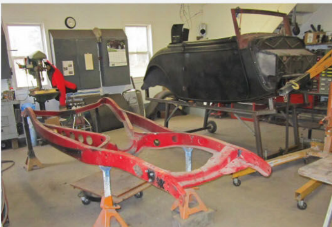
By December 2012, the Cabriolet's body repairs have been completed and sealed in a protective coat of self-etching primer. Note that the body has been re-secured to the jig, and the Ford's original frame has been disassembled and made ready for media blasting.
