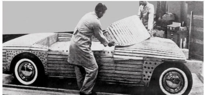
Early clay model shows original front end, with floating front bumper. Design studio staff bucked the model onto a lightweight wood frame after initial full-size drawings were approved by management. This was close to the actual production version.
