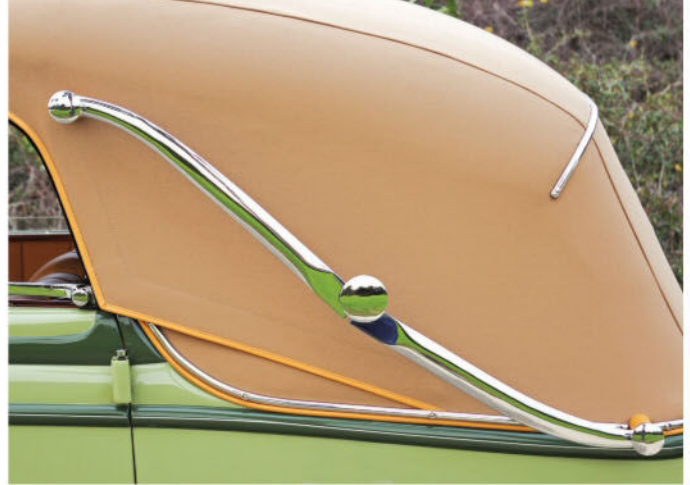
The insulated top has a spring-loaded mechanism that locks it down and helps raise it partway. Note the inscribed sill plate.
