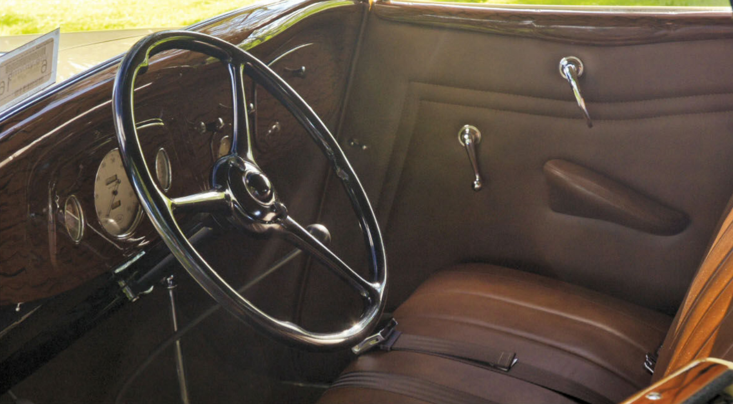
The woodgrain instrument panel, gauges and steering wheel, were restored onsite; plated door and window cranks were merely polished.
