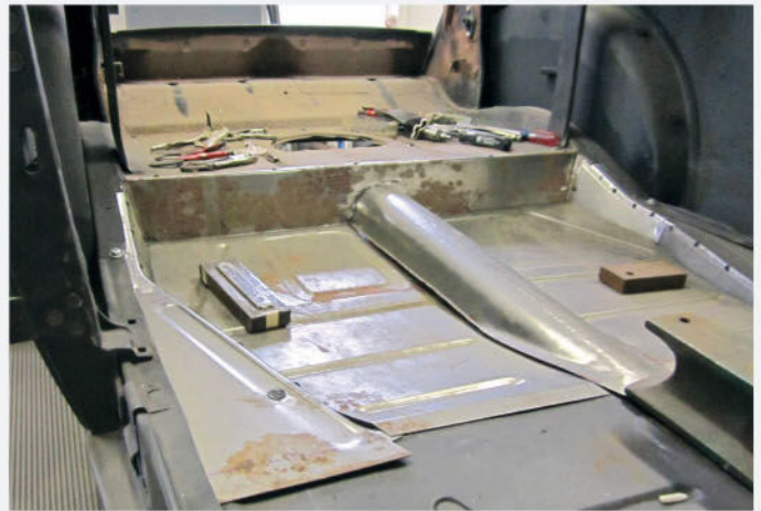
With nearly all the exterior body repairs completed, the restoration effort turned to the floorboards. The original metal had been all but destroyed by moisture, forcing replacement sections to be fabricated using the originals as a pattern.
