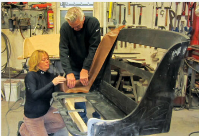
Having earlier fabricated the front seat's main frame from wood, restorer Cliff is assisting his daughter, Diana, with the upholstery phase of the restoration. Properly stretching and securing the new leather is an exercise in extreme patience.
