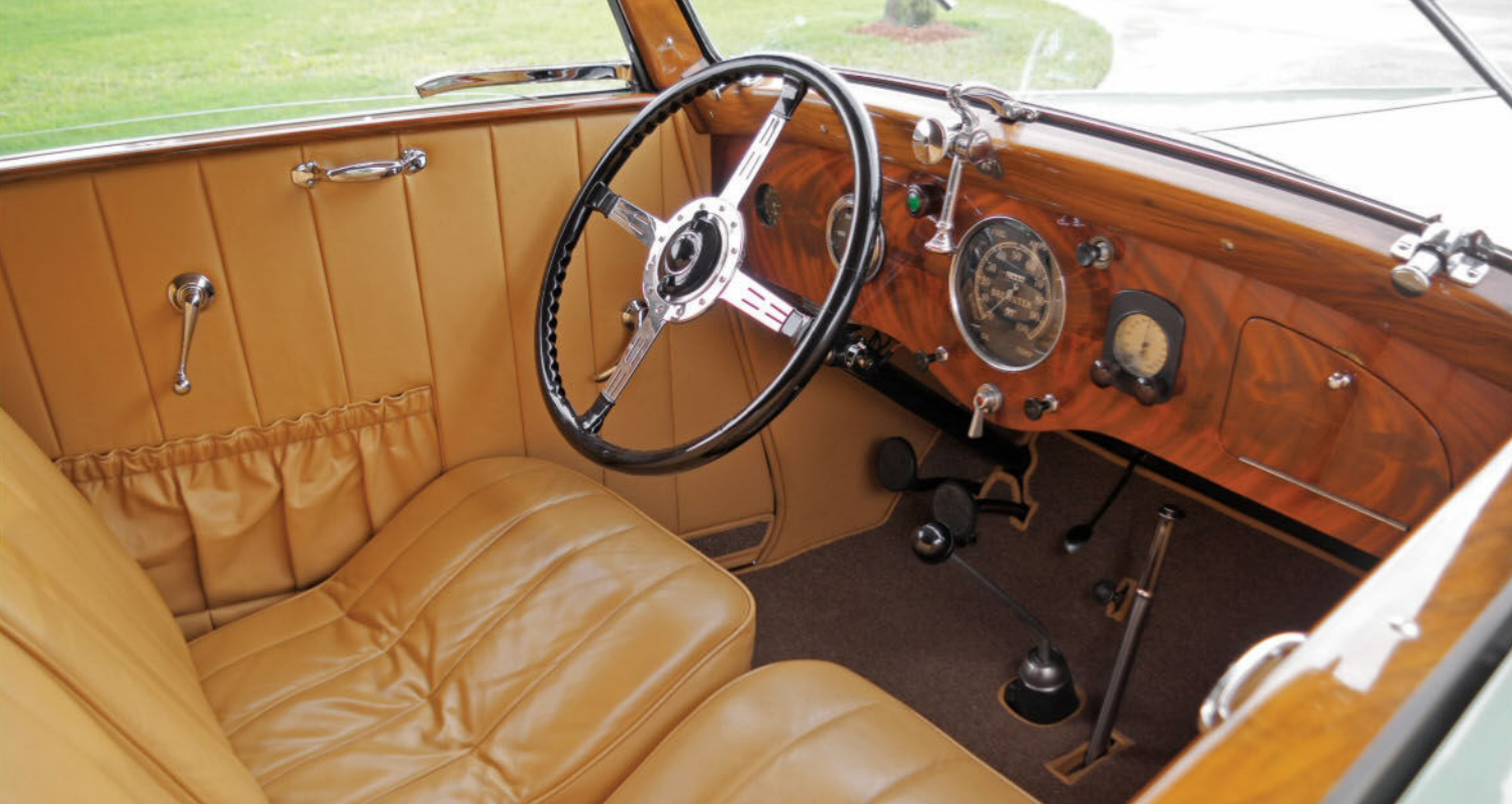
Unlike production U.S. open-top Fords, this custom Luxus has a hinged, venting windshield with trafficators built into the frame.
