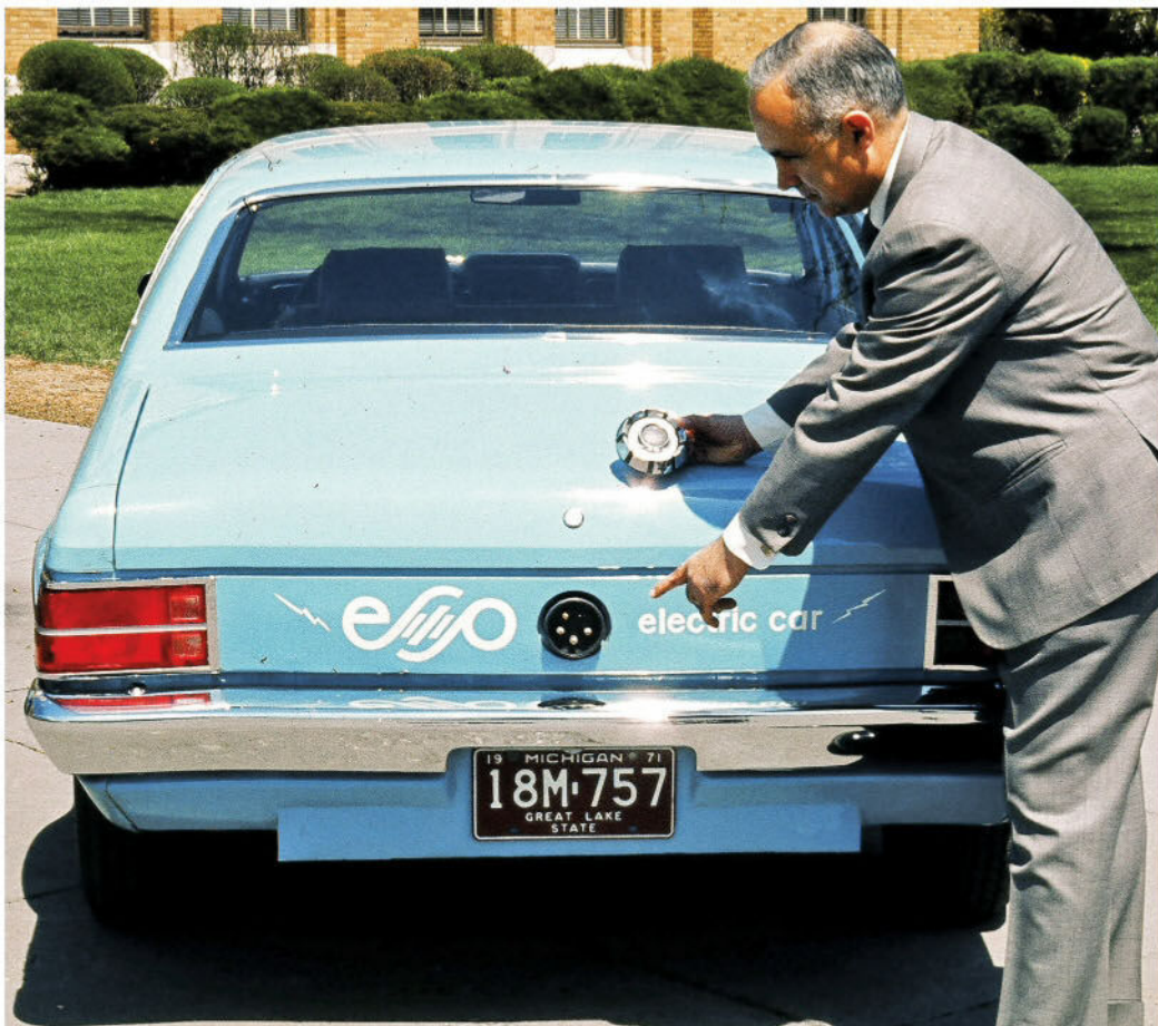
The gas cap conceals the plug-in for recharging the battery pack.
