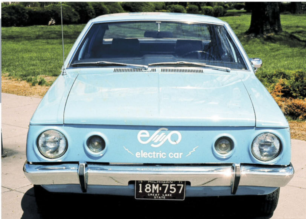
Exterior modifications to the EFP Hornet were minor. Grille fascia was unique, as were nameplates on front fenders.
