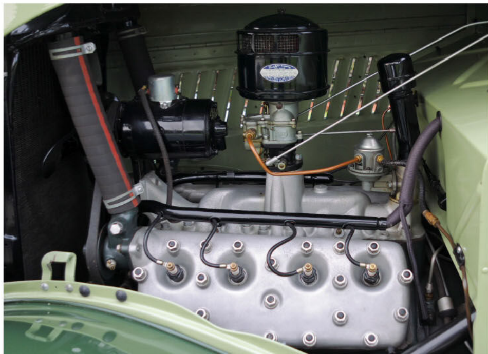
The Cologne, Germany-built body was placed on a standard Model 40 chassis when it arrived in Michigan in August 1934, so its 85hp V-8 engine is stock.
