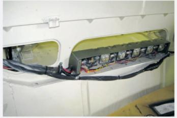
Located behind the rear seat is the primary bank of 12-volt starter relays required to manipulate the folding hardtop. The process of restoring the wiring was tedious, as each unit had to be properly linked to circuit breakers and limit switches.
