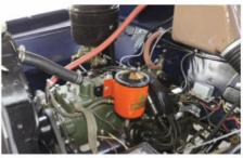
An accessory Fram oil filter is a wise periodcorrect accessory. Out back, the Caravan Top kept cargo covered and dry.
