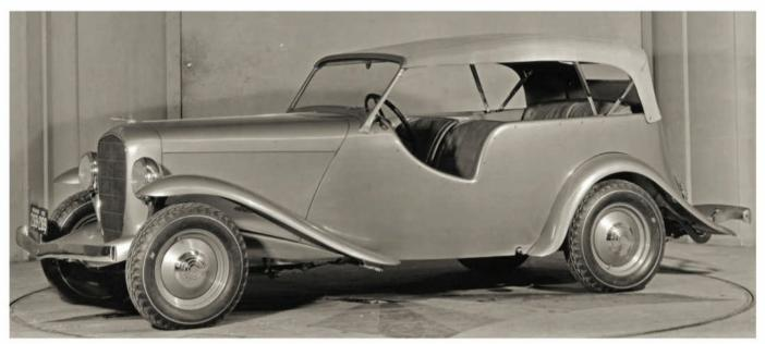
Frank Spring designed this low-cut and sleekly styled 2+2 sports car on a 1932 Terraplane chassis. Note the soft, flowing lines, the raked windshield, and lack of running boards. Unfortunately, the company chose to not put it into production, so this car remained a one-off prototype.
