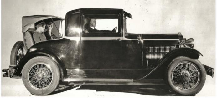
In 1929, Hudson's designers came up with a neat, though rarely seen, option for rumble seat coupes and roadsters. Called the "Rumble-Roof," it provided passengers in the rumble seat with a degree of protection from the elements.
