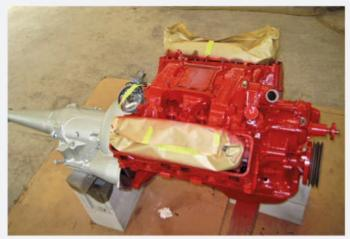
A previous owner's refurbishment effort had the 312-cu.in. V-8 engine and Ford-O-Matic two-speed automatic transmission already rebuilt. After careful inspection, all that was required for this restoration was a simple cleaning and proper repaint.
