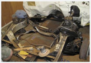
A decision to not remove the body from the frame turned out to be a hindrance, as the second phase of the project jumped into high gear. So as not to damage the new paint, the chassis had to be carefully stripped by hand or with small pneumatic hand tools.
