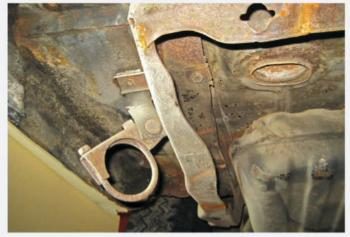
Few photos of the Skyliner's restoration were taken because of the original intention to merely make a good "driver"; however, this one illustrates the overall condition of the chassis in the early stages of disassembly. Only a few patch panels were found and no rot.
