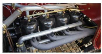
Making power on every downward piston stroke with far fewer parts, two-cycle engines are inherently more efficient. But they require some unique engineering. In the case of Elmore's 254.4-cu.in. inline-four, the crankcase (below) requires a separate, sealed chamber for each cylinder.
