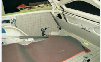
A foam pad—specifically, the material used to hide the bulk of the electric top wiring and corresponding mechanisms, some of which can still be seen—is used to protect the surface of the Ford's rear compartment as finish work progresses.
