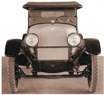
This 1921 experimental car, which looks to be a seven-passenger touring model, demonstrates some of the methods used in styling early Hudsons. From the side, it appears to be a fully-functioning automobile, but a look at the front reveals the radiator is a fake, used to gauge its appearance on the car. The fake radiator would have been made of either wood or plaster.
