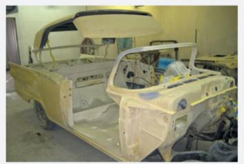
At this stage, after small repairs had been made to the quarter panels, the main body shell was sprayed in a layer of self-etching primer and Rage Gold body filler. A keen eye will note that the interior has already been repainted in Colonial White.
