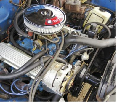
Fitting a chrome air cleaner was a popular period "upgrade" to the V-6, as owners hunted for every ounce of extra horsepower. With its two-barrel Holley carb, it made just 105 horsepower.
