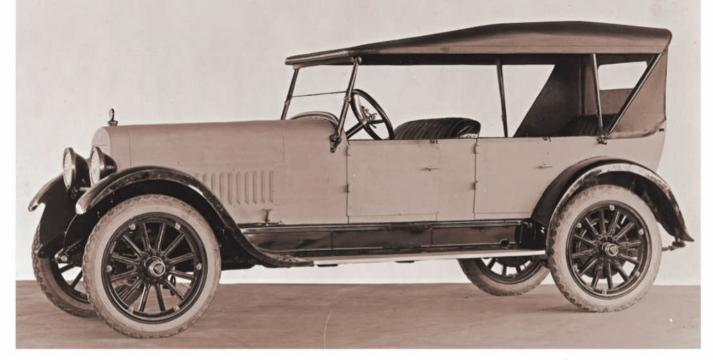
Hudson engineers continued to experiment with new ideas, such as the long-wheelbase touring car pictured here, which is a special engineering mock-up that didn't reach production. In 1924, they rebuilt the experimental 1919 Essex Speedster with modified styling, and a new name, "Essex Raceabout" (pictured below). It was purchased by Hudson cofounder Roscoe Jackson.
