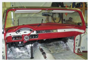
Final reassembly is progressing in the passenger compartment with the installation of the instrument panel and associated trim. Sun visors are in place, and both doors have already been hung and balanced. Also visible is the restored forward-hinged hood.
