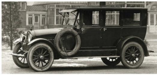
In 1920, Hudson built this experimental model with body styling features that never made it into production, including the sloped hood and unusual windshield. Note, too, the unusual forward-placed roof rack.
