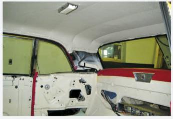
As with most restorations, interior upholstery is installed using the top-down system. Headliners, in the case of a retractable hardtop, are a little more complex at the forward edge. Seats and door panels were quick to follow.
