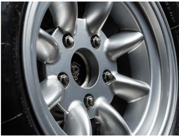
Above left: 9Jx15 Minilite wheels are used at the rear as Fuchs couldn't supply a wheel of sufficient width at that time
