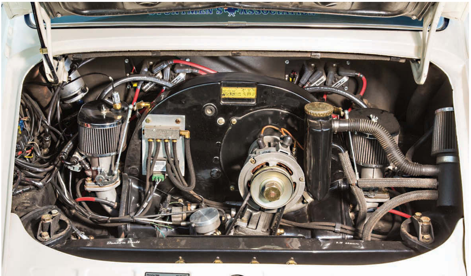
Above: Busy engine bay is home to a fuel-injected 1.7-litre 'four' running twin-spark ignition with crank-trigger and coil packs
