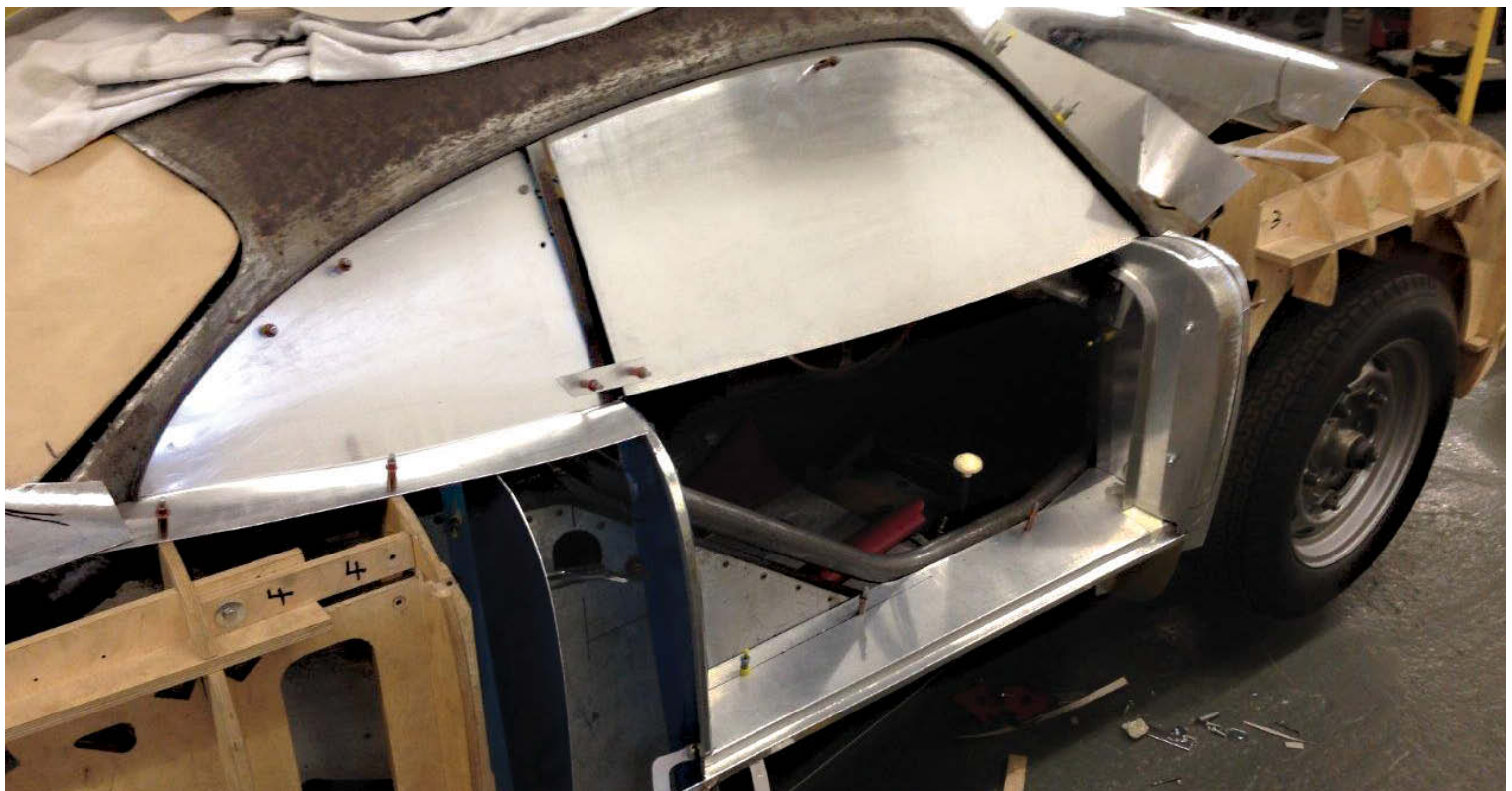
Below: Aluminium templates have been made for the windows to make it easier to cut the Plexiglas to the exact shape and formed to the correct contours
