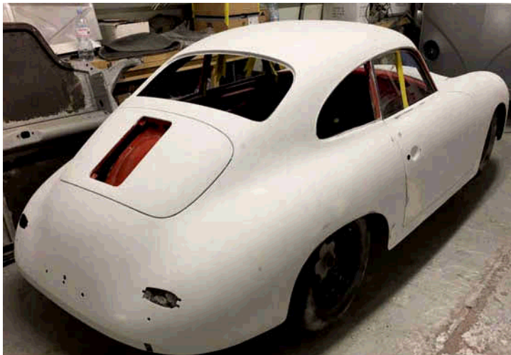
Below left and right: Once the bodywork had been fettled (the only repairs needed were to the doors and sill), it was time for the high-build primer and first hand-flatted colour coats
