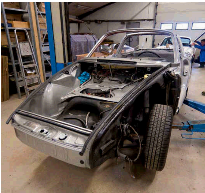
Below right: Aluminium engine lid and replacement quarter panels fitted to a new JP project
