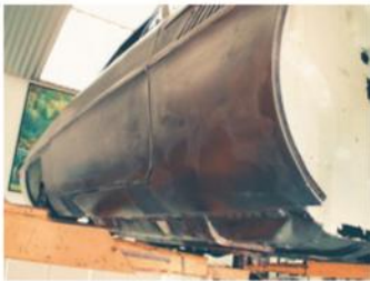
As part of the Cosmo's complete restoration, its body was dip-stripped then mounted on a rotisserie for painting
