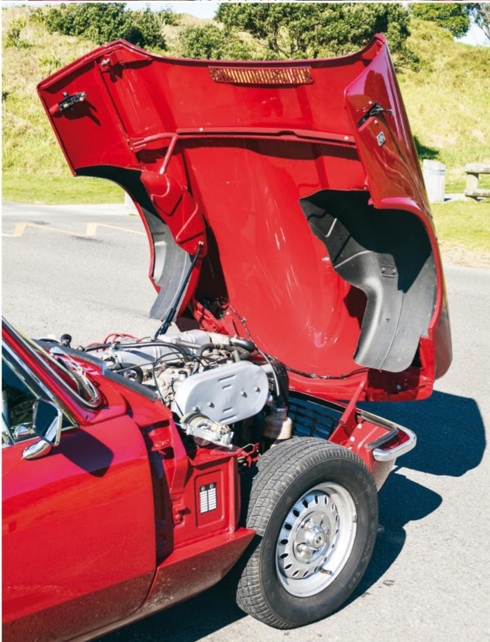
Like the Triumph Herald and Spitfire, the GT6 enjoyed easy engine access
