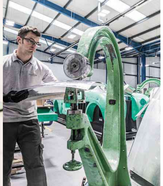
Below, from left Body design begins with a CAD program before moving on to computerised milling; scale model is of Eadon Green Black Cullin; Matt Godsell at work with the English wheel.
