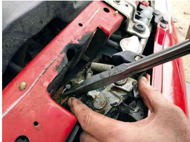
Clockwise from above Disengaging the bonnet release cable so the Insight's latch mechanism could be adjusted; Derek Magrath makes an 80-year mental leap from the 1920s Amilcar engine on his bench; Insight was always engaging and enjoyable to drive.
