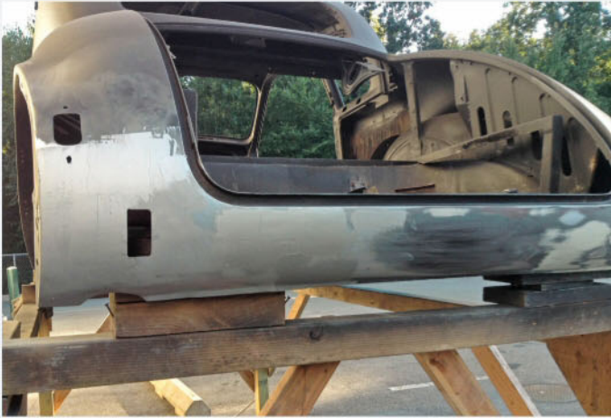
After the patch panels had been welded into place and the joints ground smooth, a skim coat of Evercoat Rage body filler was applied. Using three different grades of paper, the area was then sanded, providing a smooth surface for the next stage.
