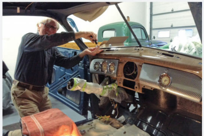
A significant portion of the Buick's final reassembly needed to be completed; however, one of the first critical steps was the installation of the instrument panel as a nearly completed sub-assembly. Note the steering column is carefully wrapped.
