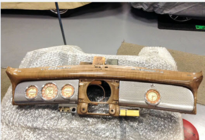
Several smaller projects were underway while the chassis and body were being restored. This included the Buick's instrument panel. Note that at this point new woodgraining had been done, along with the engine-turned applique and rebuilt gauges.
