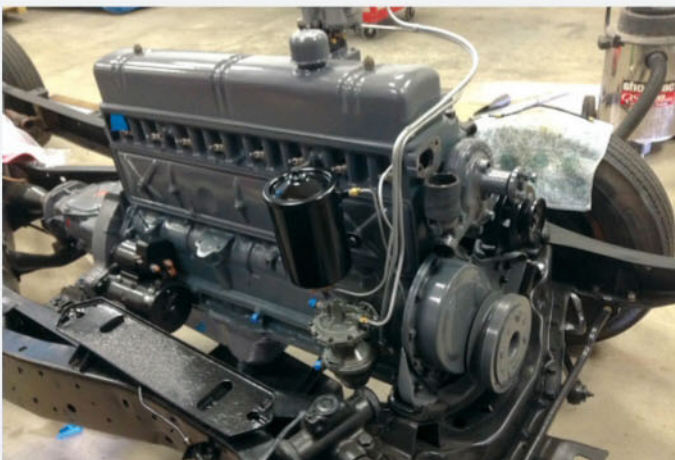
The Buick's original 248-cu.in. straight-eight engine has been bolted to the chassis at this stage; rebuilt and repainted a proper shade of gray. A keen eye will also note that the fully synchronized three-speed manual transmission has been installed.
