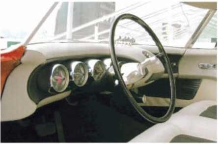
Interior view of the Mercury D-528 for 1955 shows a modern wrap-around instrument panel, power window switches, and two-spoke steering wheel.
