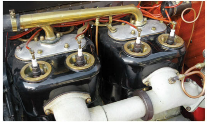
Cross-flow flathead design is called a T-head and utilizes dual camshafts to actuate valves on either side of the cylinders. The big four-cylinder is a derivative of the six-cylinder engine used in the Limited series. Fed by a large, brass Rayfield carburetor, the Autocrat's engine puts power to a four-speed.
