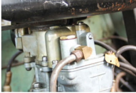
600-series models were powered by an 82-hp, 172.6-cu.in. L-head straight-six fed by a single-barrel Carter carburetor, while upmarket Ambassadors used an OHV straight-six engine.
