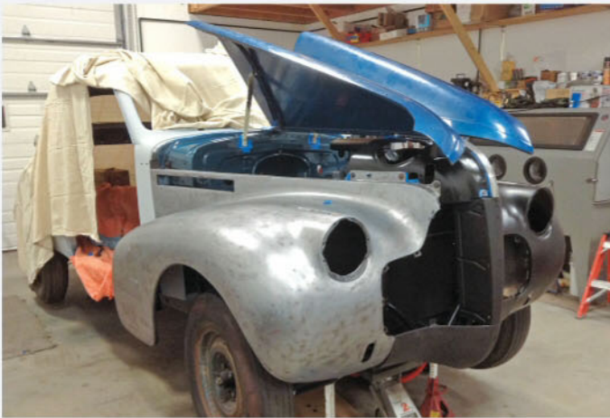
Prior to the rest of the body being painted, it and the other removed panels were test-fit both to the chassis and each other. Final adjustments were easier to plan and/or accomplish at this stage without risk of marring new paint, save for the firewall.
