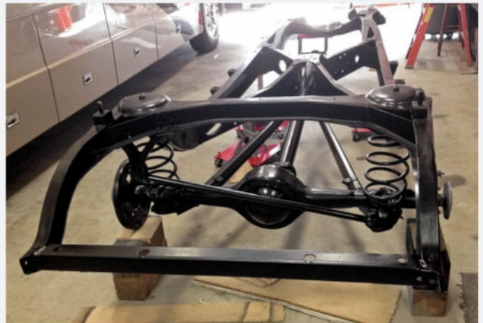
Part of Buick's "Full Float" ride is on display in the image during the chassis' reassembly, which featured, in part, coil springs and lever-action shocks. The rebuilt differential and torque tube assembly were also installed.
