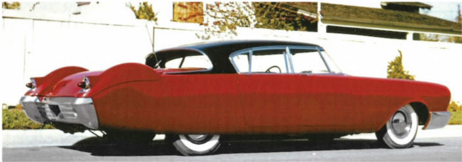
Side view of the Mercury D-528 shows off the unusual rear "fins," though "humps" might be a better descriptor. The reverse angle C-pillar and enclosed rear wheels give this car a distinct Nash flavor.
