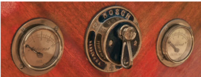
Pump between seats allows driver to pressurize fuel system before starting. Gauges include oil pressure, fuel, and Jones speedo. Switches reveal Bosch dual-coil ignition. Gated shifter for four-speed trans is located to driver's right.
