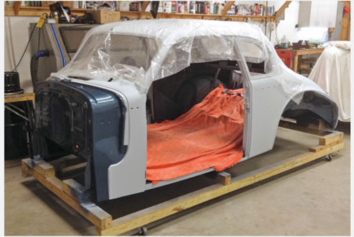
The Buick's main body shell once all the body prep had been completed. You'll note that while the outer surface is exhibiting two coats of epoxy primer, the firewall—and portions of the interior—have been finished in Bandelier Blue paint.
