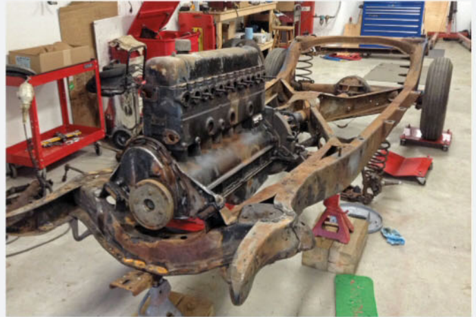
The Buick's second disassembly began immediately upon its arrival. After the body had been placed on a homemade wooden dolly, all attention was focused on the 121-inch wheelbase chassis, which was systematically stripped to a bare frame.
