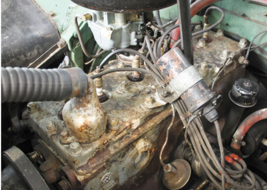
600-series models were powered by an 82-hp, 172.6-cu.in. L-head straight-six fed by a single-barrel Carter carburetor, while upmarket Ambassadors used an OHV straight-six engine.
