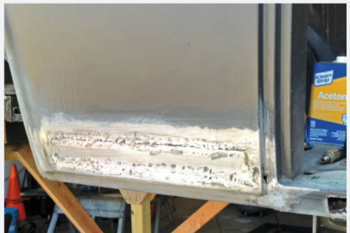
Here is one example of the fabrication work required to correct corrosion uncovered while the body was stripped of paint. This area is located behind the passenger door. The patch panel was created from 18-gauge steel and MIG welded into place.
