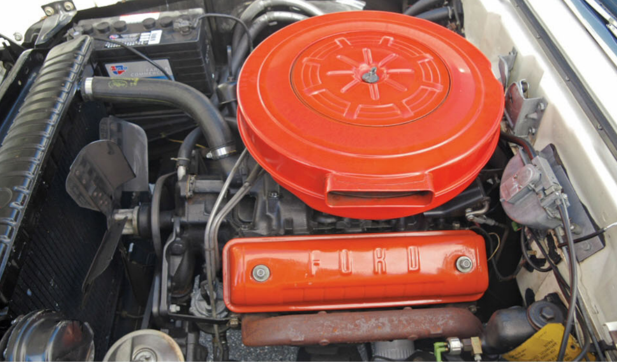
The 292-cu.in. engine appears to be virtually untouched since its installation, and even some original hoses and belts remain. A few hose clamps were replaced with a newer design.
