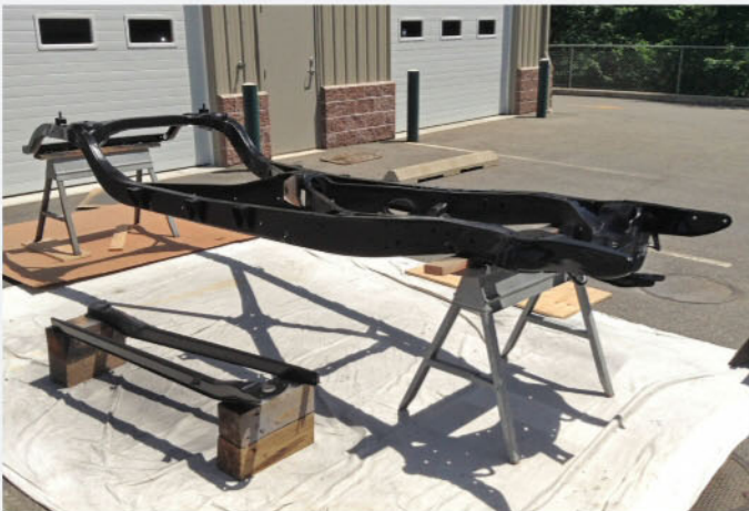
Pictured here is the Buick's frame after being stripped of equipment and sandblasted. With no damage to contend with, it was sealed in primer and finally painted in chassis black paint. All of the work was performed at the owner's shop.
