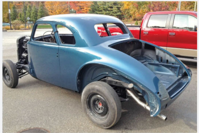
The business coupe has just been delivered after receiving the rest of the paint process. A basecoat/clearcoat system was used, consisting of three coats of each. After curing, it was wet sanded and buffed, followed by final polishing.
