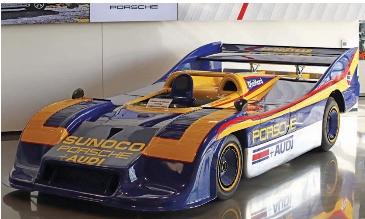
Left: Mark Donohue successfully raced the Can-Am 917/30, running a 1200+bhp 5.4-litre flat-12
