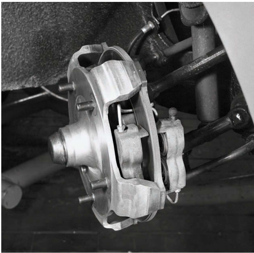
Above left and right: Porsche's own annular disc brake (the caliper is mounted inside the disc) was effective but ultimately doomed to failure as it could only be used with wheels using the 'wide-five' bolt pattern
