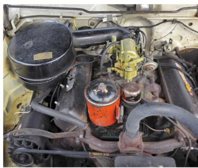
Debuting in 1951 at 232-cu.in., the rugged Studebaker V-8, with its forged crankshaft, generous bearing surfaces, solid lifters, and other tough components, displaces 259 cubic inches in the 1956 Parkview.
