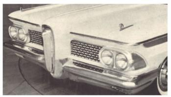
Rejected 1959 design looks almost too much like current Pontiac to believe. Edsel brass rejected exposed nose because of vulnerability.
