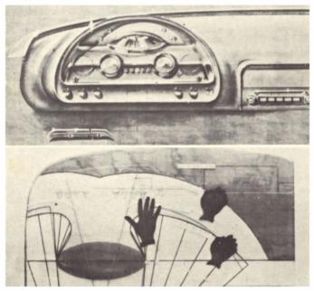
Edsel was to get pushbuttons on the dashboard, behind steering wheel. Studies showed this would be awkward, so the designers moved buttons to steering hub. Dome speedo was retained.
