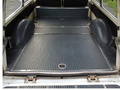
The two-door, six-passenger Studebaker wagons of 1956 featured a long cargo area with the rear seats folded down. And the split tailgate allows you to open the window separate from the drop-down door.
