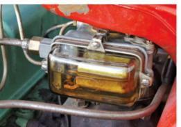
Specifying the 145-hp, 223-cu.in. six-cylinder earned the buyer a \$83.70 credit and got an engine identical to standard Fords. Glass-bowl Holley carb and "mustardtop" coil are characteristic of the Ford six-cylinder.
