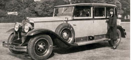
1929 Cadillac limousine-cabriolet by Letourneur & Marchand. The roof over the chauffeur could be opened up, and the car is on a lengthened chassis.
