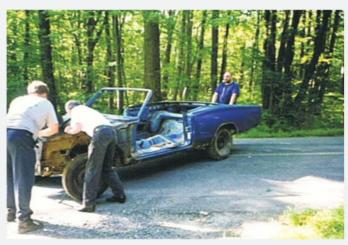
Flash forward to summer 2002. Having been in garage storage since the winter of 1979-'80, the convertible's restoration has finally begun. Except for the suspension and differential, the unit-body Dodge has been completely disassembled.
