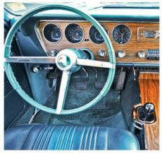
The interior is original, and the woodgrain dash appliqué was included when the console was ordered. A lever under the dash is for a windshield-washer hand pump (since removed) that was added when the stock pump expired.
