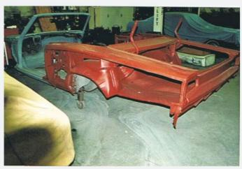
The restoration was put on hold until Wayne could find a facility capable of managing the rest of the effort could be found. In 2004 it resumed, and here the vertical flanks of the rear quarter panels have been removed, as well as one part of the trunk floor.
