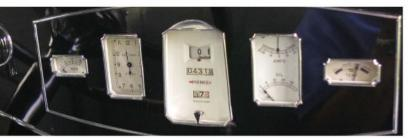
The instrument panel's gauge bezels would be replated. Note how the central speedometer unit echoes the radiator's shape.
