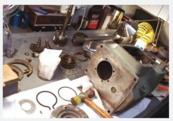
Like the engine, the Coronet's original four-speed manual transmission, fitted with a Hurst shifter on the assembly line, was disassembled and rebuilt. With no wear to speak of, it only required new seals and bearings.
