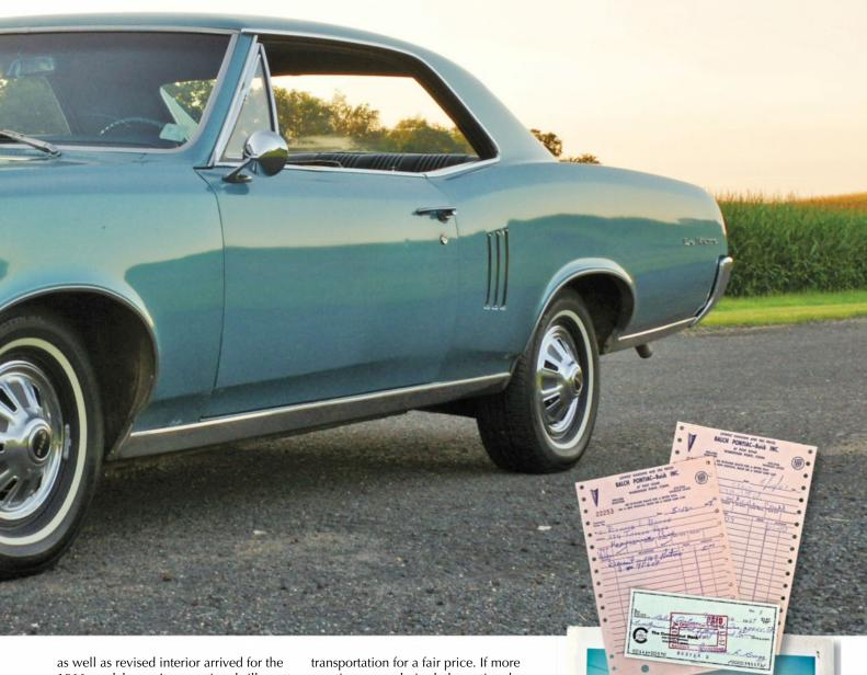
as well as revised interior arrived for the 1966 model year. Its sensational silhouette was carried over for 1967, which also featured a restyled grille and taillamps, as well as simulated louvers on the quarter panels—a Le Mans two-door exclusive. New upholstery patterns and scads of standard safety equipment, including an energy-absorbing steering column, dual-circuit master-cylinder brake system, fourway hazard warning flasher, and much more also set the 1967 models apart.
