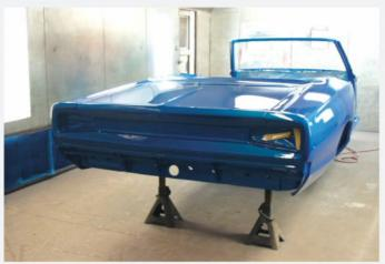
Earlier, the body received a few coats of Glasurit primer that were sanded smooth for the next stage of the restoration seen here: the application of a Glasurit basecoat/clearcoat perfectly, matched to the factory hue of Bright Blue metallic.
