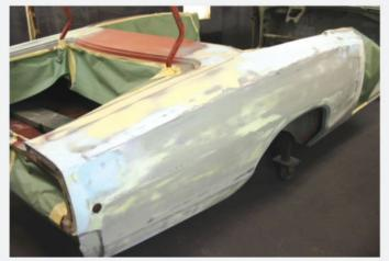
Vertical flanks from reproduction coupe quarter panels have been butt-welded into place. Welds were then ground smooth, and the metal was sealed in a layer of epoxy primer. Here a skim coat of filler has been applied and block-sanded smooth.
