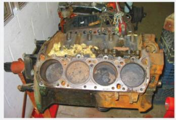
During downtime between stages of body repair, other aspects of the restoration were accomplished, such as rebuilding the Mopar's 330-hp, 383-cu.in. V-8 engine. During disassembly, a massive mouse nest was discovered in the lifter valley.
