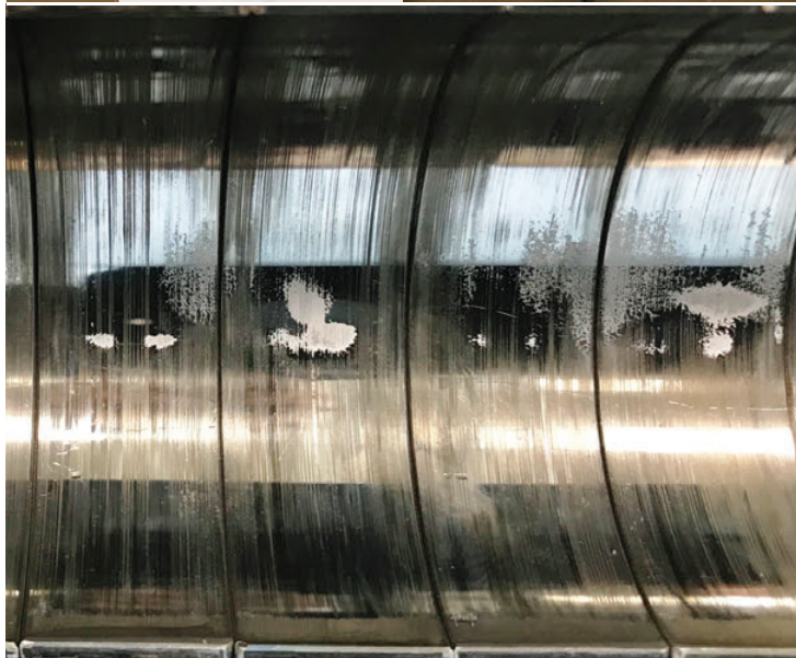
ABOVE & BELOW Used rod bearings illustrating overlay fatigue and, below, cavitation
