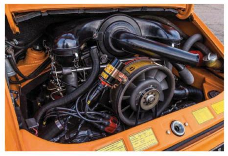
Above left: 180bhp 2.2-litre engine features mechanical fuel-injection, a definite improvement over the older model's carburettors
