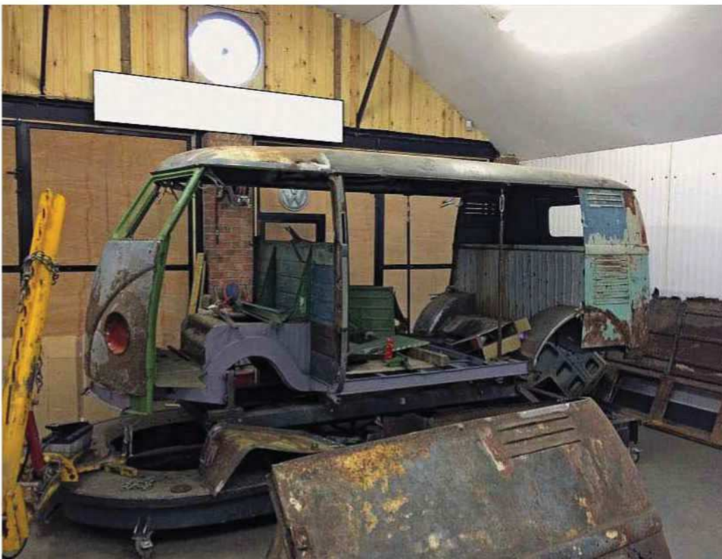
Anti-clockwise from top right These cabin parts were deemed salvageable; rear torsion tube housing was re-used; section from rear of roof (here on left) was patched into corroded front part; bodyshell part-way through the rebuild; underside was fully painted for future durability. →
