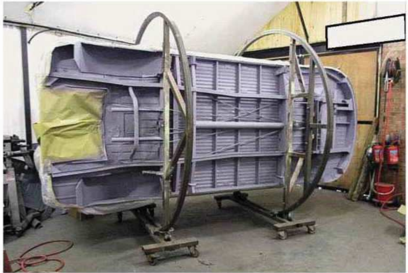
Anti-clockwise from top right These cabin parts were deemed salvageable; rear torsion tube housing was re-used; section from rear of roof (here on left) was patched into corroded front part; bodyshell part-way through the rebuild; underside was fully painted for future durability. →
