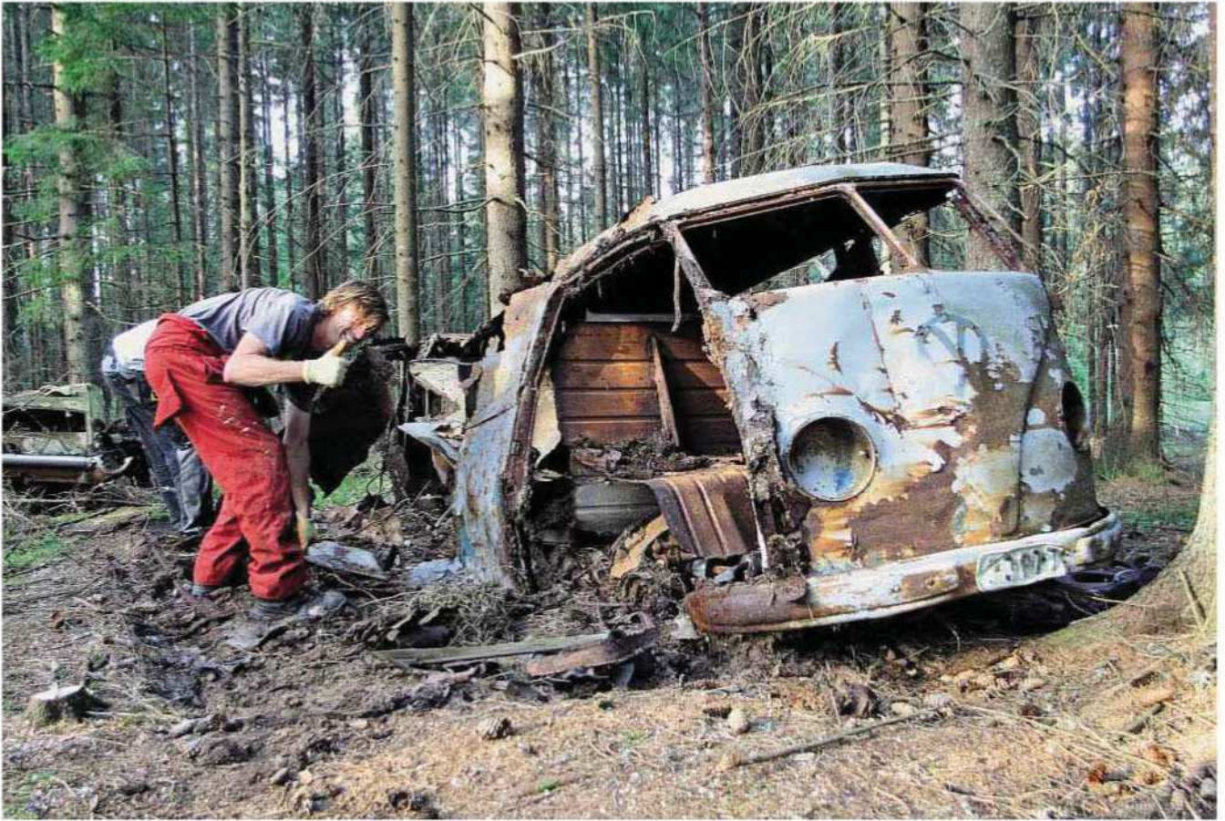
Above, left and below Bus shell was too fragile to be moved in one piece, so was cut up with an angle grinder and stacked on a trailer.
