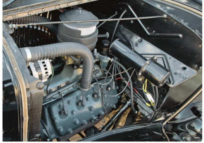
A "21-stud" 1937-vintage V-8 stands in for the original engine in this '35. A one-wire 6-volt alternator keeps the headlamps glowing.
