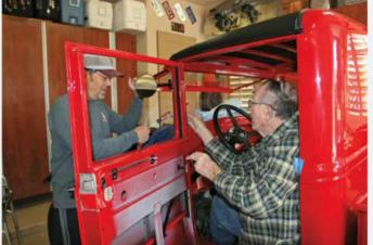
Kevin's dad, Paul, continued to help with parts of the restoration when possible. Proving that an extra set of hands can be handy, here they are carefully installing the windshield, which is hinged on the top corners to help ventilate the cab.
