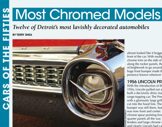
t the beginning of the 1950s, dowdy and conservative were giving way to adventurousness and daring. With the technical processes of chrome plating all worked out by the 1950s, and with chrome both brighter and lower maintenance than the previous nickel-plated finishes, designers could fully embrace chrome plating, and that they did! Automotive stylists seemingly couldn't get enough of it. If a little was good, more was better, and too much was just about right.
