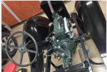
After panel fit was tested, final adjustments were performed, which culminated with the last coat of primer and wet sanding. Once the primer had cured, the fenders were finished in several coats of gloss black enamel, and installed on the chassis soon after.
