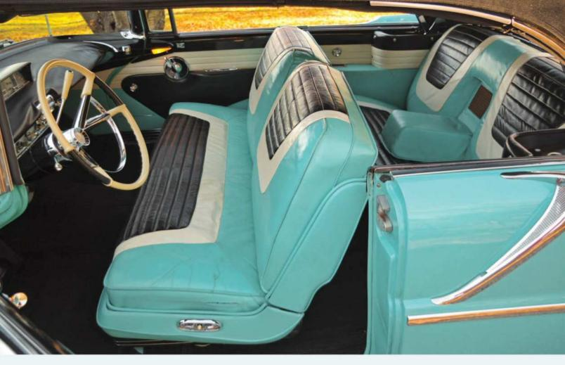
Optional "3-tone" leather trim interior is original. The extra-cost Travel-Tuner radio features "Town" and "Country" selector bars, and came with front and rear speakers, a power antenna, and a foot switch to change the stations when the driver would rather not reach for the radio buttons. Power windows were standard in the Premiere.
