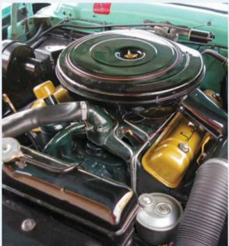
According to this Premiere's owner of 36 years, the original 300-hp 368-cu.in. V-8 engine has yet to require any major work, aside from detailing.
