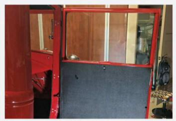
Like the aforementioned roof insert, all new interior upholstery was purchased from LeBaron Bonney. Their packaging included ready-toinstall kits for the bench seat, as well as both door panels, the latter of which is seen here, already screwed into place.
