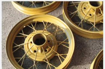
After having the Ford's original wheels cleaned and powder coated, Kevin was advised to have them checked for irregularities and enlarged stud holes. Ultimately, new wheels were obtained, media blasted, trued, and powder coated in gloss Cream.
