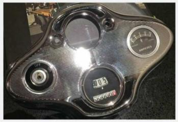
Earlier, several pieces of trim were replated, while others were polished to a factory-new shine, including this simple-yet-detailed instrument bezel. The bezel was repopulated with restored gauges; it would then be installed in the cab as a sub-assembly.
