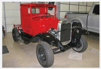
The cab, properly aligned to the frame, is bolted into place, while a few components have been secured to the firewall. Note that, in addition to the fenders, the running boards and headlamp bar are installed; the steel wheels are temporary.
