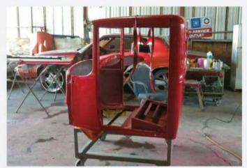
The Ford cab has just emerged from the paint booth after receiving a few coats of DuPont enamel paint matched to Vermillion Red, a hue original to the 1931 Ford color spectrum. The cowl and hood were also painted the same color at that time.
