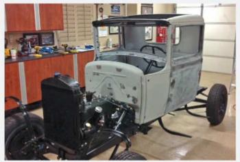
At the conclusion of Part I of this story, the body had been returned to Kevin in primer. It was then partially reassembled on top of the restored chassis. The test-fit enabled the team to check tolerances and alignment, and make corrections prior to paint.
