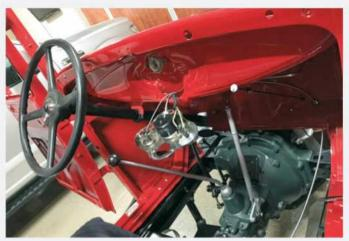
Reassembly has commenced in earnest with the fitting of the cowl/ fuel tank with its integral fuel gauge, the latter slotting into the open position on the instrument panel. A new wiring harness was obtained earlier. Note that the doors have been hung.
