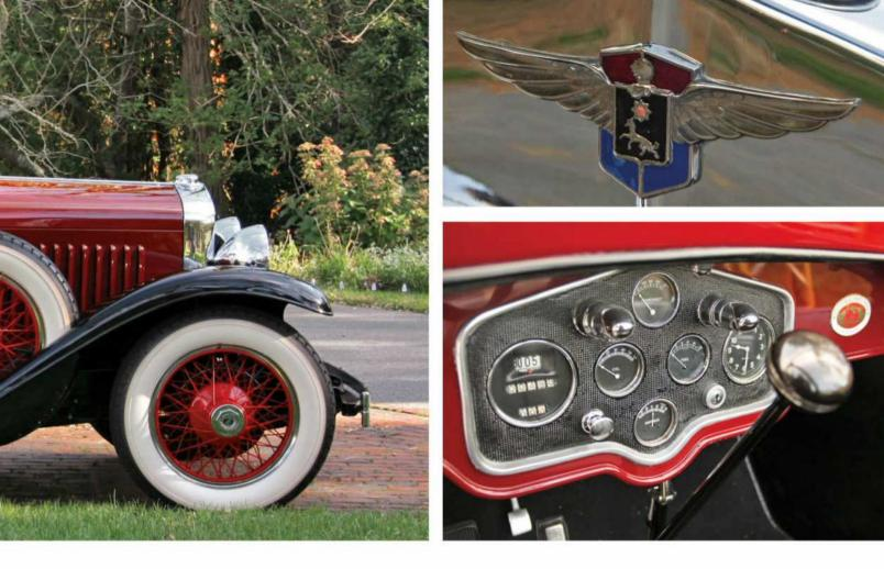
As the priciest four-passenger open car in the La Salle line, the Sport Phaeton was lavishly equipped with a distinctive pedestal spotlamp, dual side-mount spares, and a folding rear luggage rack. The winged radiator emblem included the La Salle family crest and Hispano-Suizastyle wings. Instrumentation was comprehensive, and leather upholstery was used in both front and rear cabins.
