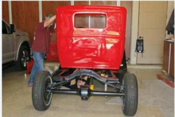
According to Kevin, the hardest part of the restoration was bodypanel alignment. A crucial first step is the installation of the cab. Here, a friend (standing) provides gentle persuasion while Kevin (below) aligns the cab to the frame, checking clearances.
