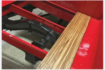
One of the final tasks required to complete the Model A pickup's restoration was the installation of new wood for the bed floor. When new, Ford painted the wood, however, Kevin—as many restorers typically do—varnished the material instead.
