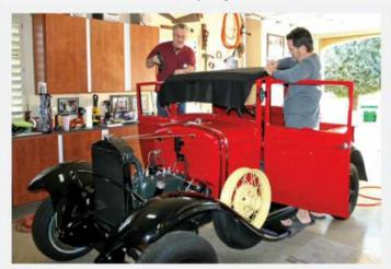
Although the redesigned closed-cab pickup utilized more steel than ever, the central section of the roof remained comprised of fabric over wood framing until August 1931. Before the rest of the interior was installed, a new vinyl roof insert was carefully put on.
