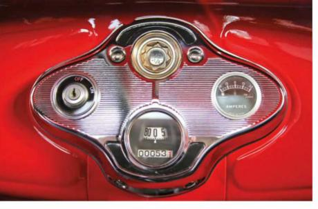
Ford updated the appearance of the Model A's basic instrument panel for 1931, which was now chrome plated and featured a ribbed motif. New varnished wood complements the pickup's bed, the one visual deviation from factory-stock configuration. The gloss black rectangular plate is centered over the differential.
