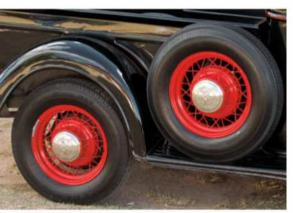
The 1935 restyle included moving the pickup's spare tire from the front fender to the bed side.
