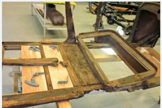
The roadster's original sill-plate assembly, which had been bolted to the frame, was deemed unusable. Note the rot present (foreground, center) just behind the seat riser. Two of the turtle-deck trunk floorboards have already been replicated and test fitted.
