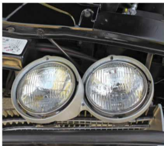
Headlamps rotate down from under the hood via vacuum when activated. Buick's 430-cu.in. engine was introduced two years prior, and the 10.25:1 compression big-block V-8 maintained a factory rating of 360 hp and 475 lb-ft of torque through 1969.
