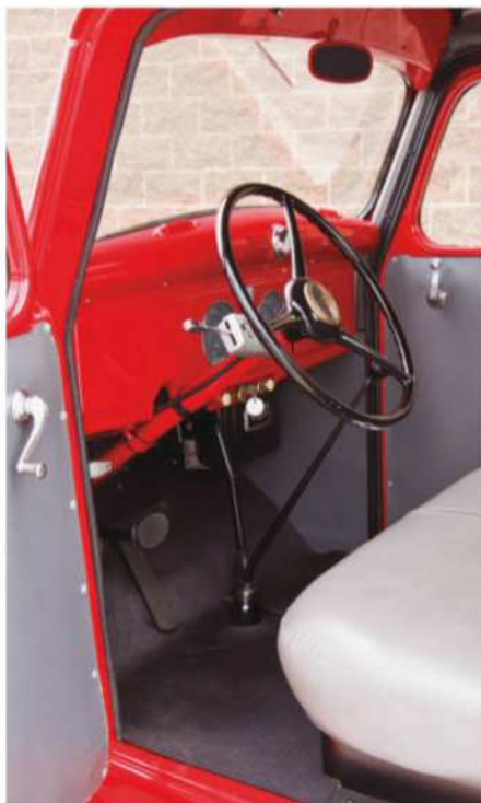
Creature comforts were minimal, but if the driver or passenger needed more fresh air, the windshield could be cranked open using the folding handle mounted top center on the dashboard.
