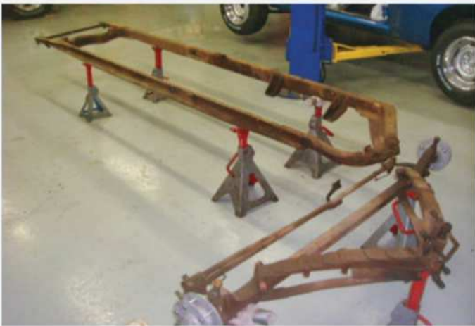
Stripped of its running gear, the Overland Model 91's very simple frame can be seen. Note the unique front axle and leaf-sprung suspension subassembly. Though a solid axle was used, the design is reminiscent of a primitive independent arrangement.
