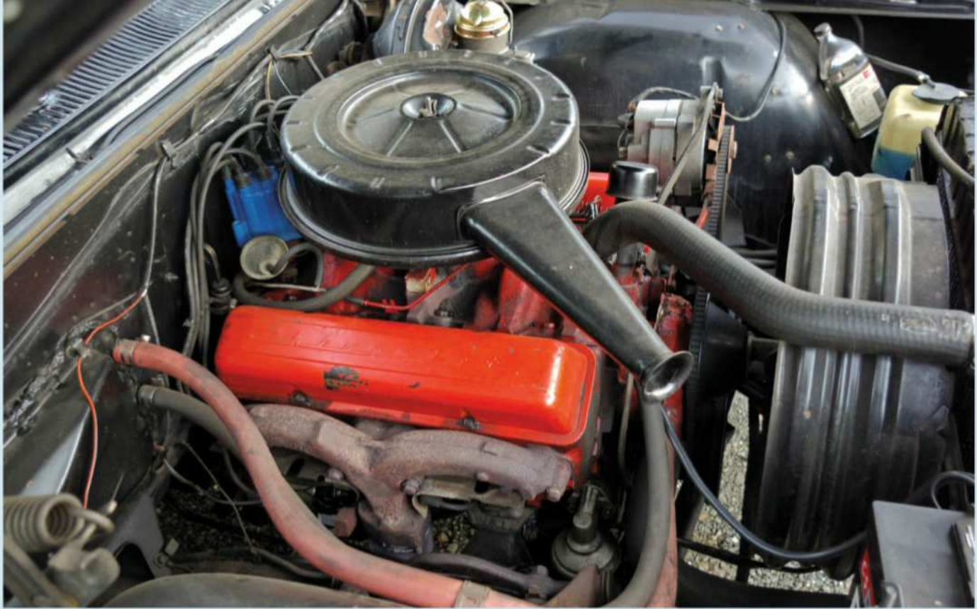
The 195-hp 283-cu.in. two-barrel V-8 hasn't required rebuilding, but was treated to new valve seals and periodic tune-ups over the years.
