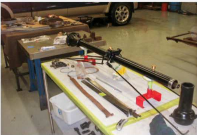
To maximize restoration efficiency, the project was always in constant motion. For example, while the frame was being media blasted and the engine was being rebuilt, the Overland's torque-tube assembly was carefully refurbished on custom stands.
