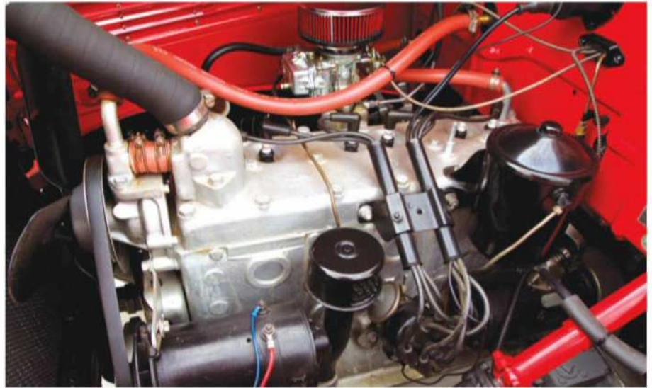
The 218-cu.in. L-head six was the standard engine in Dodge light haulers for 1938. A chrome rear bumper was optional and would've added $8.50 to the truck's $600 base price.
