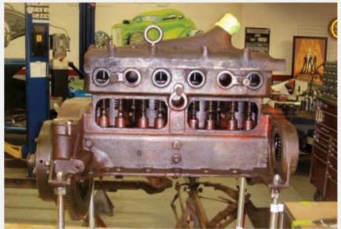
After removal of the Overland's 27-hp, 154-cu.in. four-cylinder engine, it was partially disassembled, exposing the crankshaft and valve assemblies for a quick inspection. It was then mounted in a custom-made crate and shipped out for a complete rebuild.
