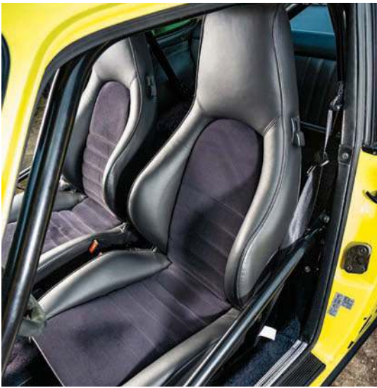
Above: Interior features retrimmed tombstone seats with lightweight RS-style door cards and door pulls. Momo steering wheel was the natural choice...
