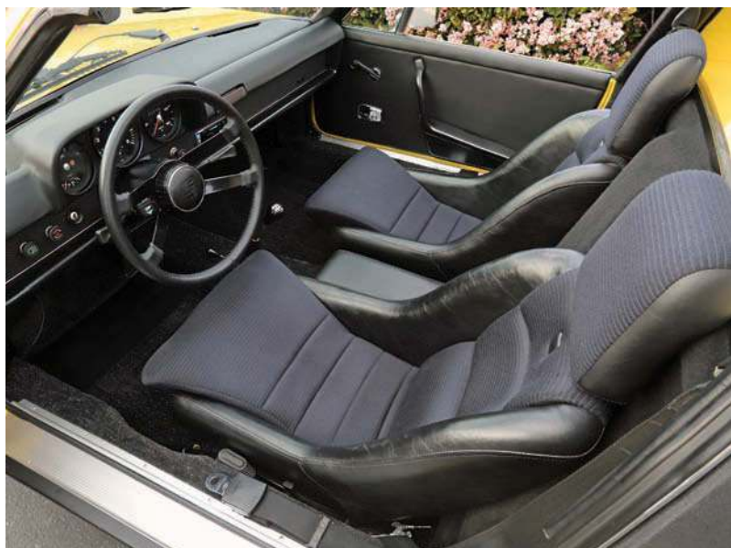
Above: Scheel seats are the perfect addition to the interior, offering far better support than the original fitment
