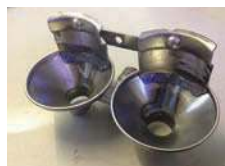
Twin Brake Reservoir bracket Ideal for twin master cylinder conversion on 356 or early 912 and 911. Designed to hold standard 356C reservoir Price £250 + VAT
