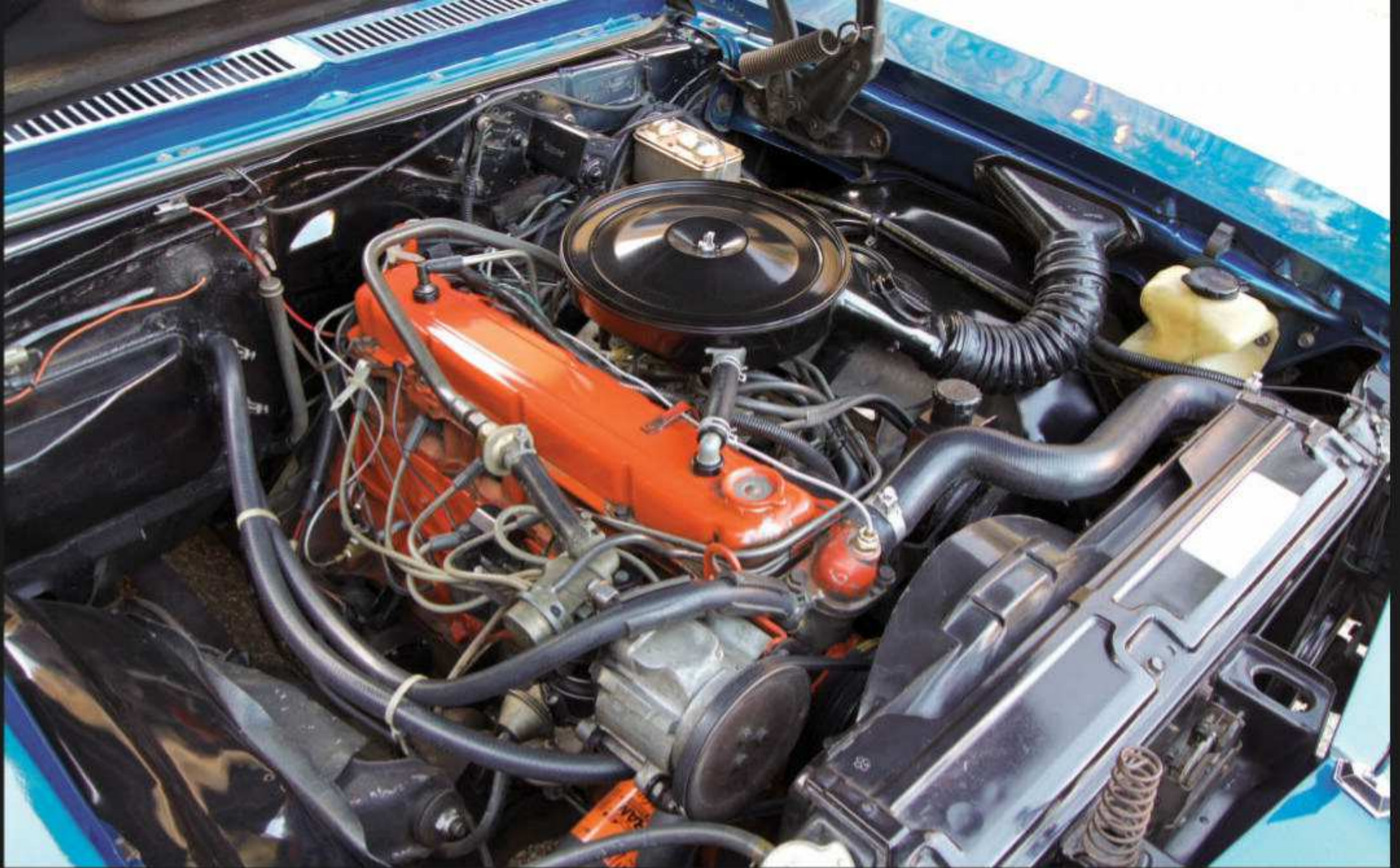
According to its owner, with more than 115,000 miles and 42 years of service on the Chevrolet 250-cu.in. six-cylinder engine, its carburetor hasn't even required a rebuild yet.
