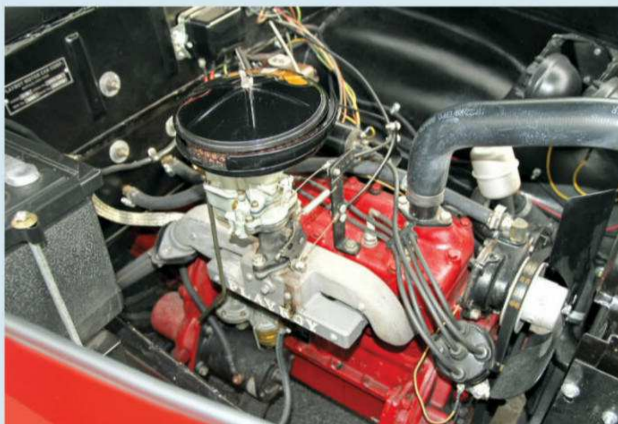
The 48-hp Hercules engine sits lower in this production car, increasing hood clearance and stability. A correct Carter one-barrel carburetor feeds fuel to the four-cylinder.
