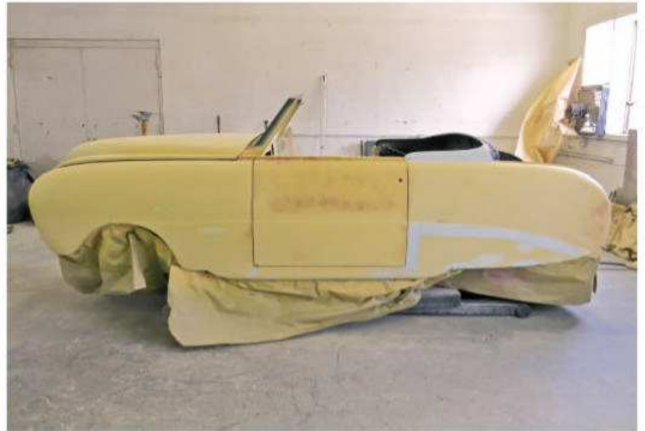
Several steps are underway in this image. A guide coat is sprayed over the high-build primer to identify high and low spots in the bodywork while block sanding.
