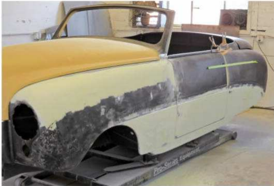
The hood has already been protected in primer and massaged to better fit the body, while corrective bodywork has begun on the flanks. Note that the door, which has been realigned, is clamped shut to help maintain the proper contour of body lines.
