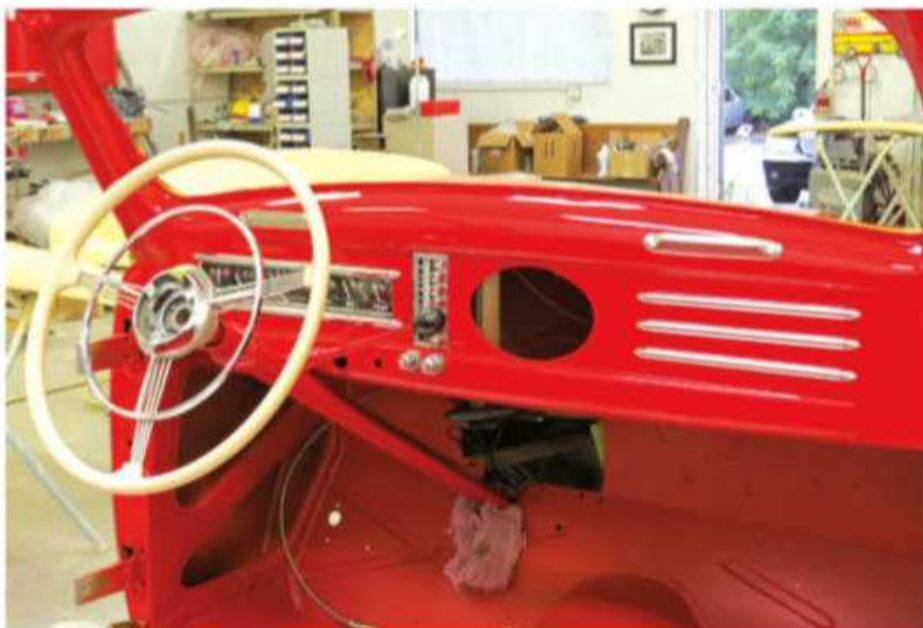
Once the paint process had been completed, the Playboy's final reassembly moved forward, beginning with the steering system, shift linkage, gauge cluster, and optional radio. Decorative dash trim was fabricated and plated prior.
