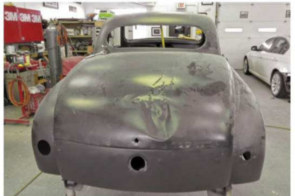
A closer look at the rear of #102 reveals multiple cutouts performed by factory employees in 1948; the dents in the decklid came later. Note that the convertible top has been raised, which is in the process of being adjusted for fit and function.
