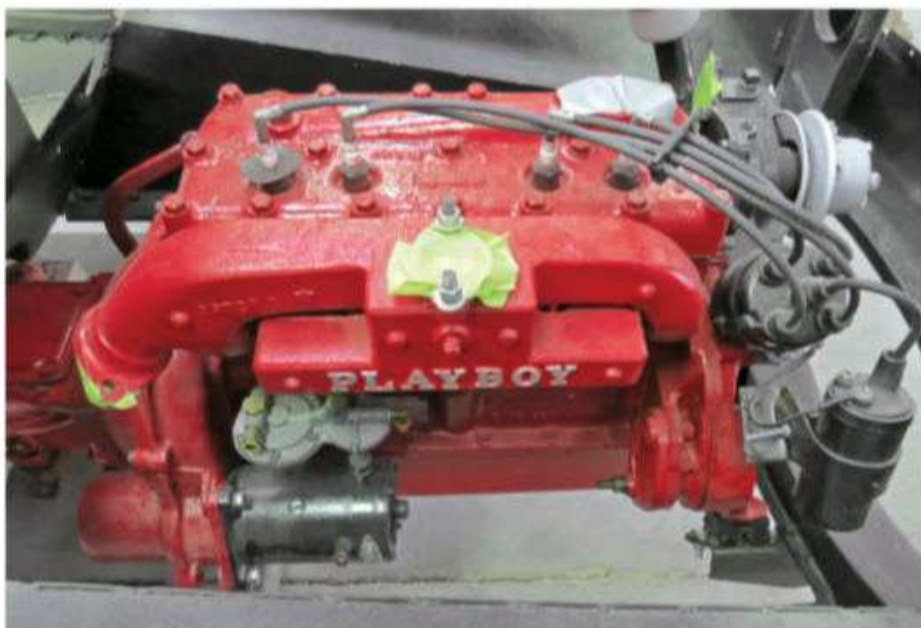
The Playboy’s engine and transmission were removed and rebuilt during the project’s early phase. Featuring a factory custom intake/exhaust manifold, the four-cylinder engine is a 48-hp unit purchased from Hercules. A correct carburetor was added later.
