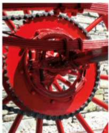
Dual chain drive (right, below) features differential action via clutches on the drive sprockets, which disengage when the wheel turns them faster than the sprockets are driven.
