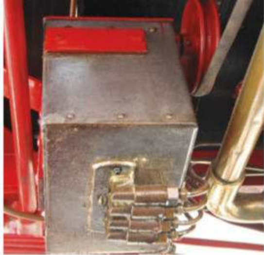
The Model P Surrey rides on an 87-inch wheelbase; its tall wooden wheels are 36 inches in diameter, 1 3/8-inch wide. The two-cylinder Reeves engine (left) is mounted below the seat. All mechanical pieces are lubricated from a single oil tank (above). A simple, brass updraft carburetor (above right) feeds the engine. "Motorgo" brass plate (right) conceals the ignition switch.
