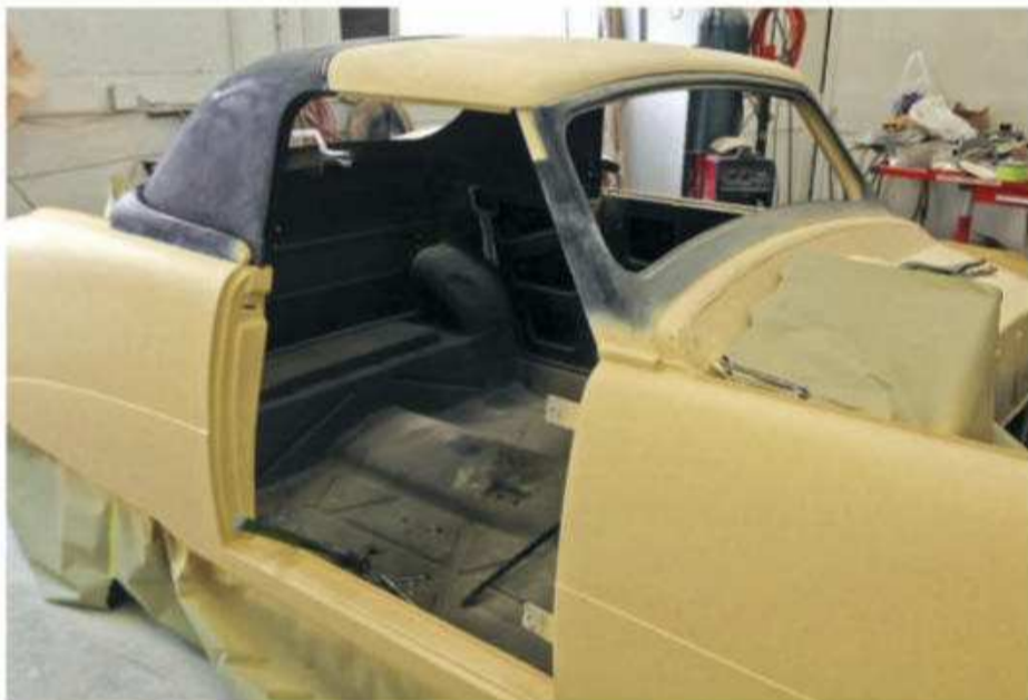
Though the two-piece folding hardtop had been tested prior, it was checked once more to help verify smooth operation and fit against the main structure. Each section then received the same filler/sanding/primer treatment as the body sides.
