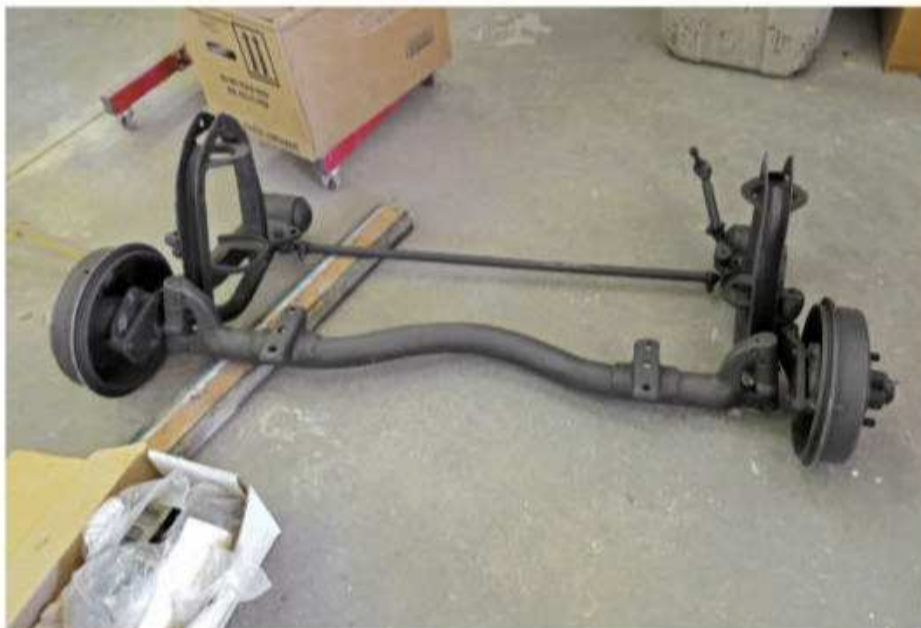
This is a portion of the Playboy’s unique front suspension system, removed from the chassis as a subassembly. Dry storage prevented rust from invading the metal, which meant most of the components only need to be cleaned and refinished.
