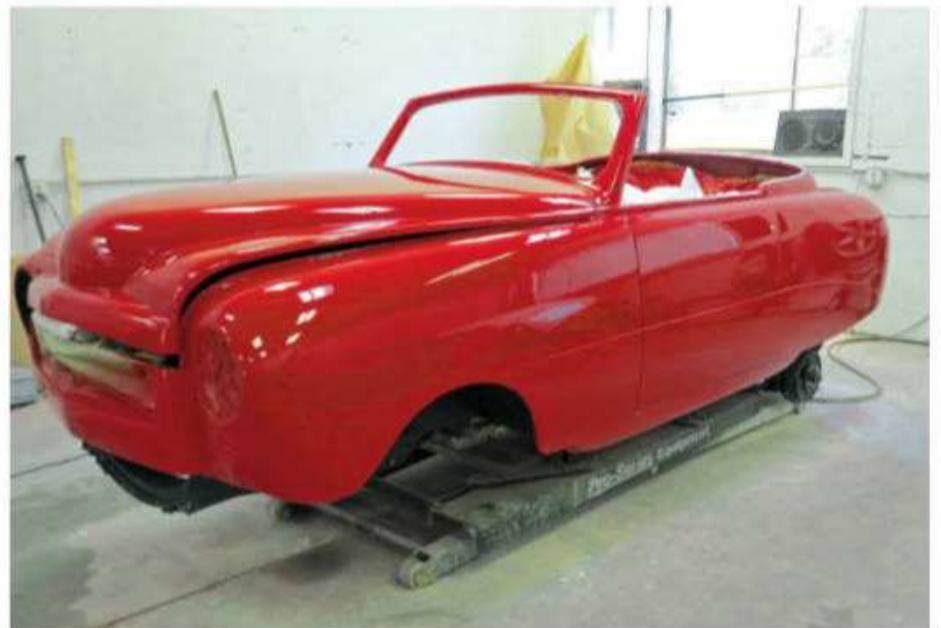
After a final coat of primer, which was then wet-sanded smooth, several layers of basecoat were applied, then topped with a few layers of clearcoat. There was friendly debate about color; however, red—matching factory literature—was selected.
