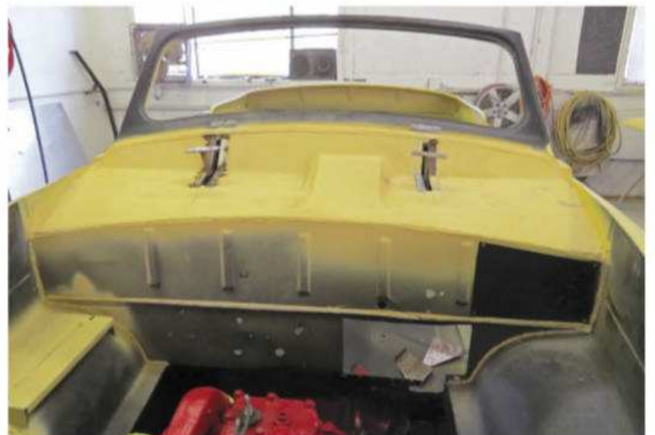
While the firewall had been hand-formed and welded in at the plant, the top of the cowl had never been fabricated. A significant step forward in the restoration was replicating what the factory had in mind, in addition to engineering hood hinges.
