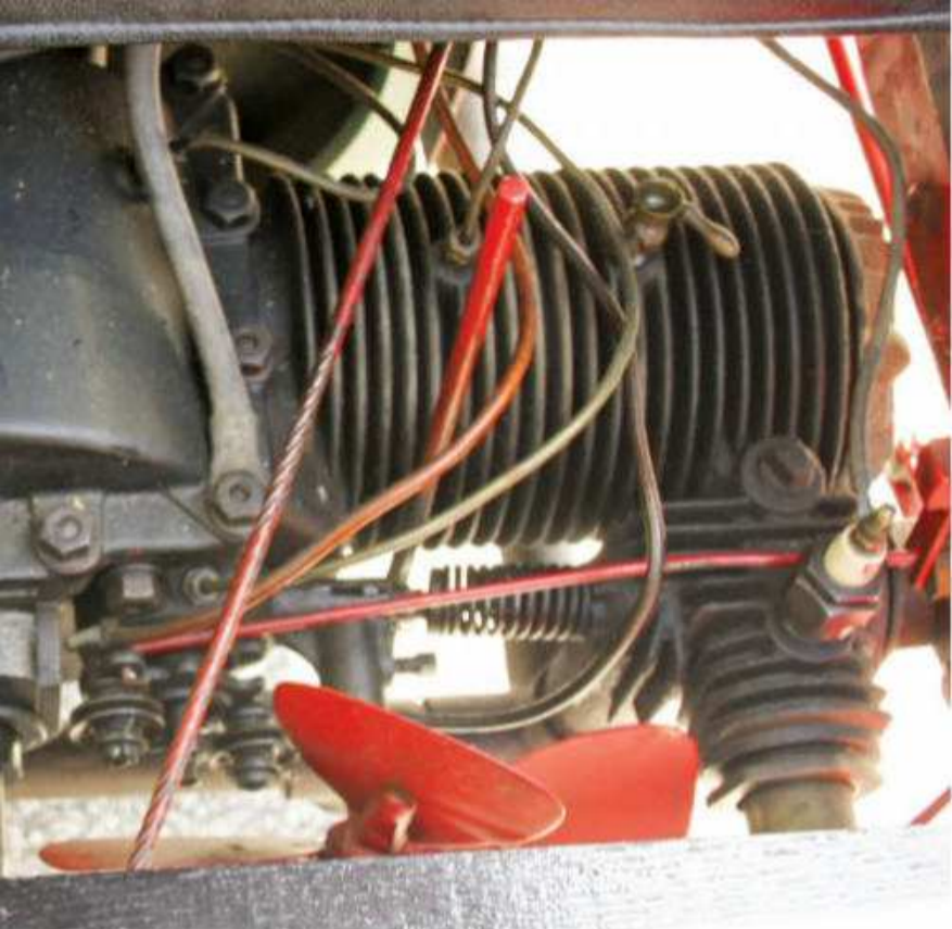
The Model P Surrey rides on an 87-inch wheelbase; its tall wooden wheels are 36 inches in diameter, 1 3/8-inch wide. The two-cylinder Reeves engine (left) is mounted below the seat. All mechanical pieces are lubricated from a single oil tank (above). A simple, brass updraft carburetor (above right) feeds the engine. "Motorgo" brass plate (right) conceals the ignition switch.
