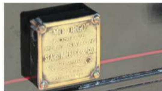
The Model P Surrey rides on an 87-inch wheelbase; its tall wooden wheels are 36 inches in diameter, 1 3/8-inch wide. The two-cylinder Reeves engine (left) is mounted below the seat. All mechanical pieces are lubricated from a single oil tank (above). A simple, brass updraft carburetor (above right) feeds the engine. "Motorgo" brass plate (right) conceals the ignition switch.
