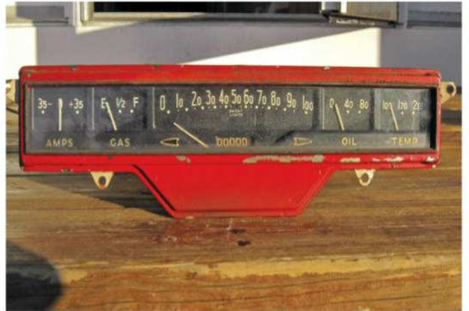
One of the first parts removed from the hardtop convertible was the gauge cluster; the only piece secured to the dash panel. Note the mileage is “00000.1” and the red paint that had been applied to the surround at the factory in late 1948.
