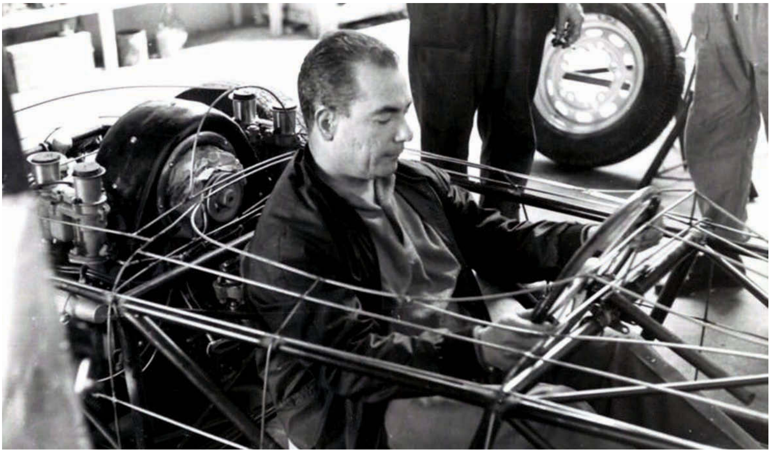
Above: Behra's personal mechanic Auguste Stocklin assisted in final assembly at Giorgio Neri's workshop. Wire frame delineated the surface of the bodywork
