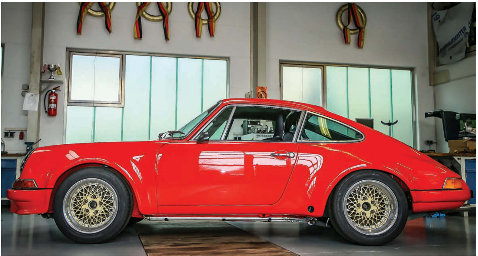
Above: Knüpfing Motorsport's ST-style 911 sits pretty on a set of BBS E50s with 205/55 and 245/45x16 Continental Conti Sport Contact 2N2s
