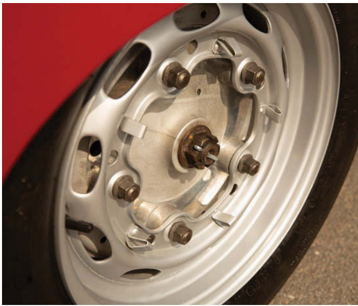
Above left: In the past, the car was equipped with Rudge knock-on wheels, which have since been replaced with the original-style rims.
