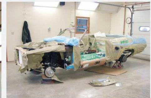
Once the metal repairs had been accomplished, the body was given multiple coats of primer, was permitted to cure, and then masked to protect the surface while the driveline and suspension were rebuilt. Note the interior has already been repainted.
