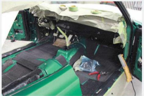
Following the paint process, reassembly of the Torino GT's interior could begin in earnest. Here, reproduction sound deadening/ insulation is in the process of being fitted. New floor carpet and reupholstered seats would follow. Note the dash is installed.
