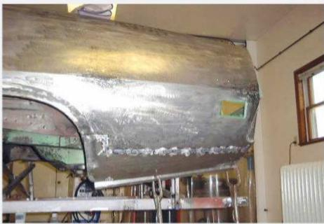
After the unit-body chassis had been repaired, metalwork shifted to the lower extremities of the car's quarter panels. New lower patch panels were fabricated to properly correct questionable repairs attempted by a prior owner.
