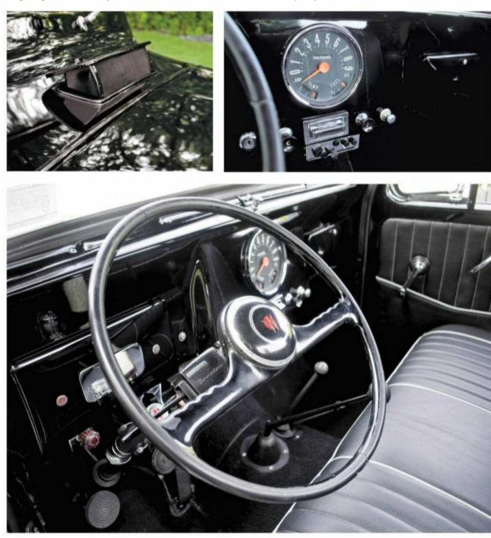
Carpeting, as well as pleated and piped upholstery, add some civility to the Willys interior. That's a radio-delete plate and plugs in front of the driver, while the speedometer was offset.
