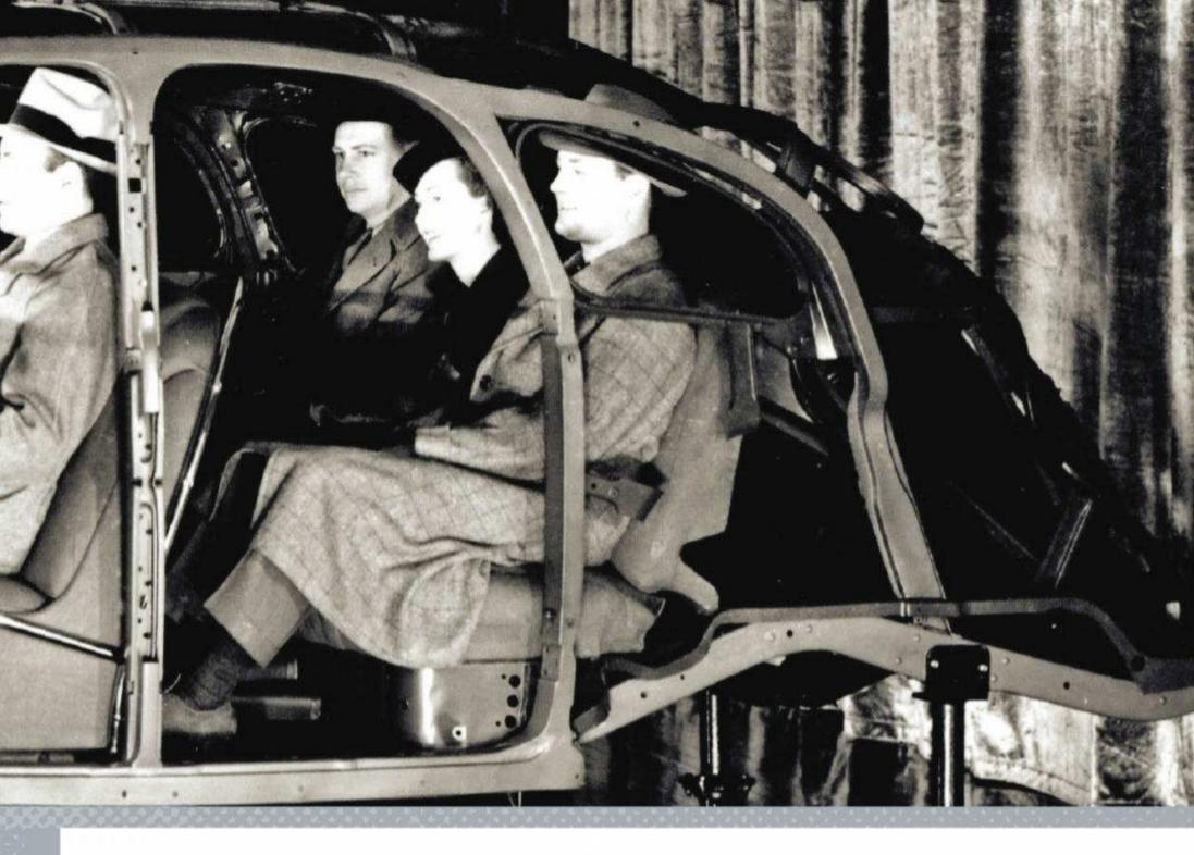
this compromised side-impact protection considerably, while adding weight. As cars became lower, another problem was revealed: the frame, being the strongest part of the car, was rapidly becoming too low to offer adequate protection in side impacts. In addition, the structural integrity of the body/ chassis combination was dependent on a handful of body bolts that held the body to the frame. They could easily shear off in a severe accident.
