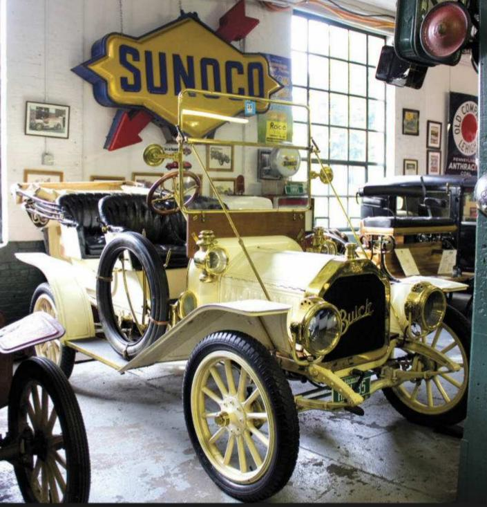
This four-cylinder, 22.5-hp 1910 Buick Model 10 was the second motorized vehicle to be used to deliver mail in all of Vermont. It's flanked by a barn-find 1908 Maxwell Model LC Tourabout and a replica 1886 Benz Patent Motorwagen, built in 1986. At right is a cutaway 1930 Ford Model A engine/transmission dealership display.
