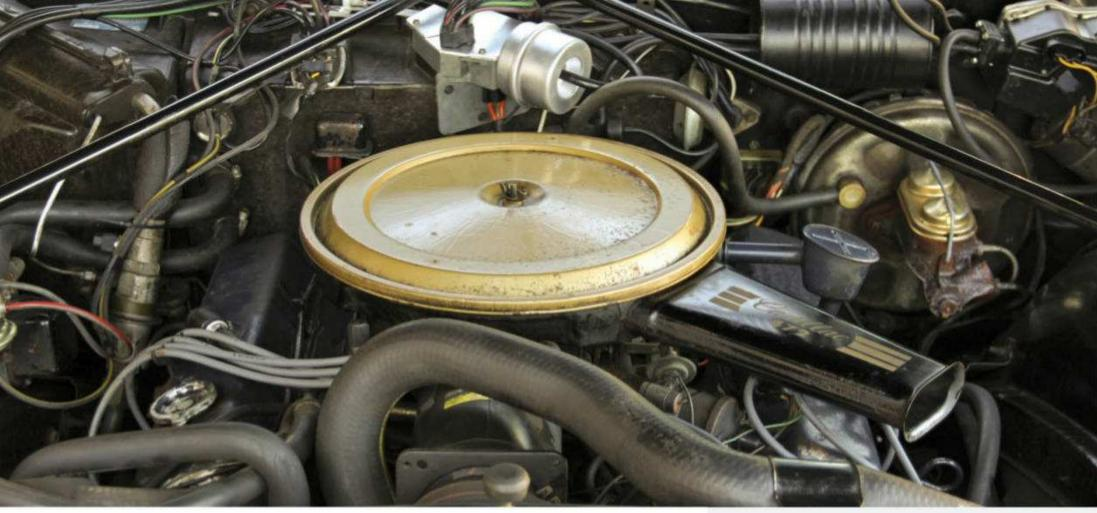
This 472-cu.in. V-8 was new for 1968, and has never been rebuilt. It provides effortless torque 50 years on, albeit with a deep thirst.
