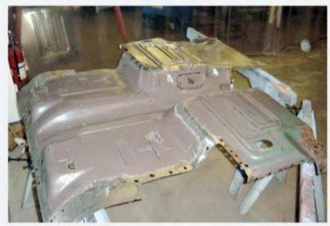
Rust had also invaded the original 21-gauge floorpan. Rather than salvage it, the unit was removed and used as a template to help expedite the fabrication of a new piece using stronger 19-gauge steel, rather than a thin (23-gauge) reproduction floorpan.
