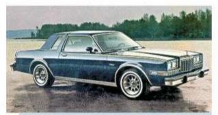
THE DODGE DIPLOMAT HAS BEEN restyled and is available as a coupe, sedan, or station wagon. Standard features include power steering, power brakes, white sidewall radial-ply tires, and the reliable six-cylinder 225-cu.in. engine; optional is the 318-cu.in. V-8 for more performance. Cabin comforts include cloth/vinyl bench seating, interior hood release, and resettable trip odometer. Look for the two-door Diplomat Special Sport to come out mid-year. The new Diplomats start as low as \$5,995.
