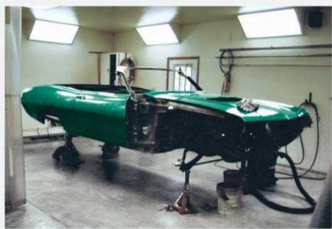
The Torino's amateur restoration did little to rectify the rust discovered within the chassis as disassembly continued. Here, most of the suspension has been detached, while the bulk of the exterior trim and incorrect Laser Stripe have been removed.
