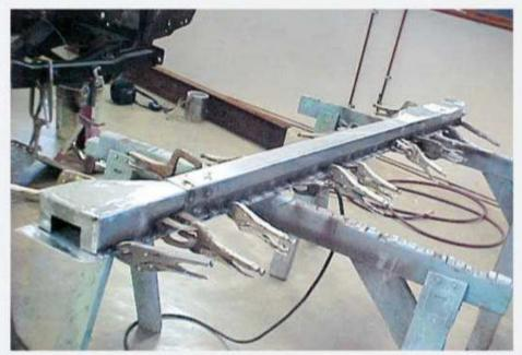
Engineers designed 7-foot-long subframe rails, with integrated torque boxes, into the unit-body chassis. Rather than repair the originals with patch panels, new all-inclusive subframes were fabricated using thicker-than-stock 12-gauge steel.
