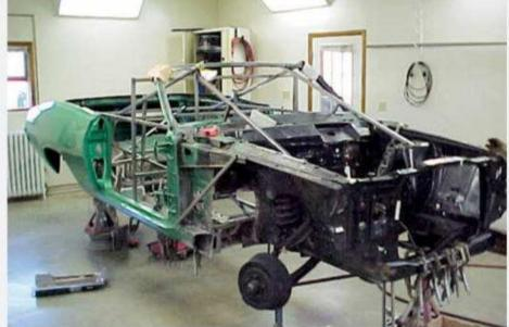
To keep the Torino's body from twisting while each subframe rail was replaced, the convertible was given an extensive web of bracing, made from square tubing, before the first cuts in the chassis were made. The new rails were TIG welded into place.
