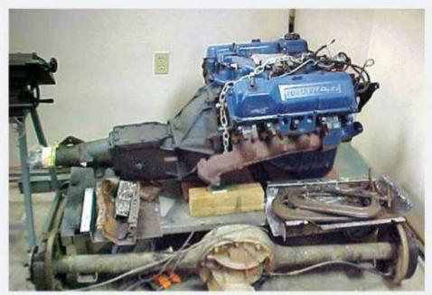
After it was determined that the convertible required a complete restoration, further disassembly started with the removal of the entire driveline. This included the 285-hp, 351-cu.in. Cleveland engine, four-speed manual transmission, and 9-inch differential.
