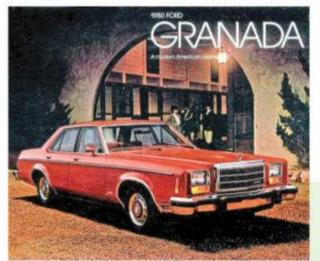
**FORD'S GRANADA RETURNS WITH SIX** editions to choose from, and a wide range of options that include new body and vinyl roof colors. The Granada is powered by a standard 250-cu.in. straight-six or an optional 302-cu.in. V-8 with a floor-mounted fourspeed fully synchronized overdrive transmission, and is available with Ghia or ESS trim. A functional, comfortable, and economical car, the base Granada costs \$4,987.
