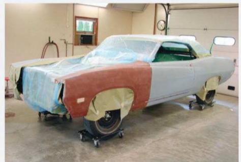
With the new top installed and the car returned to the shop, the masking was removed — exposing the body — at which point the new top, interior, and engine bay were masked, as well as the chassis, in preparation for final adjustments and paint.
