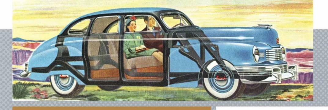
Nash Motors used a great deal of print advertising in order to fully explain the advantages of its unibody construction. Note how there are steel ramparts ahead of the cowl that tie into the front framework that extends to the front bumper area.
