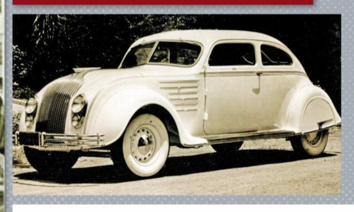
nly a handful of automotive innovations from the 1930s remain relevant today. Frontwheel drive is one, although it was a rarely seen technology in the 1930s, and steel bodies are another, and greatly advanced the sturdiness and durability of automobiles. But from the standpoint of safety and quality, the most important innovation in automobiles has to be unitized, or unit-body, construction, which became popularly known as "unibody."
