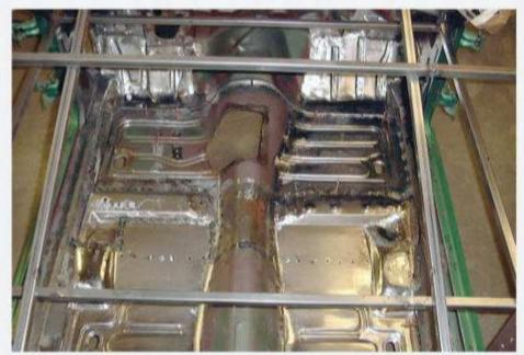
This is an aerial view of the convertible's cabin showing both the network of cross-bracing and the extensive amount of floor repairs. A keen eye will note that more TIG welding needs to be done to completely secure the new floorpans to the chassis.
