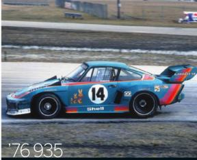
"This lightweight Group 5 with almost 600hp from the 3.0-litre Turbo engine is wrapped in slantnose bodywork, and was driven by many legends."
