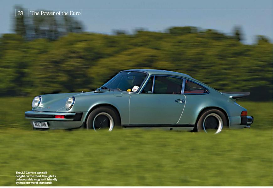
California, ghastly things such as air pumps and later catalytic converters that sucked the life out of previously happy engines. So the G Series were born with what has become known as the Impact Bumper setup. In the USA, they had spring-loaded dampers in the bumper that meant those with myopic vision and limited parking ability need not worry too much. As long as the thump of impact was around 5mph, they simply sprang back.
