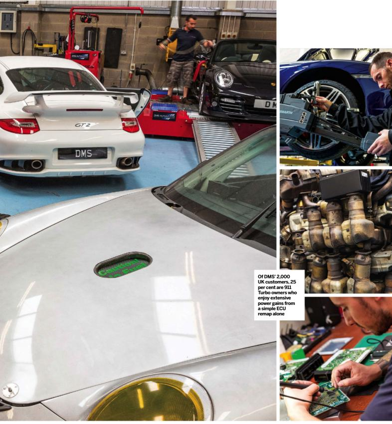
a Turbo you can get a 120bhp gain straightaway with a remap and a 200-cell catalyst. We have lots of customers who aren't necessarily petrolheads at all, but are interested in efficiency and performance enhancement. All it takes is some ECU and exhaust work, and the car can be noticeably better to drive."
