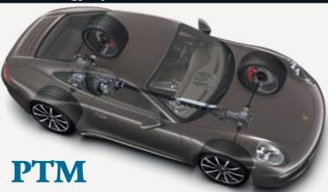
On new four-wheel-drive 911s, Porsche Traction Management (PTM) ensures grip is maintained in all conditions. Total 911 explains how the power distribution system works
