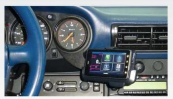
Purpose built, patented bracket and brace systems for mounting your GPS or smartphone in the classic Porsche 911
