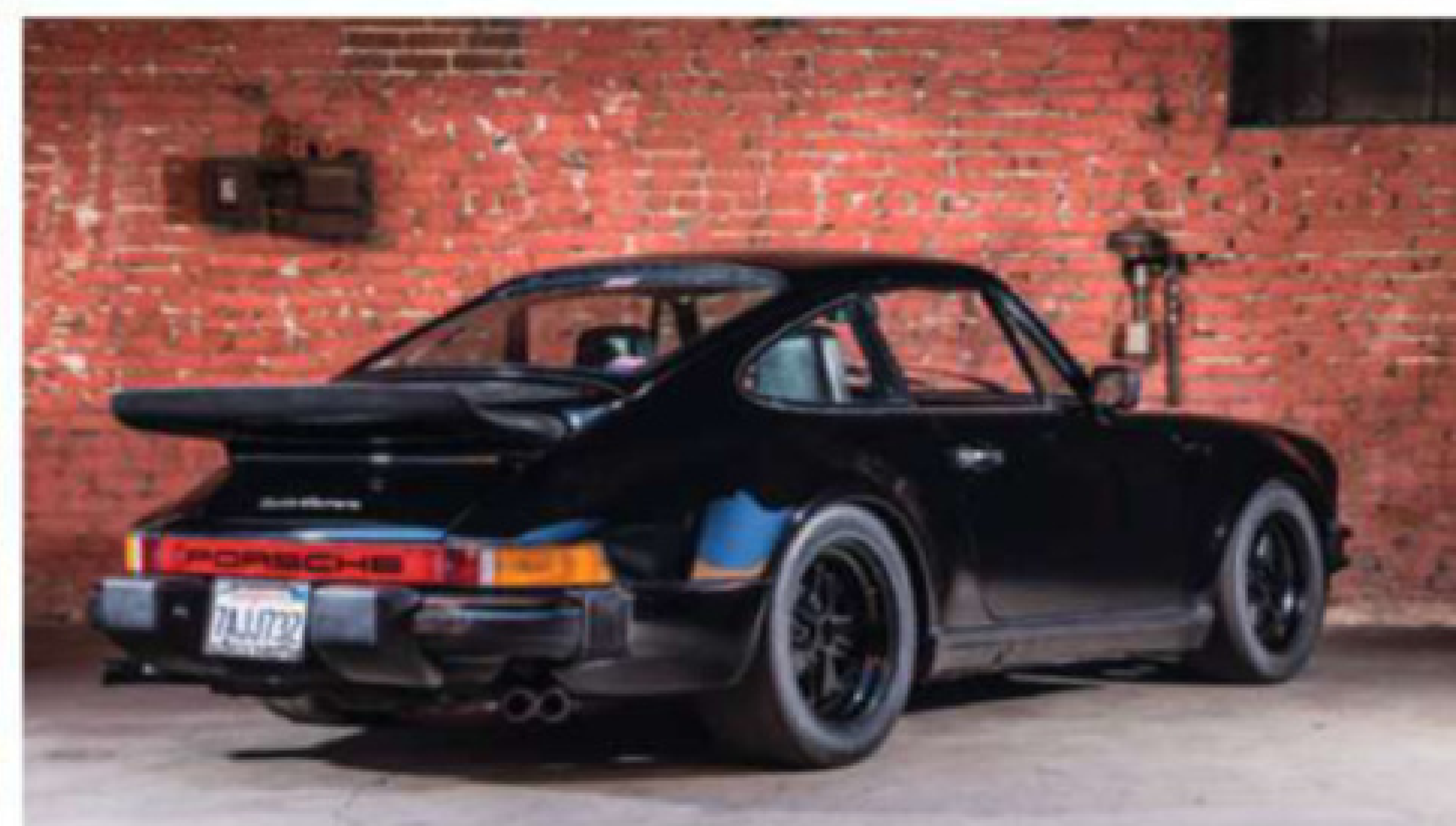
Riding on lowered springs, wider Hoosier tyres and gloss black Fuchs rims, this 1976 Turbo Carrera is mechanically standard underneath the deck lid
