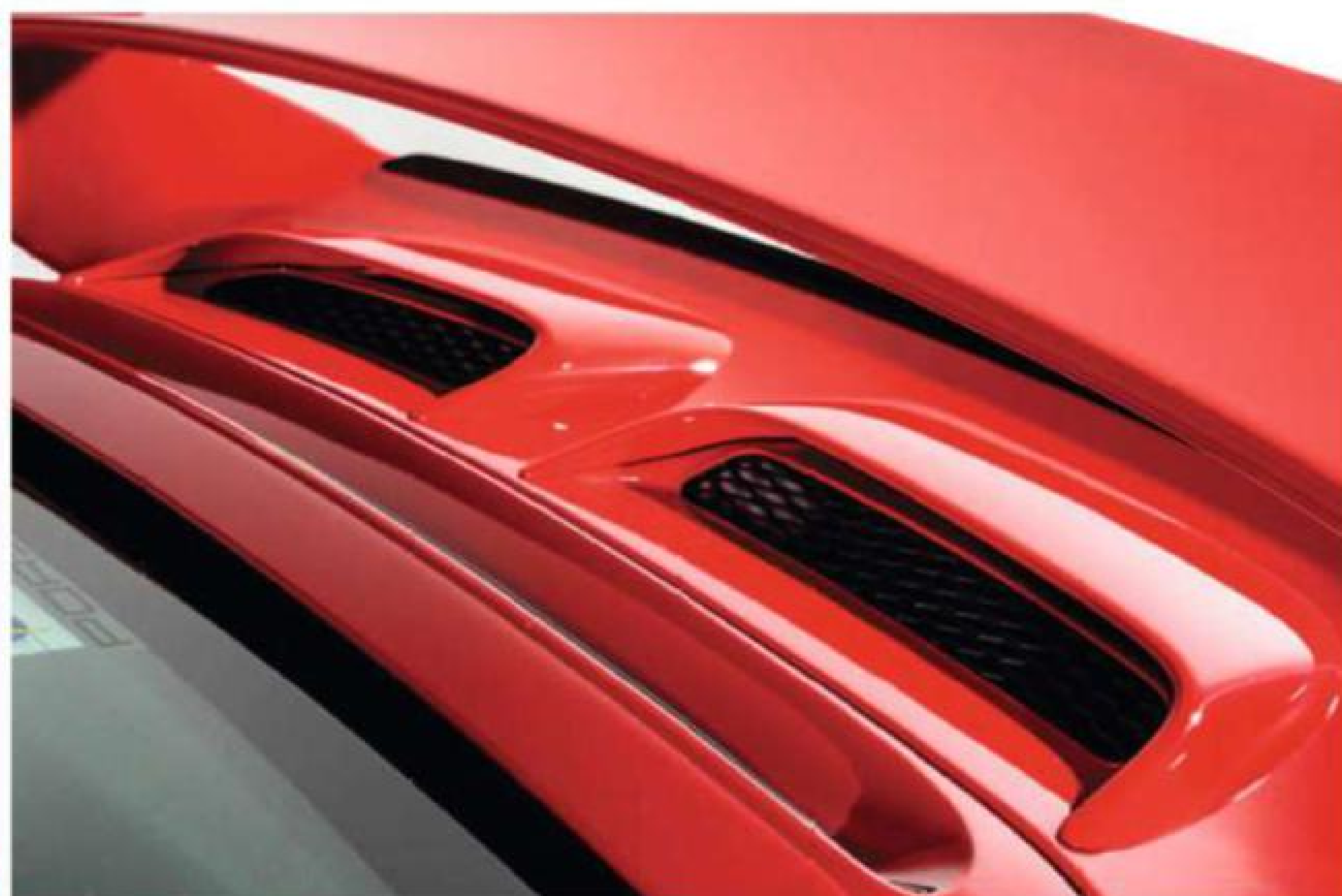
A variety of gills in the rear of the GT3 helped dissipate heat from the high-revving, dry-sump Mezger engine
